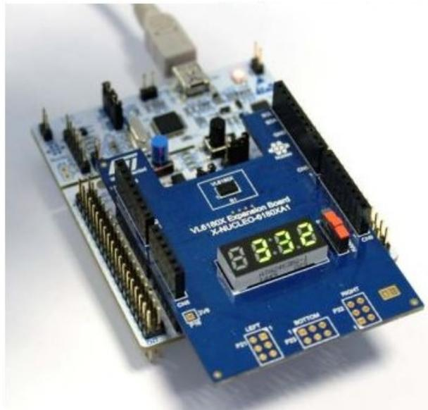
**Figure 4.9:** VL6180A1 Expansion Board plugged on a STM32 Nucleo board
