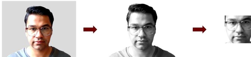
**Figure 4.9:** The process of converting input image from the webcam to a cropped version of image that contains only the face
