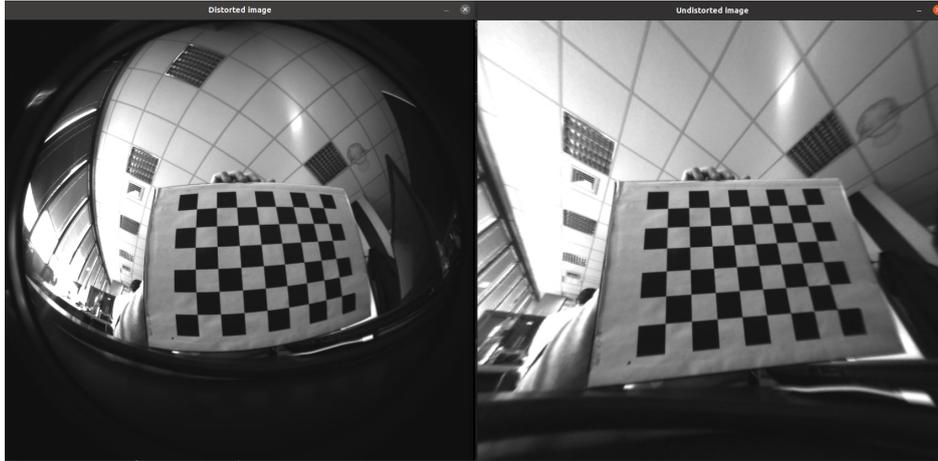
Figure 4.7: Difference between original image taken by fisheye(left) and the same image undistorted after calibration(right)
