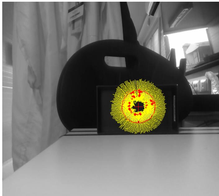
Figure 4.6: Tracking with Visp, the red points are the features extracted
