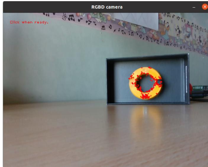
Figure 4.3: Features extracted inside ROI
