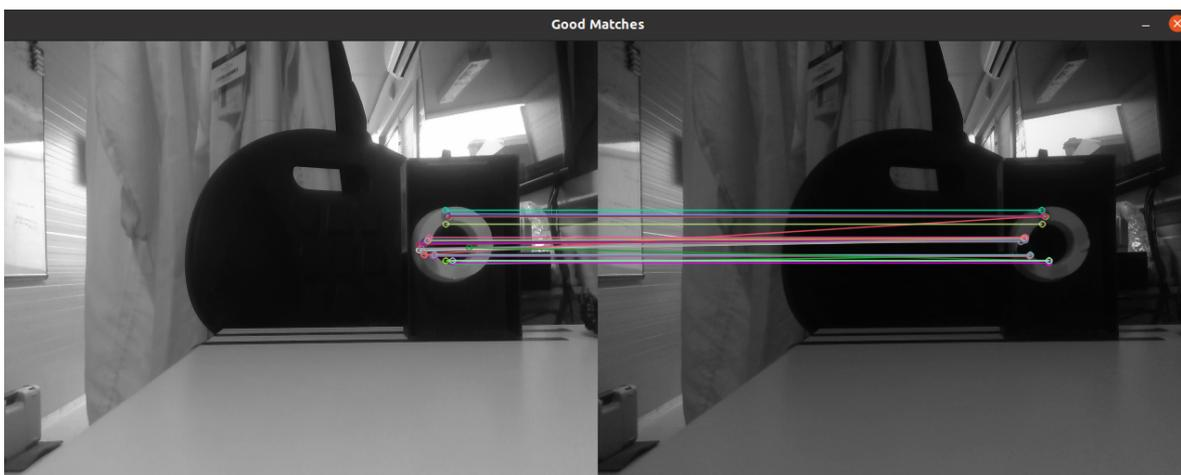
Figure 5.17: On the left is the run time image, on the right reference image (case where the run time and reference pose are equal)
