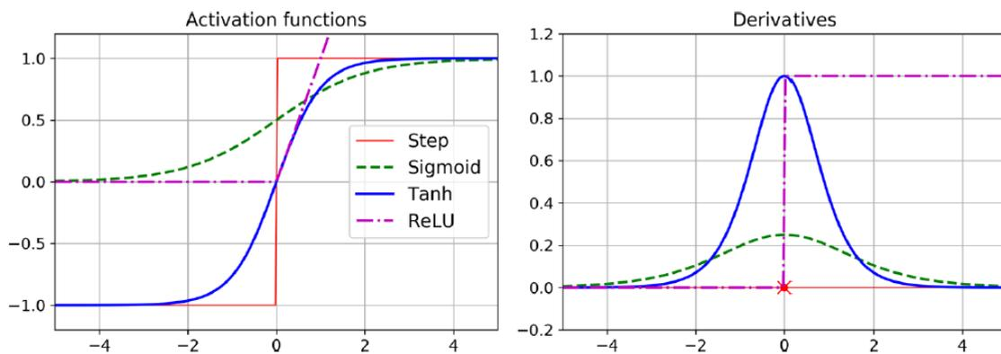
Fig.8 Different Activation functions and their Derivatives
