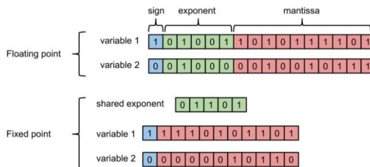
Fig. 20 Floating/Fixed-point representation
