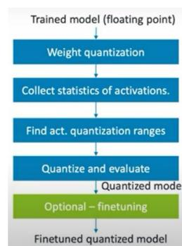
*Fig.21 Quantization Workflow*
