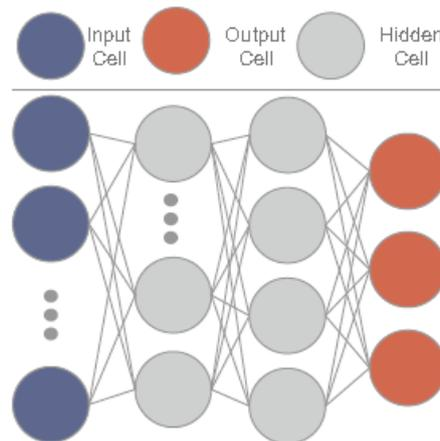
Fig.7 Architecture of a MLP with  $n$  inputs, two hidden layer and three output neurons (the bias neurons are implicit)
