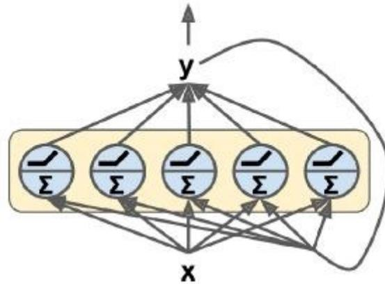
Fig.13 Layer of Recurrent neuron
