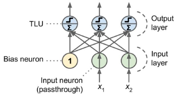
Fig.6 Architecture of Perceptron with two input neuron, one bias neuron and three output neurons
