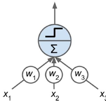
Fig.5 Threshold logic unit: an artificial neuron which computes a weighted sum of its inputs then applies a step function
