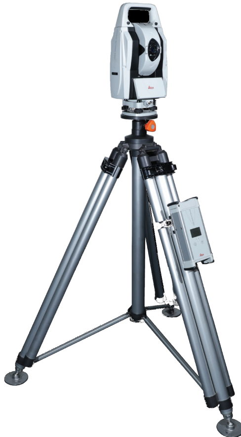
Figure 4.4: Leica AT430 mounted on a tripod with remote control unit
