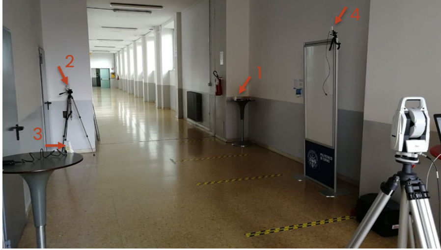
Figure 4.8: Experimental setup with four anchors
