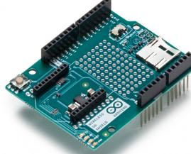
**Figure 2.9:** Wireless SD shield from [11]
