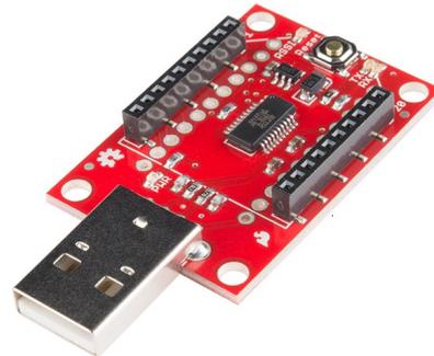
Figure 2.6: XBee Explorer from [10]
