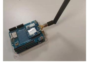
**Figure 2.10:** Transmitter/Receiver module
