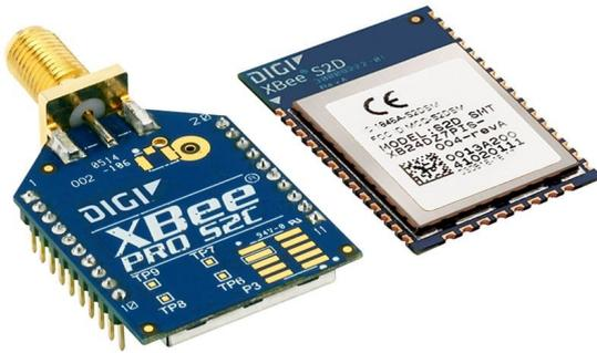
Figure 2.5: XBee module from [10]
