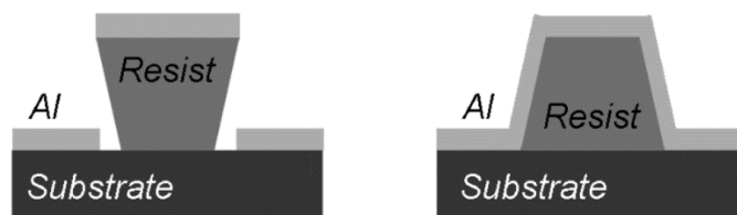
Figure 2.16: Deposited film features onto undercut (left) and standard (right) profile [73].
