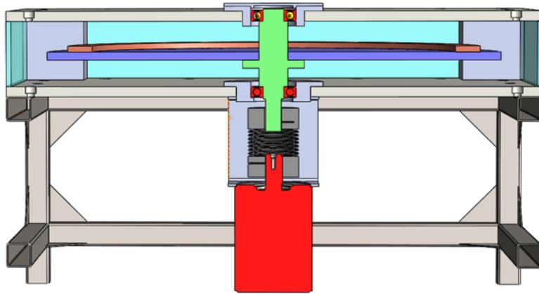
**Figure 2.3:** Test bench main frame: section view. Courtesy of Dr. A. Bonfitto, Eng. E.C. Zenerino and A. D’Oronzo.
