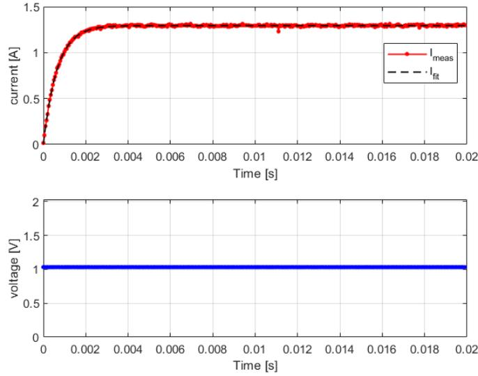
**Figure 6.23:** RL circuit identification: experimental data vs. model output
