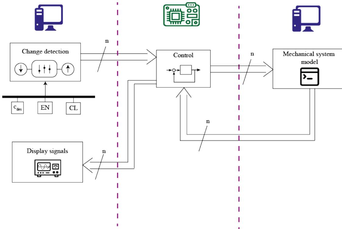
Figure 6.21: PIL test architecture
