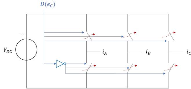
Figure 6.18: Six-step inverter, electrical scheme
