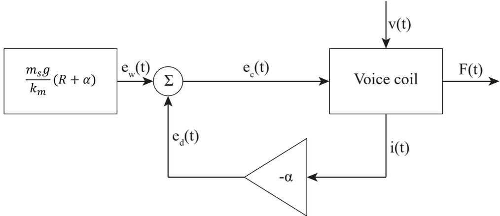
**Figure 5.2:** Voice coil control architecture: voltage feedback with constant weight compensation
