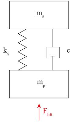
**Figure 3.4:** Two degrees of freedom levitation system: quarter car model
