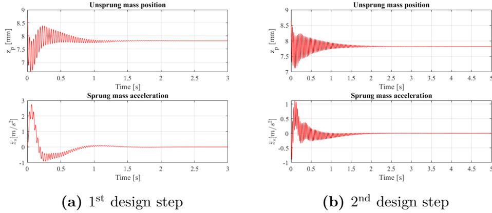
**Figure 6.12:** Output signals monitoring: unsprung mass position and sprung mass acceleration
