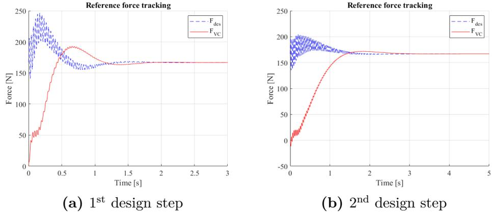
Figure 6.10: Desired force at VCA output: reference tracking
