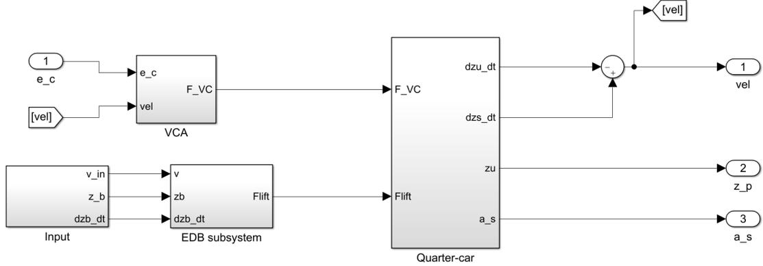
Figure 6.1: Plant and actuator, Simulink® model
