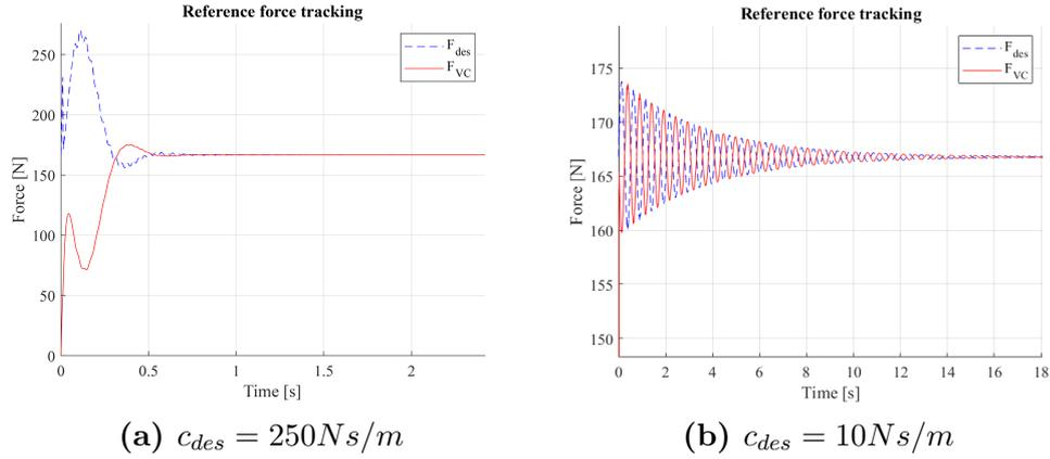
**Figure 6.6:** Desired force at VCA output: reference tracking
