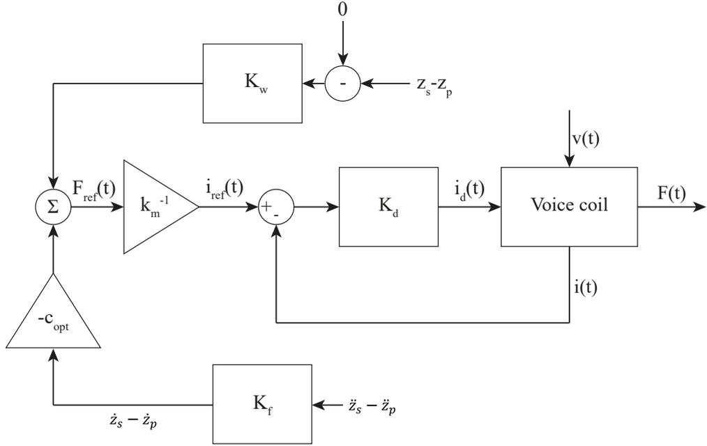
**Figure 5.4:** Voice coil control architecture: current feedback with zero regulation of  $z_s - z_p$  and  $\dot{z}_s - \dot{z}_p$  reference
