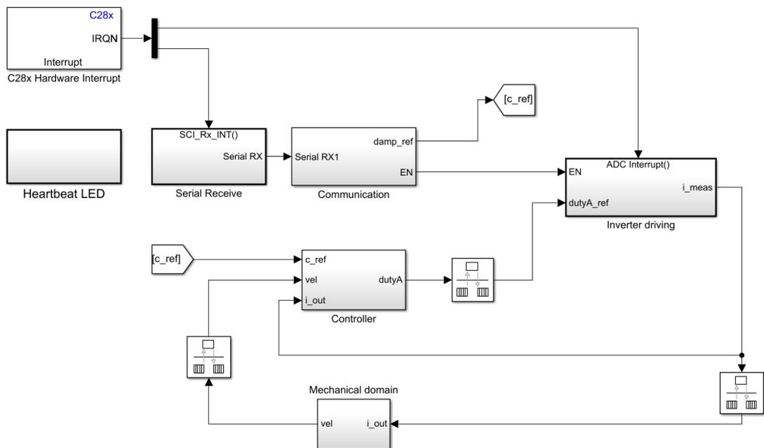
Figure 6.20: Target hardware model block diagram
