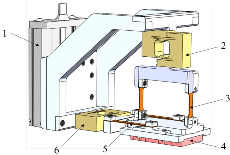
**Figure 2.4:** Measurement system for quasi-static test. Courtesy of Dr. A. Bonfitto, Eng. E.C. Zenerino and A. D’Oronzo.
