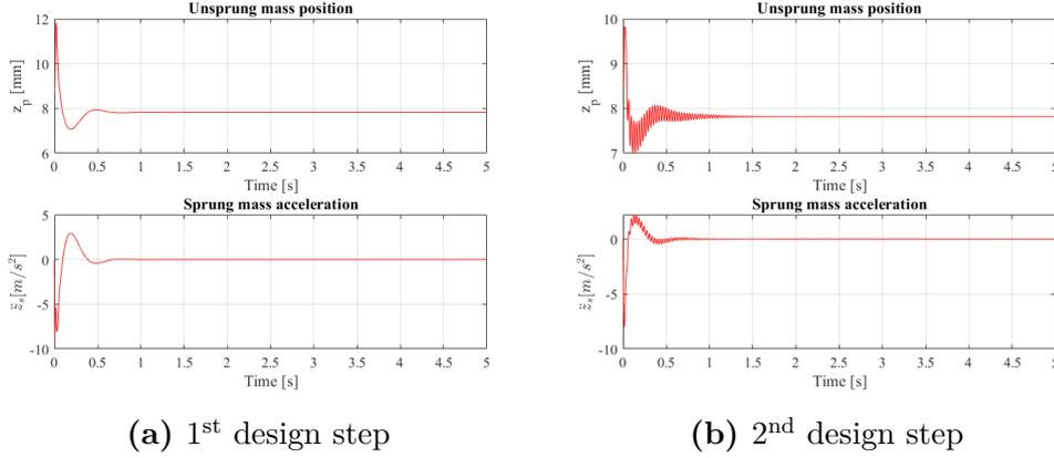
**Figure 6.17:** Output signals monitoring: unsprung mass position and sprung mass acceleration
