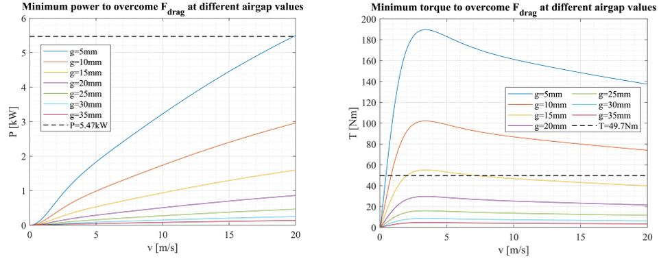
(a) Power to overcome  $F_D$  vs.  $P_{max}$  (b) Torque to overcome  $F_D$  vs.  $T_{max}$
