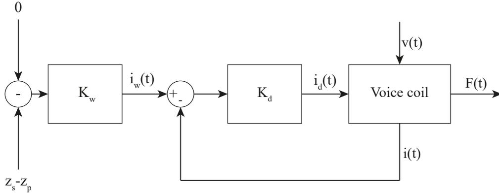
**Figure 5.3:** Voice coil control architecture: current feedback with zero regulation of  $z_s - z_p$
