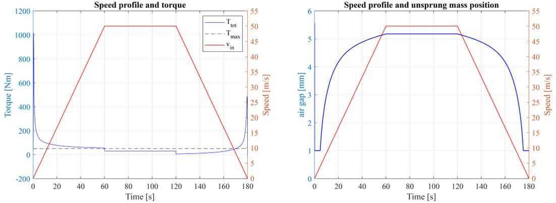
(a) Total resistant torque vs. maximum torque with respect to the input speed profile
