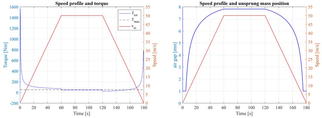
(a) Total resistant torque vs. maximum torque with respect to the input speed profile (b) Unsprung mass position with respect to the input speed profile
