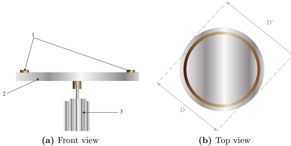
**Figure 2.1:** Frame layout: axial symmetry. 1. Track; 2. Rotating disk; 3. Motor
