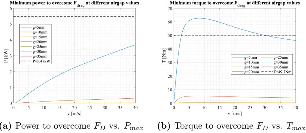
(a) Power to overcome  $F_D$  vs.  $P_{max}$  (b) Torque to overcome  $F_D$  vs.  $T_{max}$
