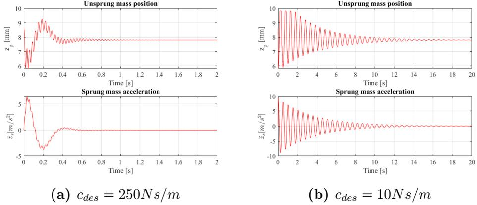
**Figure 6.8:** Output signals monitoring: unsprung mass position and sprung mass acceleration
