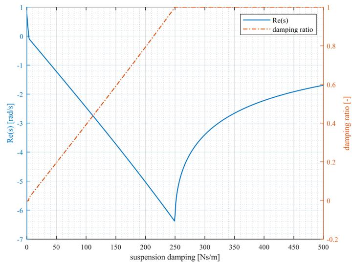
**Figure 3.19:** Stability optimisation,  $k_{us} = 0.1k_p$ . Post/Arash best payload to drag configuration
