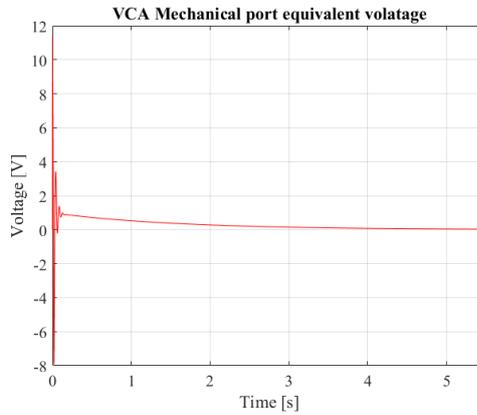
**Figure 6.27:** Equivalent voltage of the mechanical port of the voice coil actuator
