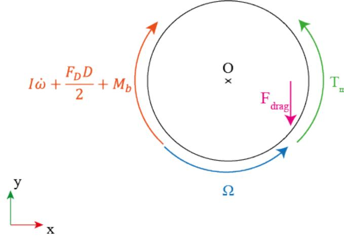
**Figure 6.2:** Disk free body diagram
