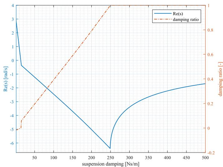
**Figure 3.18:** Stability optimisation,  $k_{us} = 0.1k_p$ . Post/Alex single bogie configuration
