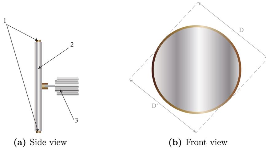
**Figure 2.2:** Frame layout: axial symmetry. 1. Track; 2. Rotating disk; 3. Motor
