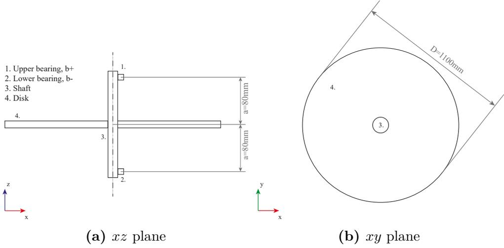
**Figure 4.1:** Test bench: shaft, bearings and disk, simplified layout
