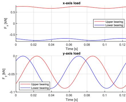
**Figure 4.2:** Time evolution of loads component over  $x$  and  $y$  axes.
