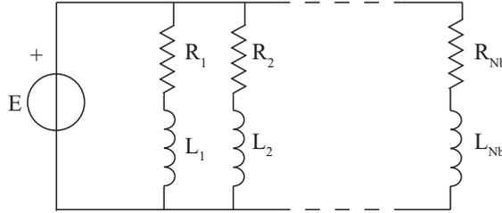
**Figure 3.3:** Lumped parameter model that describes the interaction between the PM array and the track.
