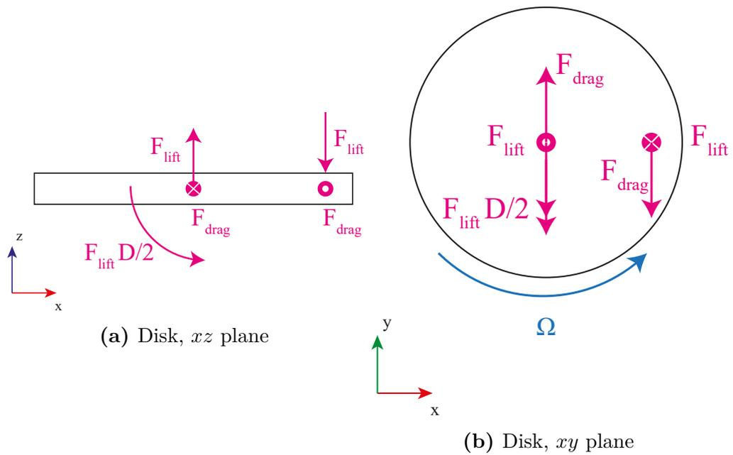
Figure B.2: Shaft free body diagrams
