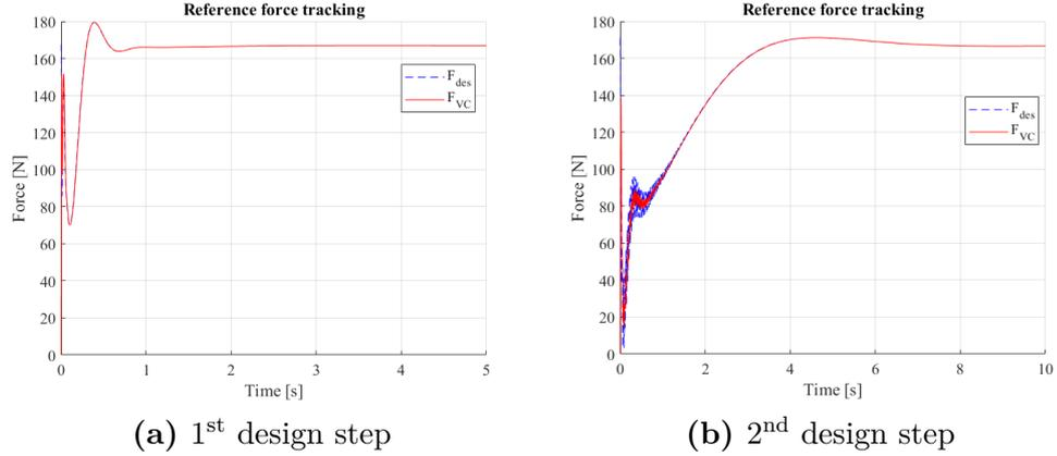
**Figure 6.15:** Desired force at VCA output: reference tracking
