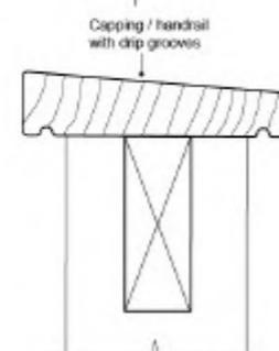
Figure 6: Typical post base to avoid water entrapment and splashing
