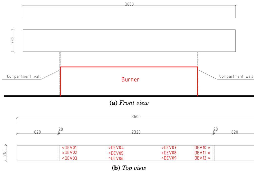
**Figure 7.19:** Benchmark structure as modeled in Thunderhead Engineering Pyrosim - Devices (DEV) for Adiabatic Surface Temperature (AST) and Heat Transfer Coefficient (HTC) - [quotes in millimeters]
