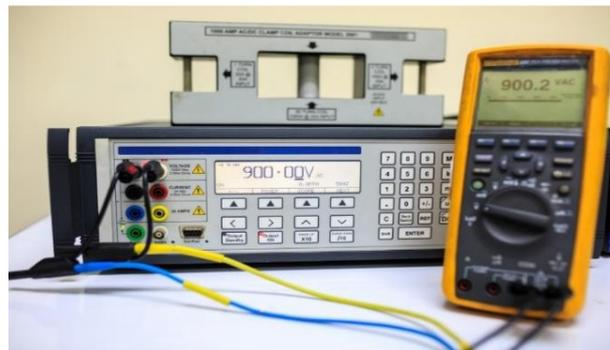
*Figure2- 7: Calibration Device.*
