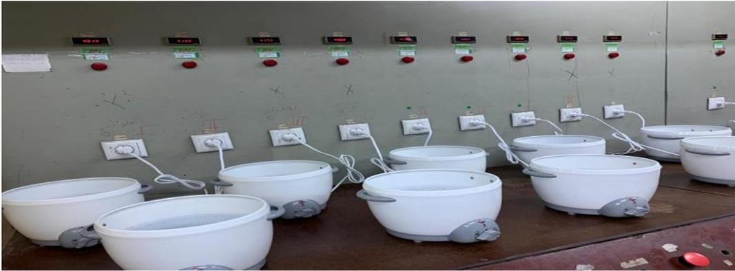
Figure 2-17: Energy Efficiency Measurement for Rice Cooker.
