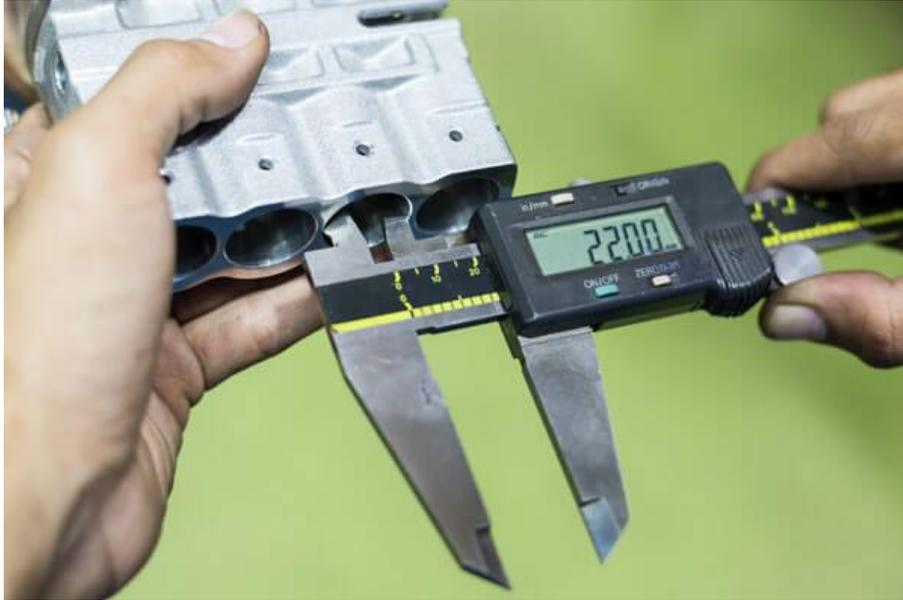
Figure 2-5: Digital Caliper.
