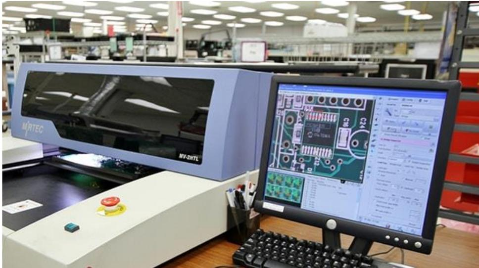
Figure 2-28: Automated Inspection.
