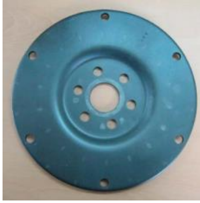
Figure 3-6 Flex plate manufactured by hot press forming technique [37]
