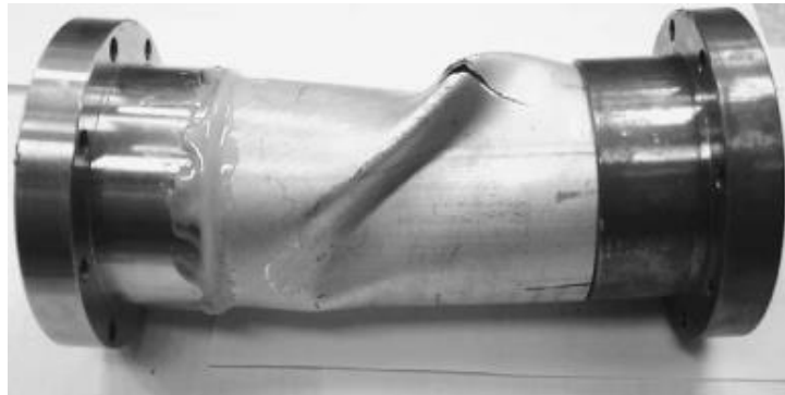
Figure 3-5 A buckled specimen after the static torque test [35]
