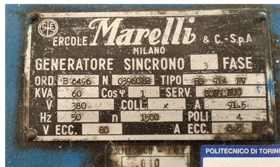
Fig. 58: Marelli Synchronous Generator nameplate.
