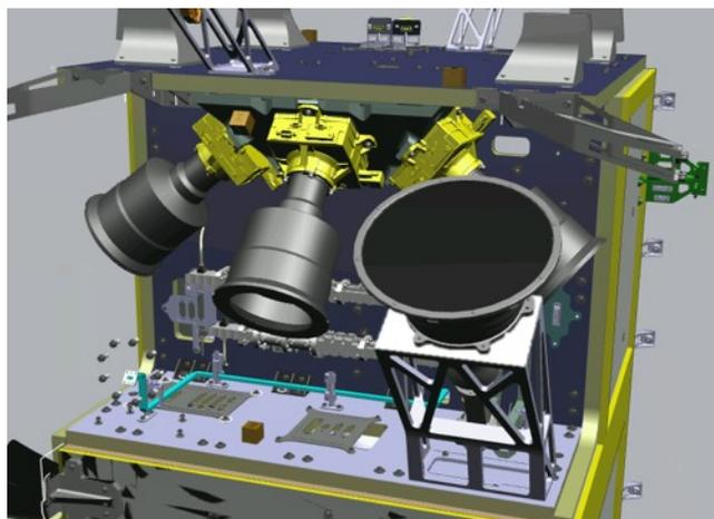
Figure 3.20: Aligning cubes on structure.
