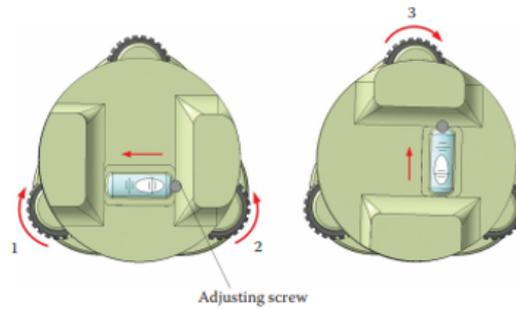
Figure 4.2: Theodolite level bubble.
