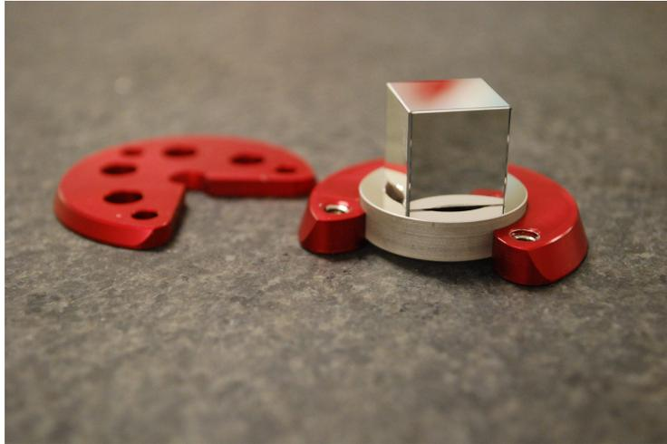
Figure 3.9: Mirror Cubes mouted on plate.
