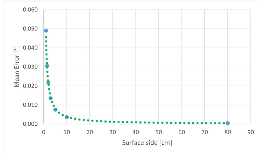
Figure 5.14: Mean Error function with side of surface,  $n = 4$ .
