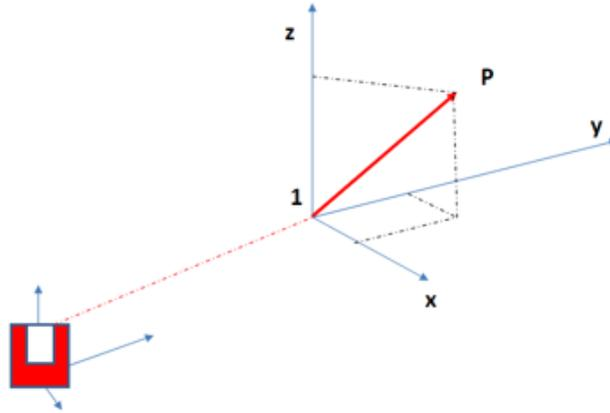
Figure 5.13: Disto Reference System Definition.
