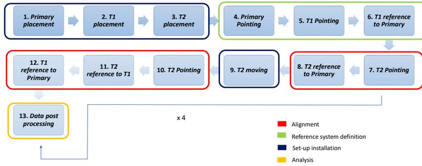
Figure 6.3: Alignment flowchart for mini-CMG.
