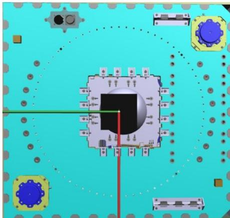
Figure 3.10: Bottom Panel representation. The circular hole pattern defines the interface with the Lightband.
