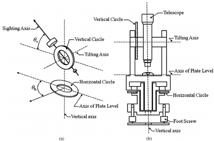
Figure 4.3: Theodolite main axes.
