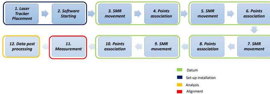
Figure 7.5: Alignment flowchart for mini-CMG 3.
