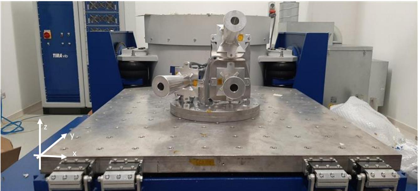
As shown in the above figure it has been established that the main measurement reference system should be located on the upper left apex of the platform. In fact, this point can be well representative of an external
