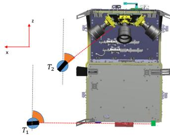
Figure 6.16: STT 1 Alignment (rotation around  $Y_{SC}$ ).
