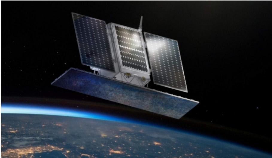
Figure 2.1: Platform and SAR antenna representation.
