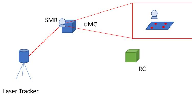
Figure 7.1: Adopted set-up for aligning units.
