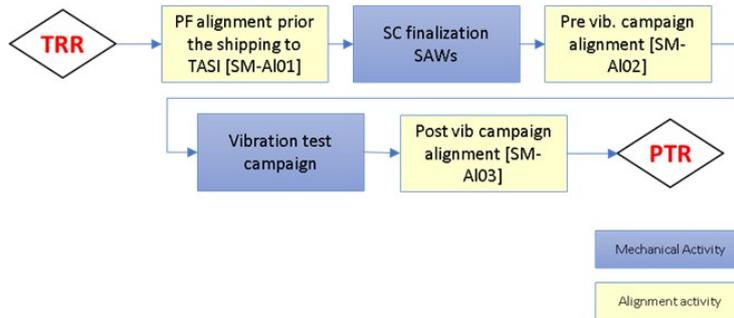
Figure 3.1: SM Alignment Flow.
