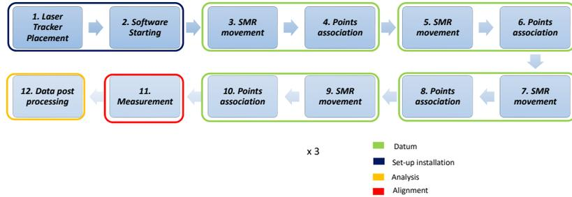
Figure 7.9: Alignment flowchart for STT.
