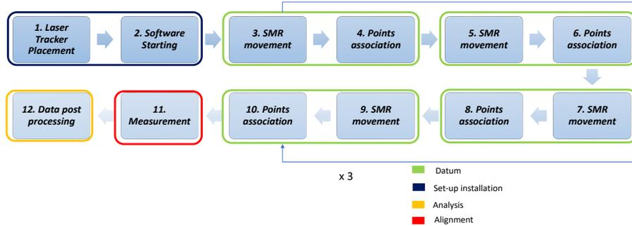
Figure 7.7: Alignment flowchart for STT.
