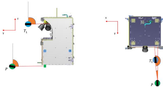
Figure 6.19: STT 3 Alignment (rotation around  $X_{SC}$  and  $Z_{SC}$ ).
