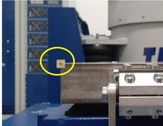
As for the reference chosen for the three units, it has been established to take the plane on each support surface. Points that are taken on these surfaces don't need stickers applications and can be checked in an easier way.
