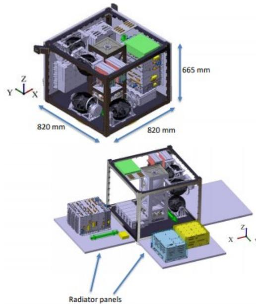
Figure 2.4: PLATiNO Thermo-structure representation.
