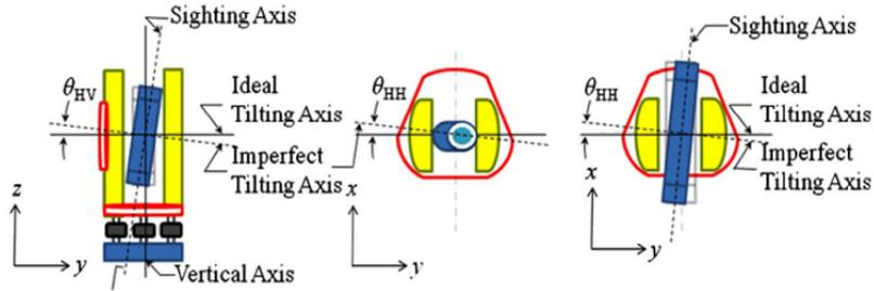
Figure 4.8: Tilting axis error.
