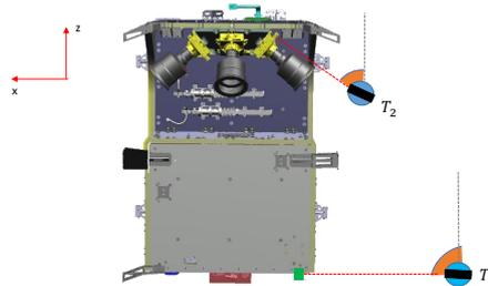
Figure 6.20: STT 3 Alignment (rotation around  $Y_{SC}$ ).
