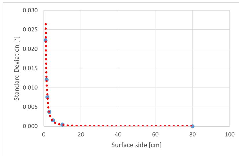
Figure 5.15: Standard Deviation function with side of surface,  $n = 4$ .
