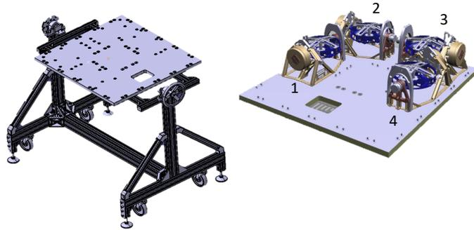
Figure 6.1: Integration Stand and intermediate panel with mini-CMG.
