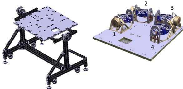
Figure 7.2: Integration Stand and intermediate panel with mini-CMG.
