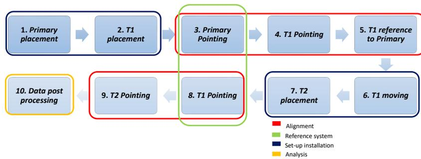
Figure 6.14: Alignment flow for STTs.
