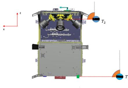
Figure 6.18: STT 2 Alignment (rotation around  $Y_{SC}$ ).
