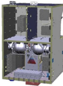
Figure 3.13: Intermediate Panel integrated on S/C.
