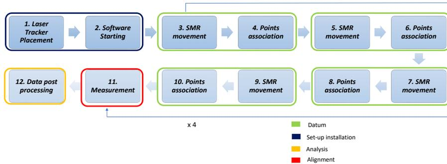
Figure 7.3: Alignment flowchart for mini-CMG.
