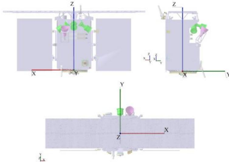
Figure 3.7: S/C Mechanical Reference Frame.
