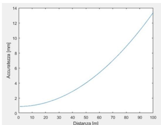
Figure 5.2: 3D Disto accuracy function.
