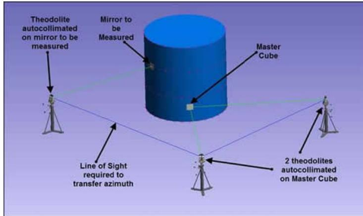
Figure 4.10: Example of Measurement Set-up with three theodolites.
