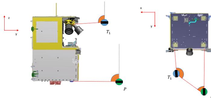
Figure 6.15: STT 1 Alignment (rotation around  $X_{SC}$  and  $Z_{SC}$ ).
