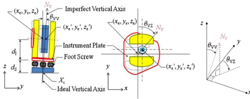
Figure 4.6: Vertical Axis error.
