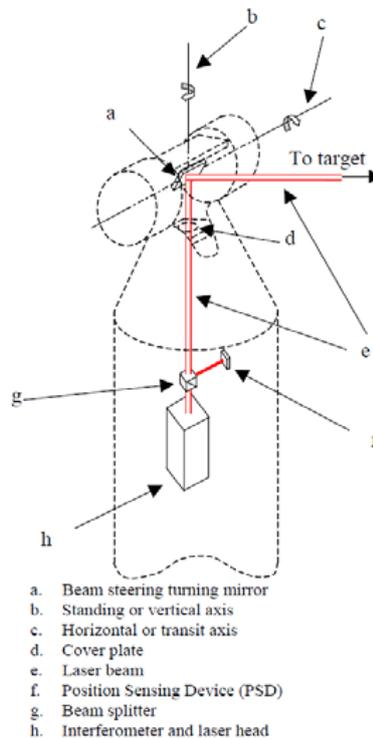
Figure 4.13: Laser tracker main axes.
