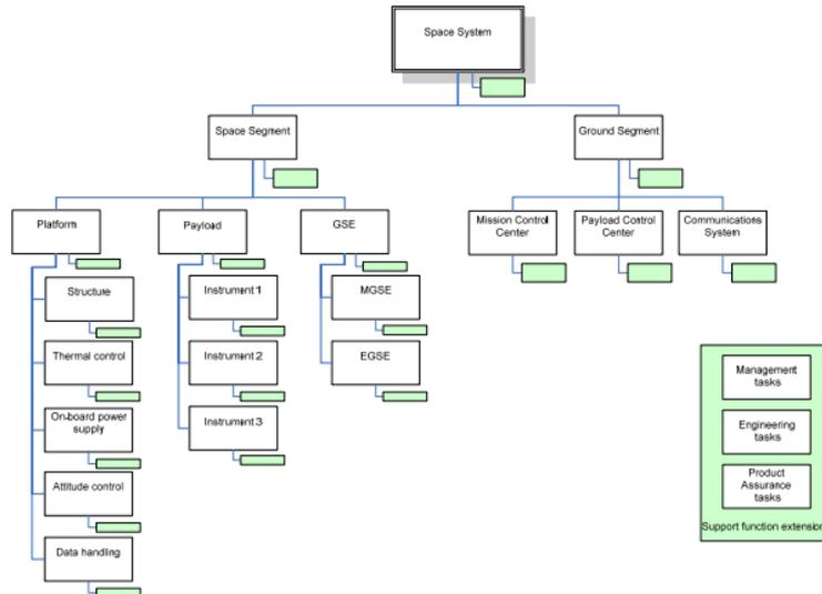
Figure 1.2: Work Breakdown tree structure.
