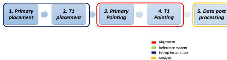
Figure 6.28: Alignment flowchart for XBA.
