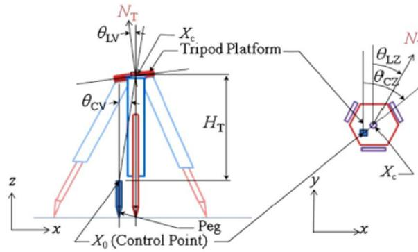
Figure 4.5: Tripod placement errors.
