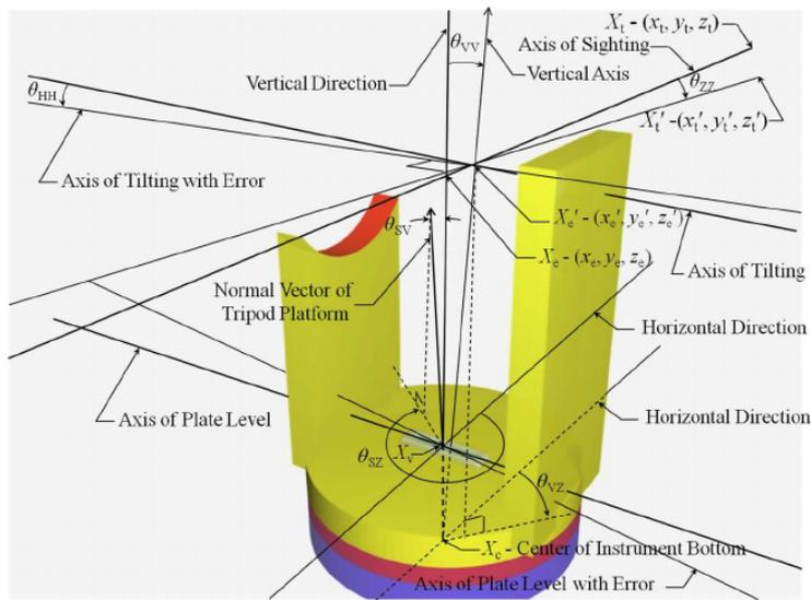
Figure 4.4: Theodolite axes displacements.
