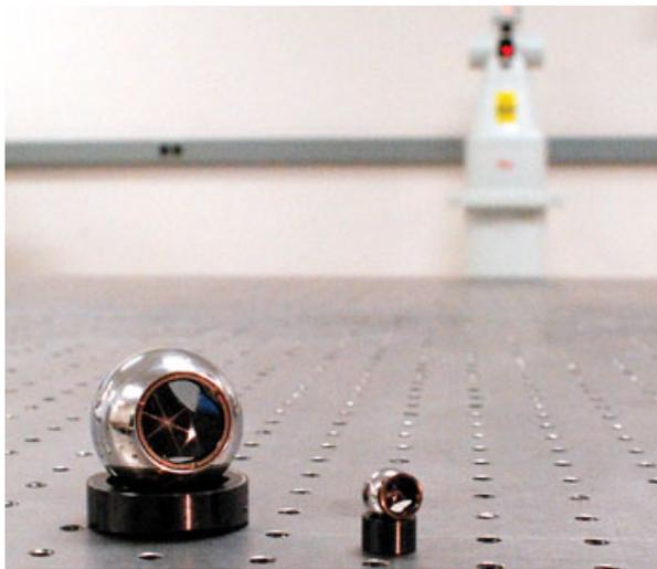
Figure 4.12: Spherical Mounted Reflectors.
