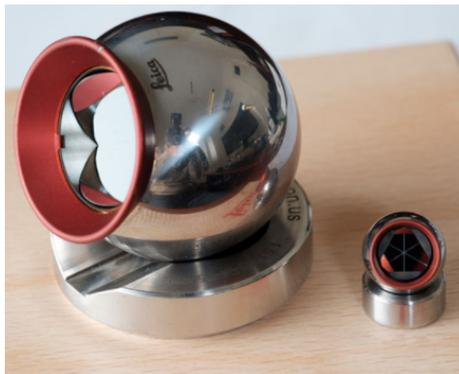
Figure 7.10: SMR of different dimensions.
