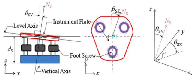
Figure 4.7: Plate level error.
