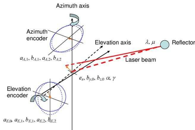
Figure 4.15: Laser tracker reference system with errors.
