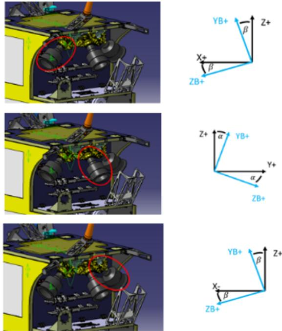
Figure 6.13: Reference system on STT1(up), STT2 (center) and STT3 (down).
