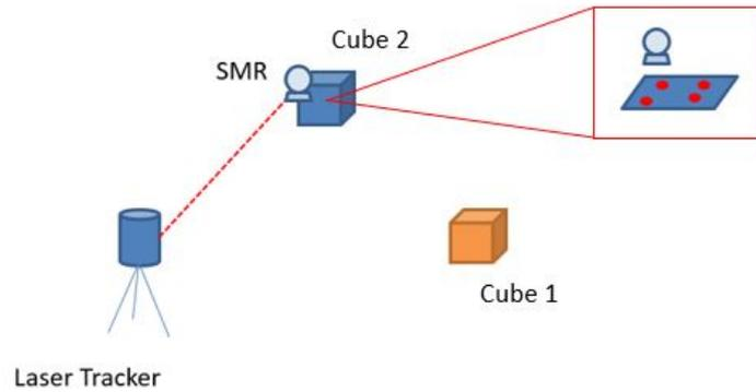
Figure 5.7: Measurement with Laser Tracker. Detail of SMR on surface.
