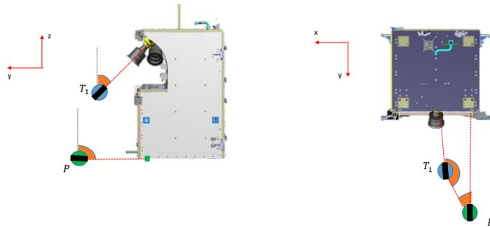
Figure 6.17: STT 2 Alignment (rotation around  $X_{SC}$  and  $Z_{SC}$ ).
