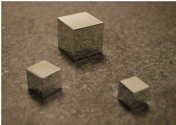
Figure 3.8: Mirror cubes of different dimensions. Cube side can typically vary between 1.5 *cm* and 2.5 *cm*.
