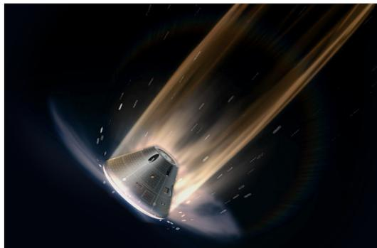
Figure 1.1: Spacecraft during atmospheric entry in the hypersonic regime. Presence of ionized gas mixture (i.e. plasma) in the region behind the strong bow shock. The picture was taken from <https://meesst.eu/technology/>.
