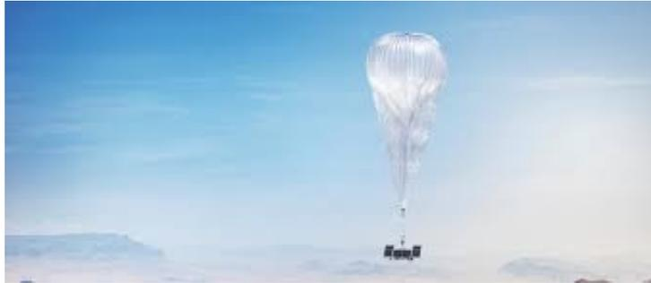
Figura 1.12: The Loon Balloon flight system
