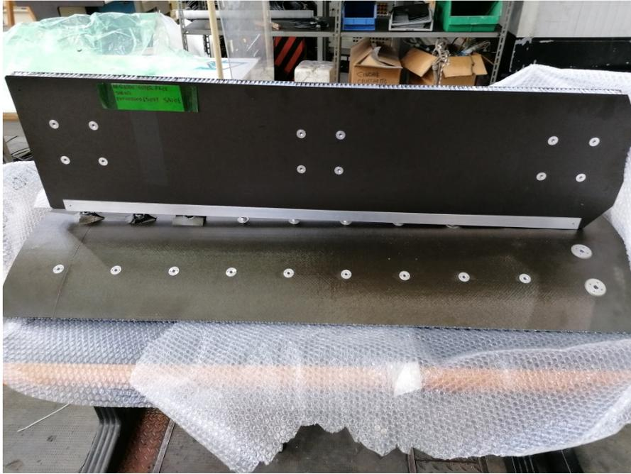
**Figure 9.4:** Photo of the coupon 2 after pullout test - *Courtesy of TAS-TO*
