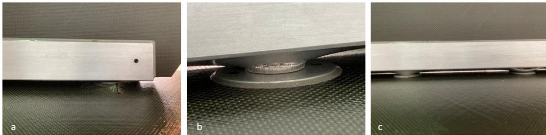
**Figure 9.10:** (a) Detail of the first insert, with the broken skin, (b) an insert which reached plastic deformation, (c) difference between two consecutive insert locations, where the cleats break in two distinct ways - *Courtesy of TAS-TO*
