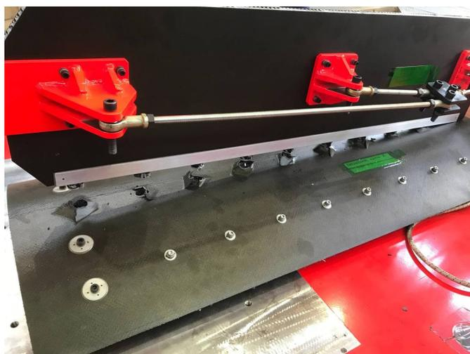
**Figure 9.7:** Axial traction coupon immediately after the test - *Courtesy of TAS-TO*
