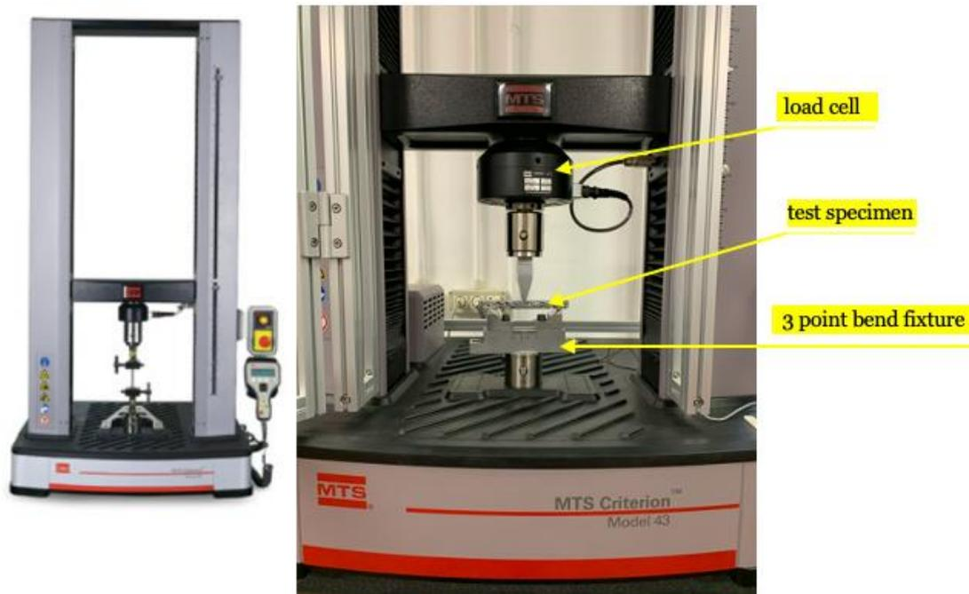
Figure 1 The test machine MTS Criterion model 43 equipped with maximum load of 50 KN
