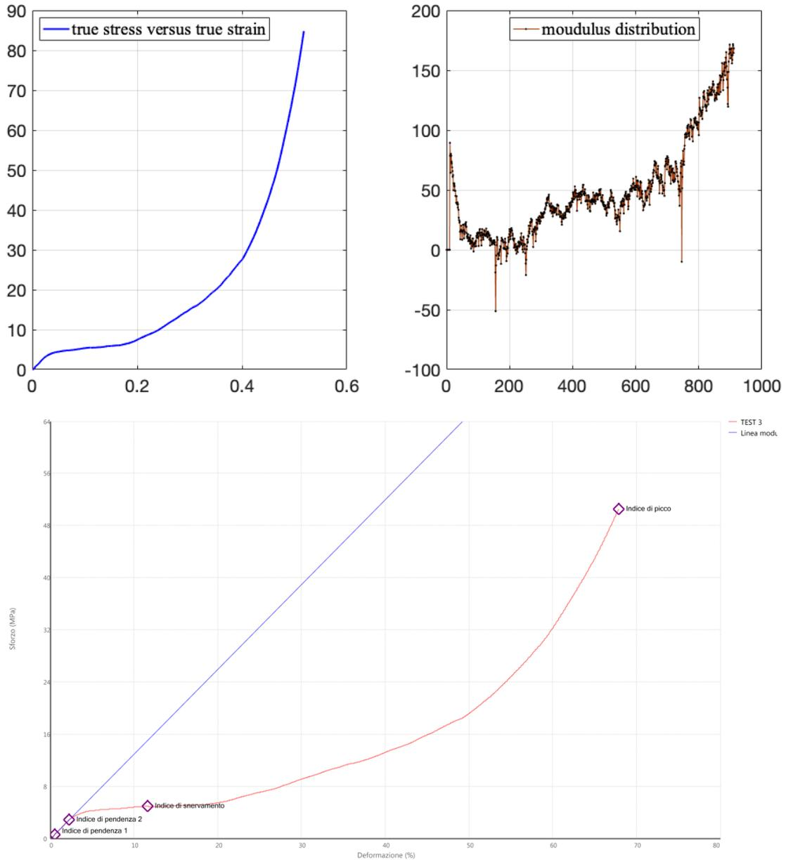
Figure 9 stress versus strain (above left), young modulus variation (above right), stress versus deformation for sample 3 (below)
