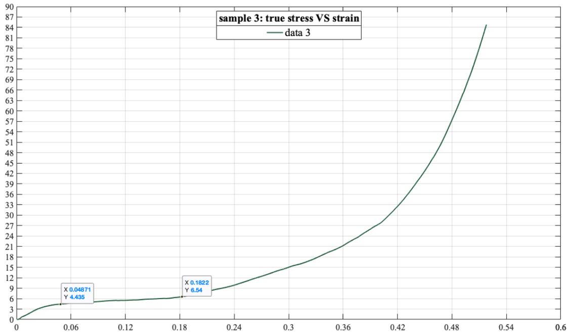
Figure 12 Compression test for sample 3: true stress [Mpa] versus strain: we could assume reasonably plateau stress and densification  $\sigma_{pl3} = 4.435 \text{ Mpa}$ ,  $\varepsilon_{D3} = 0.182$
