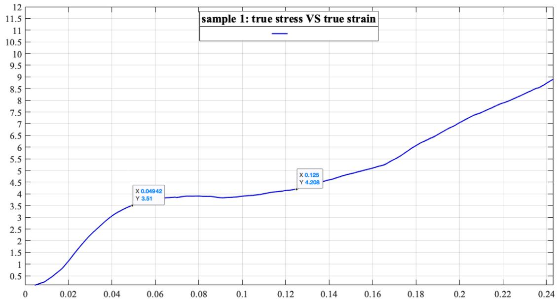
Figure 10 Compression test for sample 1: true stress [Mpa] versus strain: we could assume reasonably plateau stress and densification  $\sigma_{pl1} = 3.51 \text{ Mpa}$ ,  $\epsilon_{D1} = 0.125$
