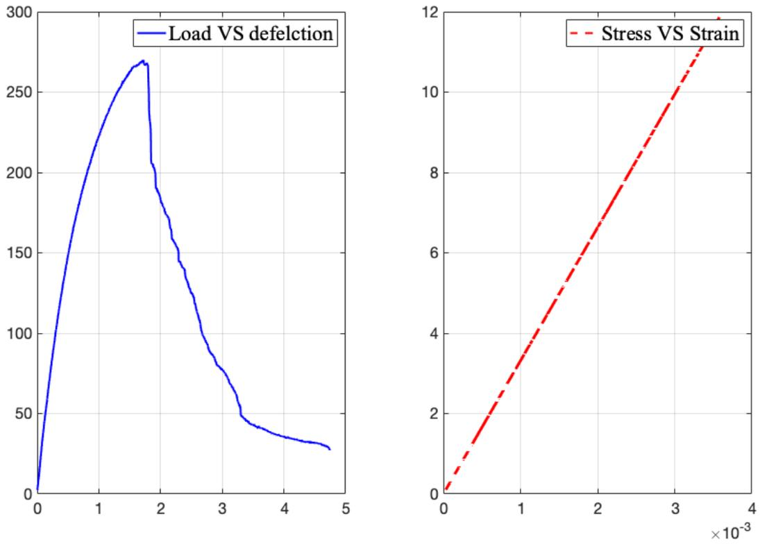
Figure 2 loads versus elongation (left) and maximum strain versus maximum stress (right)
