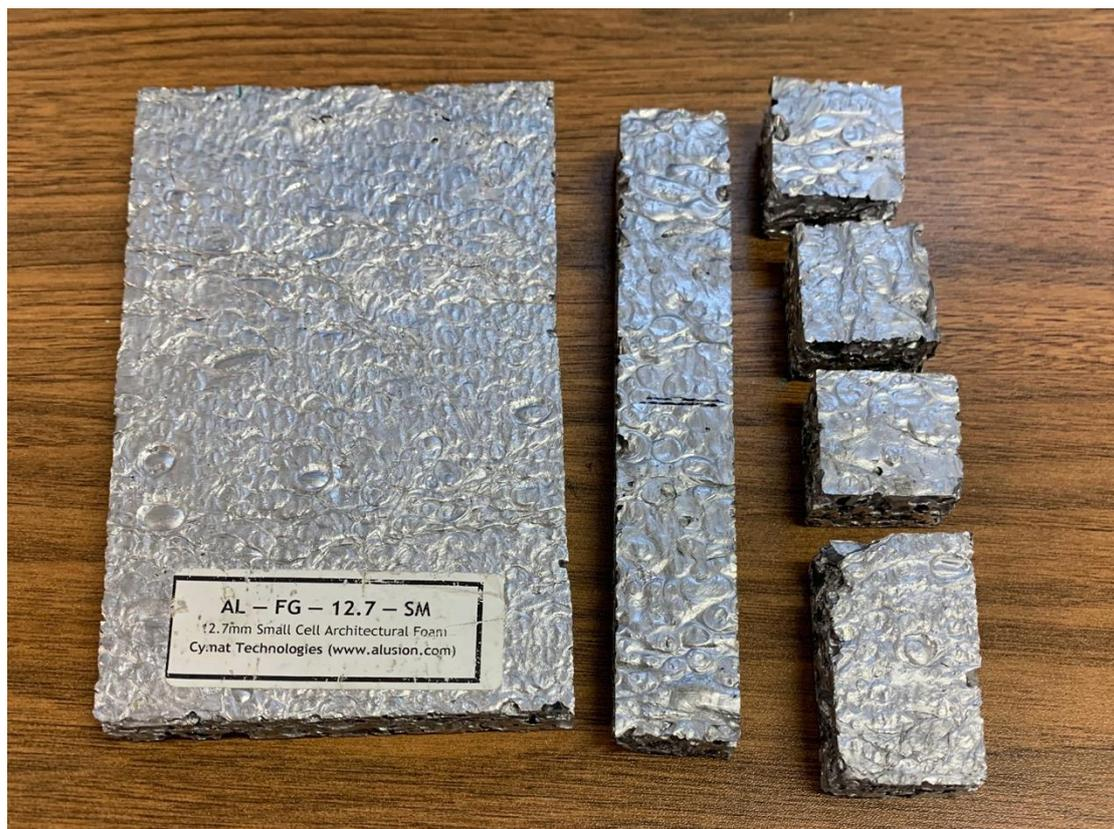
ALUSION™ Architectural Stabilized Aluminum Foam is produced by injecting air into molten aluminum, which contains a fine dispersion of ceramic particles. These particles stabilize the bubbles formed by the air, much like dry cocoa powder stabilizes bubbles when it is added to milk. Produced naturally, with a shiny shimmering silver
