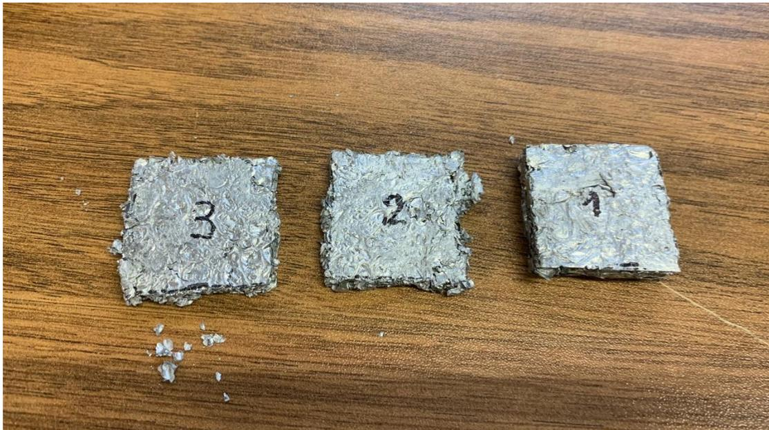
Figure 5 only first sample has been partially compressed, the others have totally been compressed.
