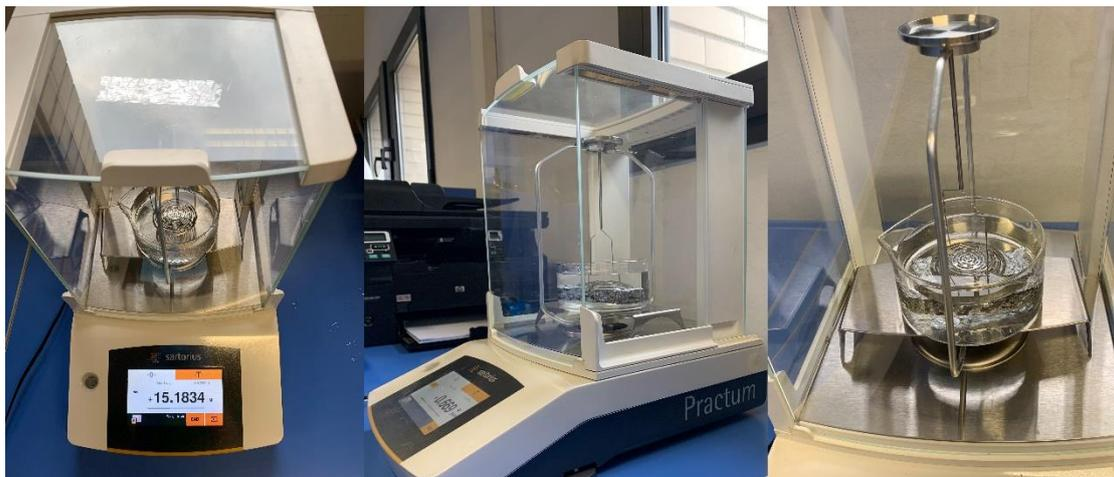
Figure 14 configuration of Sartorius YDK03 and sample been immersed to read density
