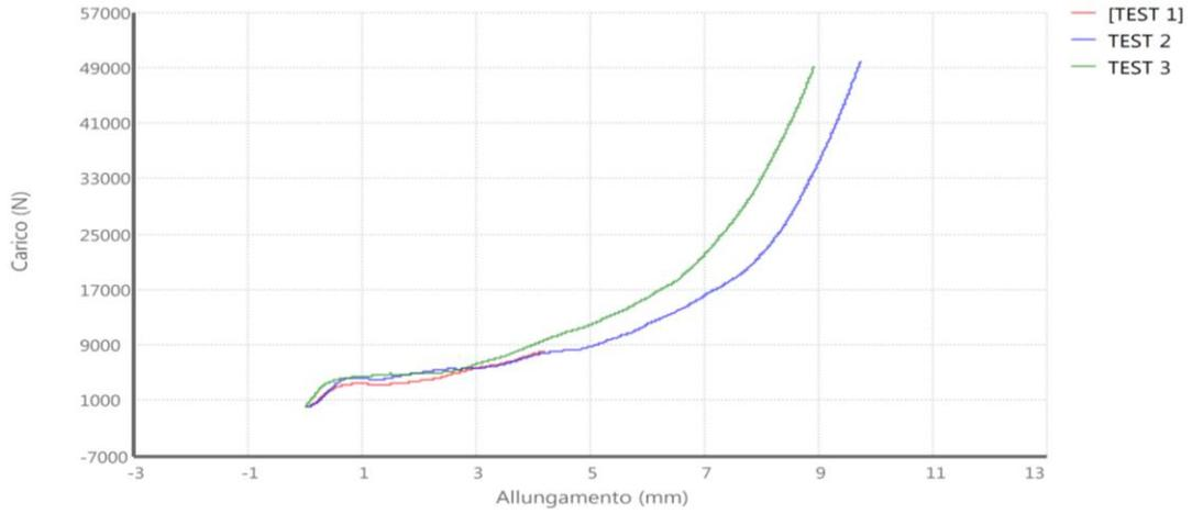
Figure 6 load versus deformation for 3 samples
