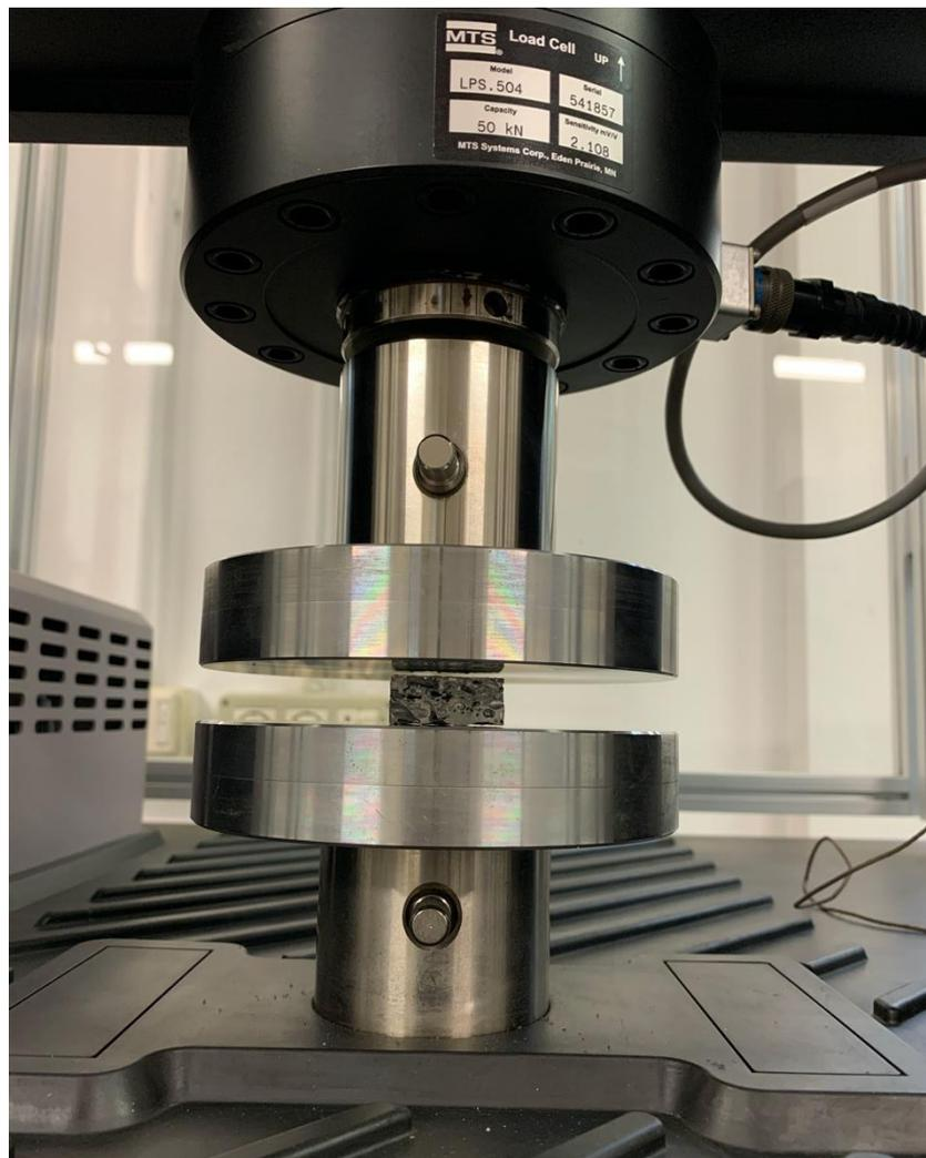
Figure 4 compression set up.
