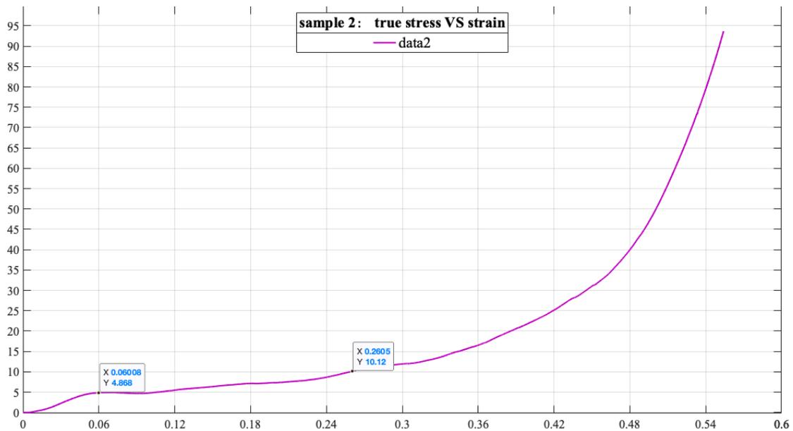
Figure 11 Compression test for sample 2: true stress [Mpa] versus strain: we could assume reasonably plateau stress and densification  $\sigma_{pl2} = 4.868 \text{ Mpa}$ ,  $\epsilon_{D2} = 0.26$
