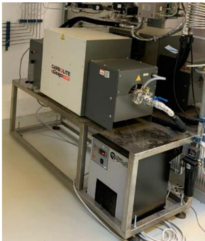
Figure 3.2: Carbolite Gero tubular microreactor.
