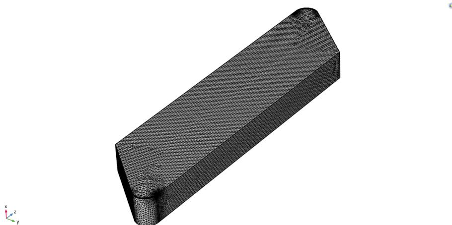
Figure 6.7 - Mesh generated for simulation of hydrodynamics inside electrochemical flowcell
