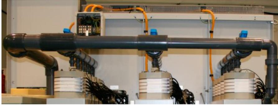
Figure 4.6- Stacking of cells in a 1 m<sup>2</sup> pilot plant for the electrolysis of wastewater
