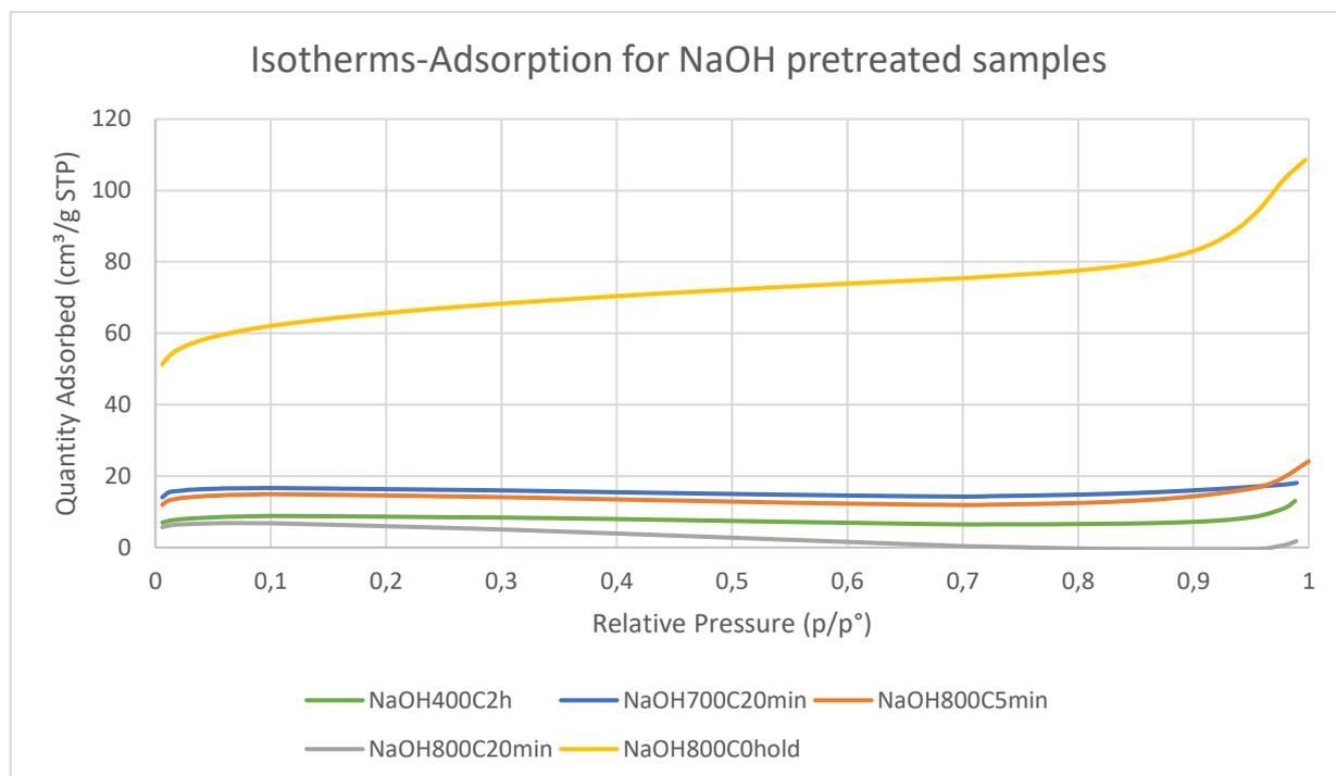
Figure [85],  $N_2$  adsorption isotherm curves for NaOH samples, author's elaboration.
