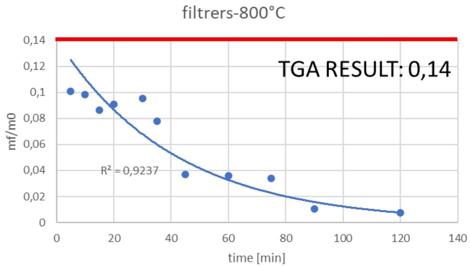
Figure [66], Evolution of the mass residue with the hold time at 800°C compared to TGA result, author's elaboration.
