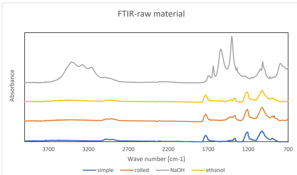
Figure [67], FTIR profiles for raw materials, author's elaboration.
