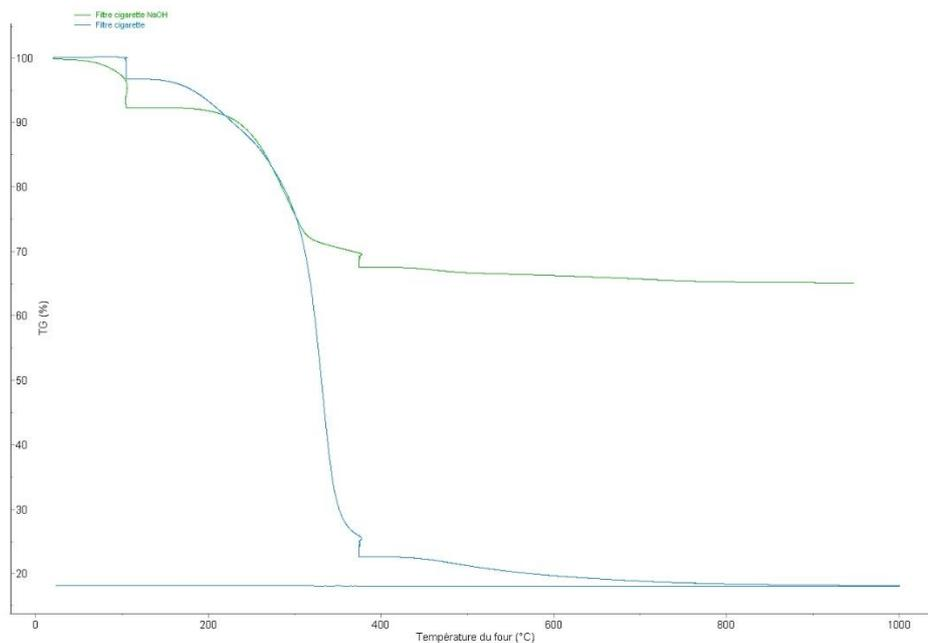
Figure [50], Comparison of TGA of filters (blue) and NaOH pre-treated filters (green), author's elaboration.
