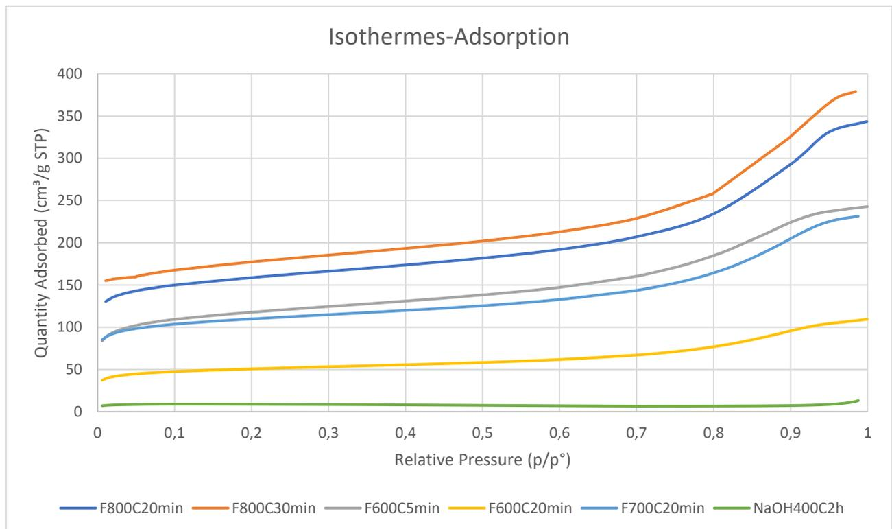
Figure [84], N<sub>2</sub> adsorption isotherm curves, author's elaboration.
