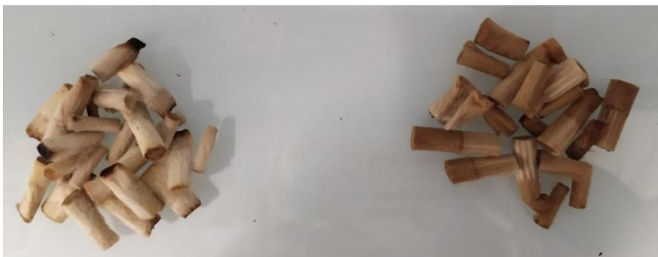
*Figure [33]. Filters before and after the ethanol pre-treatment, author's picture.*
