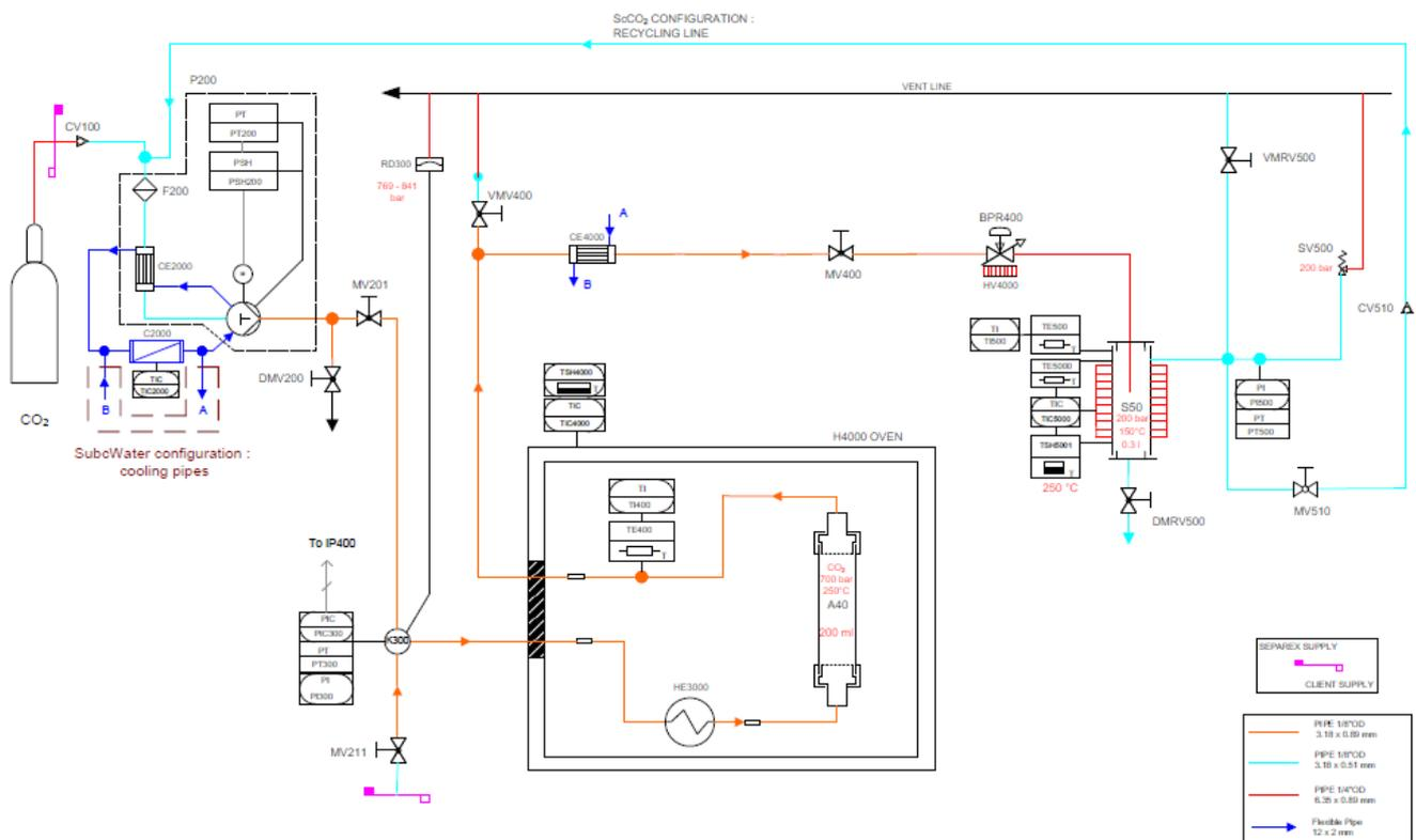
Figure [37] P&ID of the Supercritical Fluid Equipment, modified from [35].
