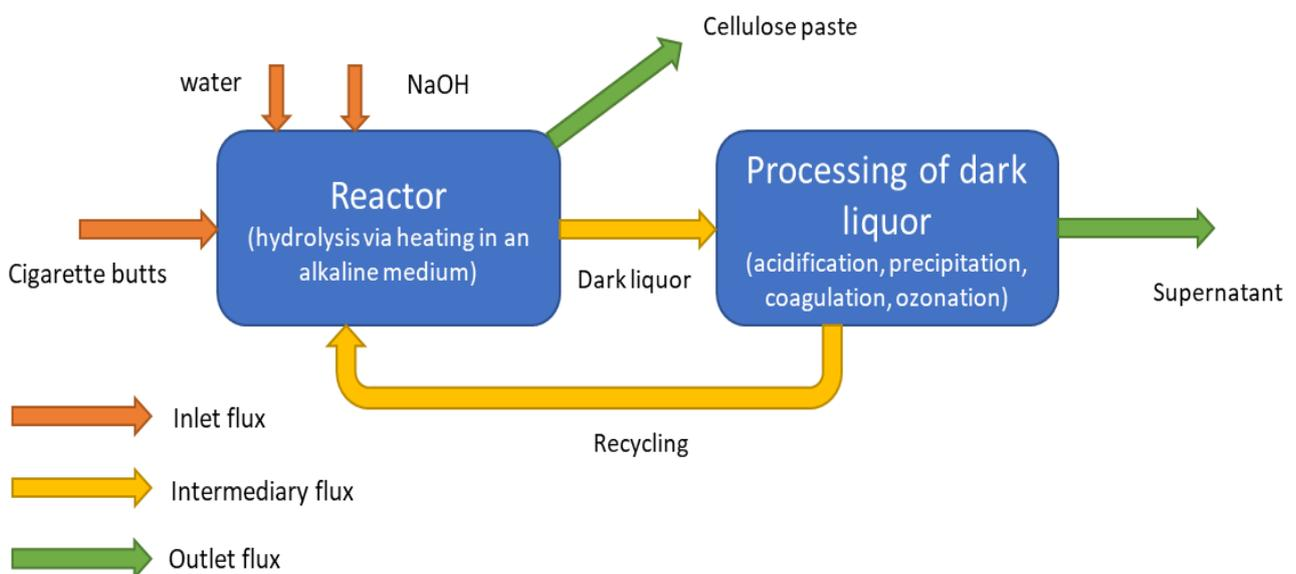
Figure [26], Diagram of the recovery process used by Poiato Recicla, modified from [36].
