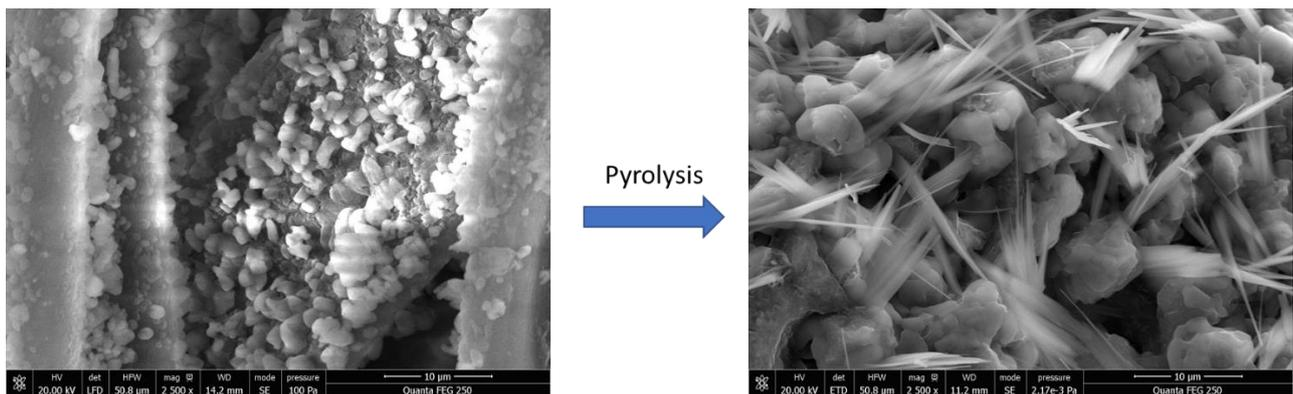
Figure [80], SEM of NaOH filters before and after pyrolysis, author's elaboration.
