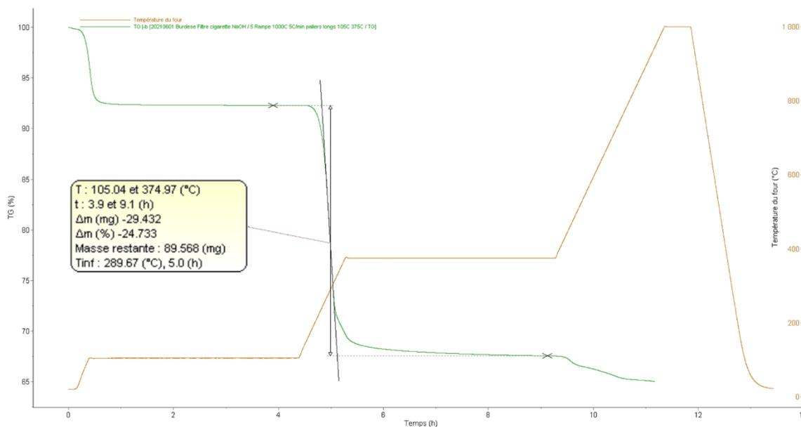
Figure [49], TGA of NaOH pre-treated filters, author's elaboration.
