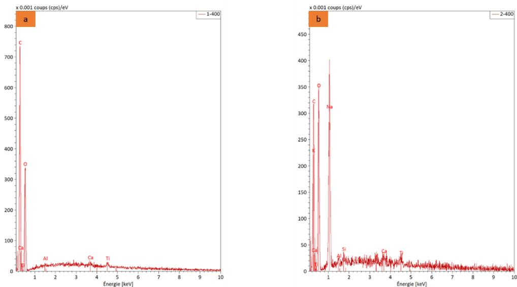
Figure [72], EDX of normal filters (a) and NaOH pre-treated filters (b), author's elaboration.
