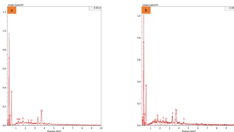
Figure [74], EDX of rolled CB's filters at 50 $\mu\text{m}$  (a) and 400 $\mu\text{m}$  (b), author's elaboration.
