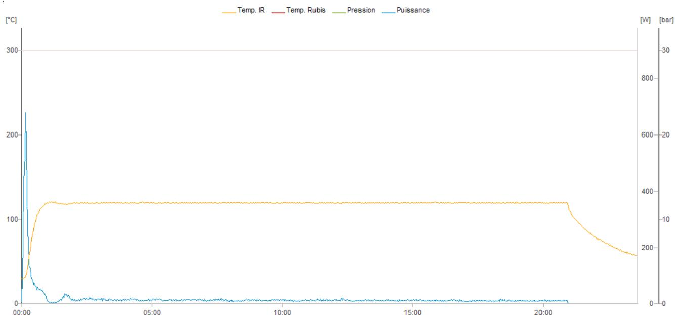
Figure [40], Profiles of temperature, power and pressure in microwave treatment, author's elaboration.
