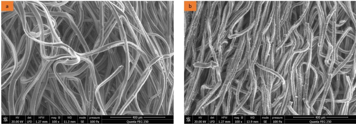
Figure [70], SEM of normal filters (a) and NaOH pre-treated filters (b), author's elaboration.
