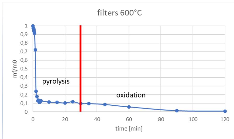
Figure [57], Evolution of the mass residue with the hold time at 600 °C for CBs' filters 0-120 minutes, author's elaboration.
