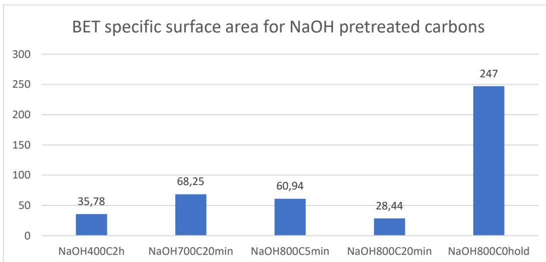
Figure [91], BET specific surface area for NaOH pre-treated carbons, author's elaboration.
