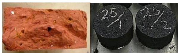
Figure [8] and [9], Fired clay bricks (left) and Asphalt concrete (right), modified from [11].
