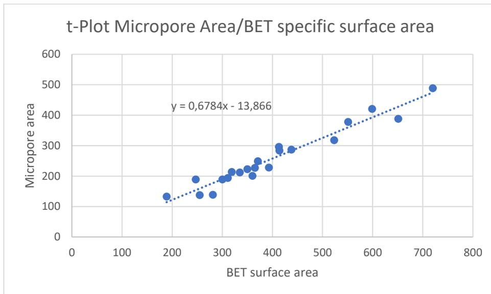
Figure [88], Micropore Area/BET specific surface area, author's elaboration.
