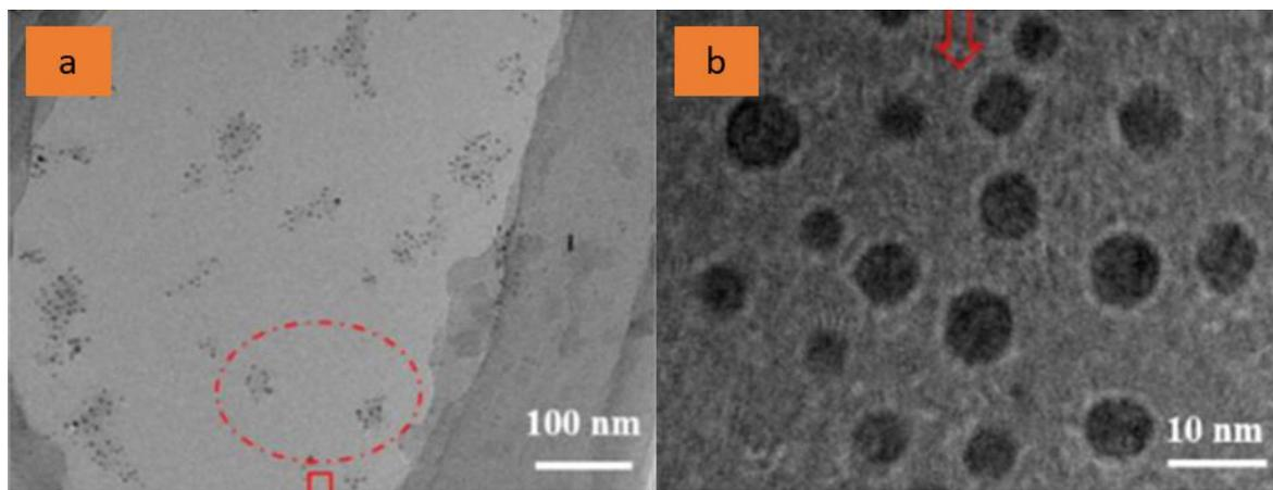
Figure [20], S/TEM images of Pd@CCB catalysts at two levels of magnification, modified from [1].
