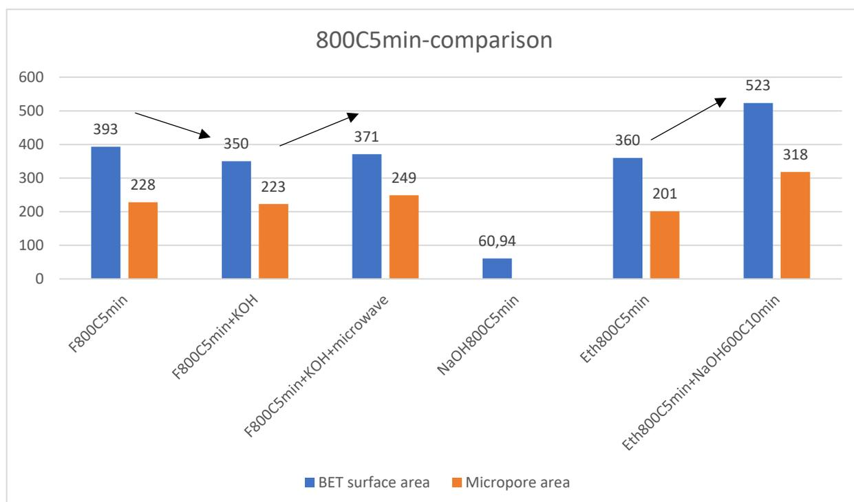
Figure [92], Comparison of the BET specific surface area for 800°C and 5 minutes samples, author's elaboration.
