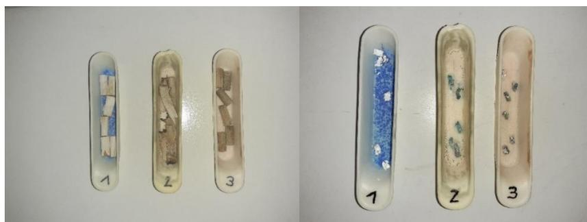
Figure [31], Before (left) and after (right) carbonisation at 800°C, author's elaboration.
