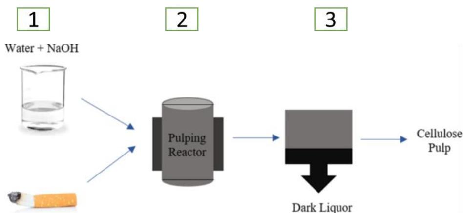
Figure [10], Cellulose pulp production scheme, modified from [11].
