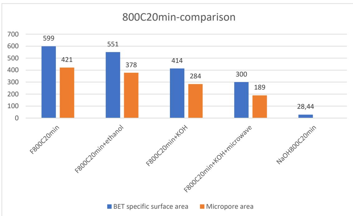
Figure [93], Comparison of the BET specific surface area for 800°C and 20 minutes samples, author's elaboration.
