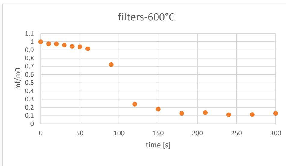
Figure [56], Evolution of the mass residue with the hold time at 600 °C for CBs' filters 0-5 minutes, author's elaboration.
