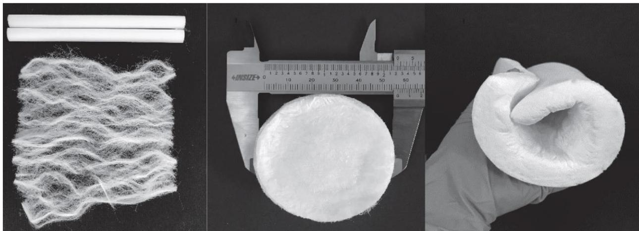
Figure [12], CA fibres and cellulose acetate aerogel, modified from [6].
