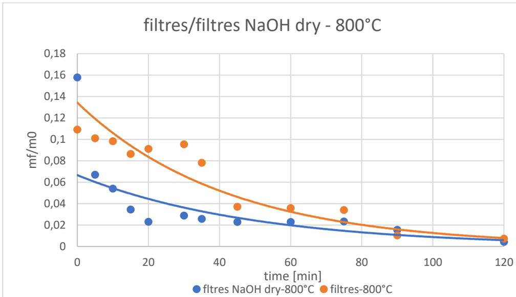
Figure [61], Comparison, at 800°C, between normal filters and NaOH filters, author's elaboration.
