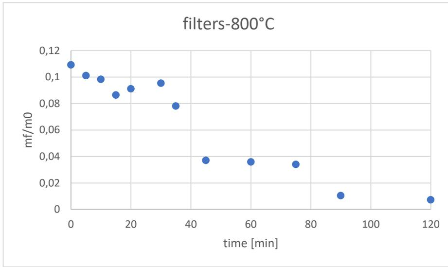
Figure [52], Evolution of the mass residue with the hold time at 800°C for CBs' filters, author's elaboration.
