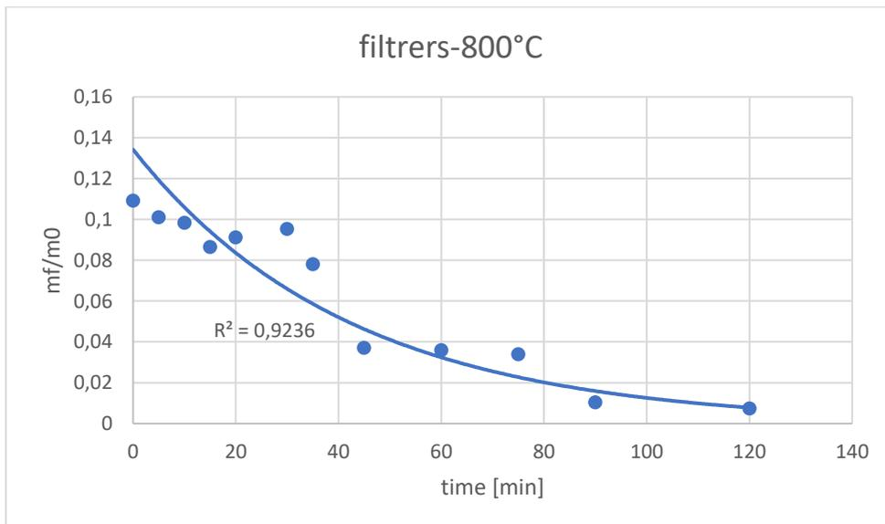
Figure [53], Evolution of the mass residue with the hold time at 800°C for CBs' filters, author's elaboration.
