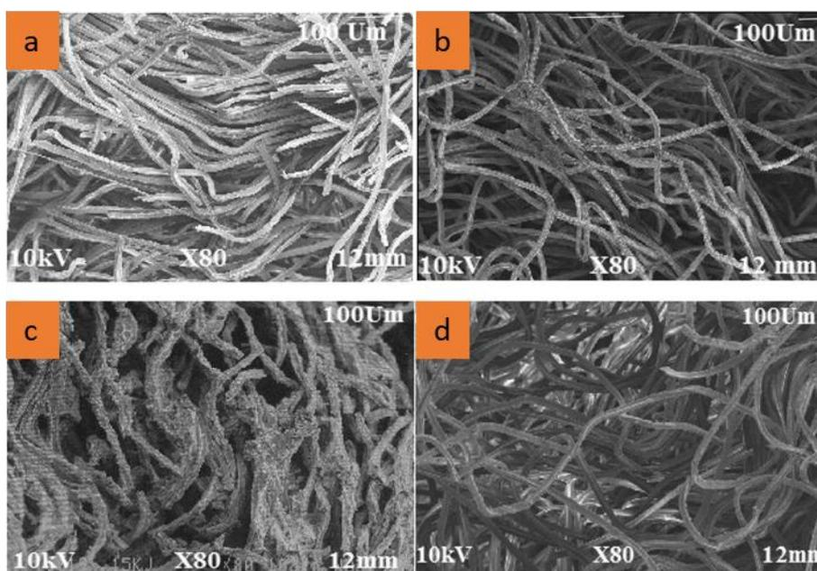
Figure [14], SEM of the pre-carbonisation cellulose acetate fibres with different NaOH ratios, modified from [5].
