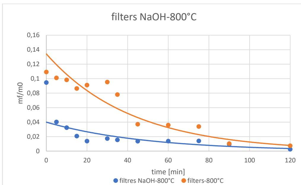
Figure [60], Comparison, at 800°C, between normal filters and NaOH filters, author's elaboration.
