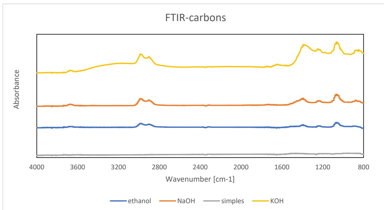
Figure [69], FTIR profiles for manufactured carbons, author's elaboration.
