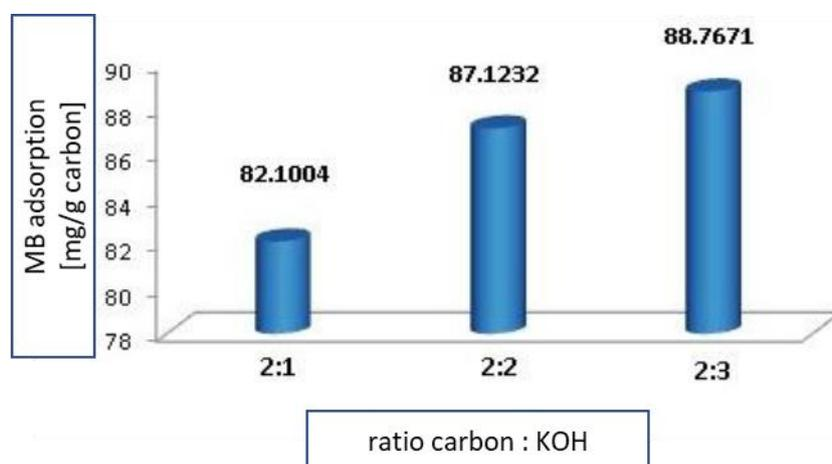
Figure [16], MB adsorption capacity for different sample, from [4].
