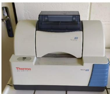
Figure [43], Thermo Scientific Nicolet iS5 FTIR spectrometer for FTIR, author's elaboration.
