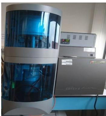
*Figure [42], Setaram SETSYS-1750 CS for TGA, author’s elaboration.*
