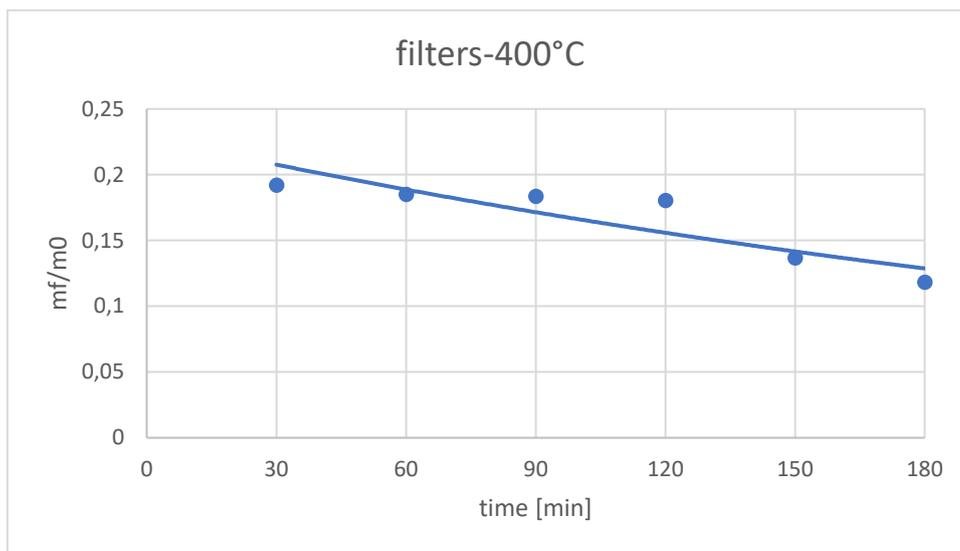
Figure [55], Evolution of the mass residue with the hold time at 400 °C for CBs' filters, author's elaboration.
