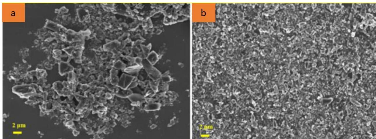
Figure [19], FE-SEM images of CCB (g) and Pd@CCB (h), modified from [1].
