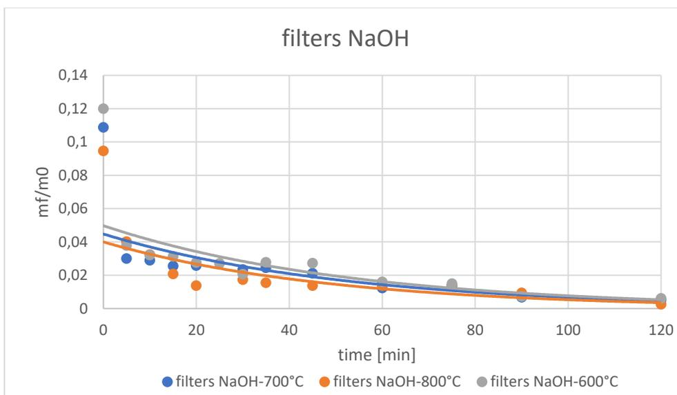
Figure [62], Comparison between NaOH filters at 600, 700 and 800°C, author's elaboration.
