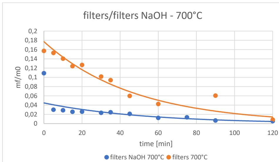
Figure [63], Comparison, at 700°C, between normal filters and NaOH filters, author's elaboration.
