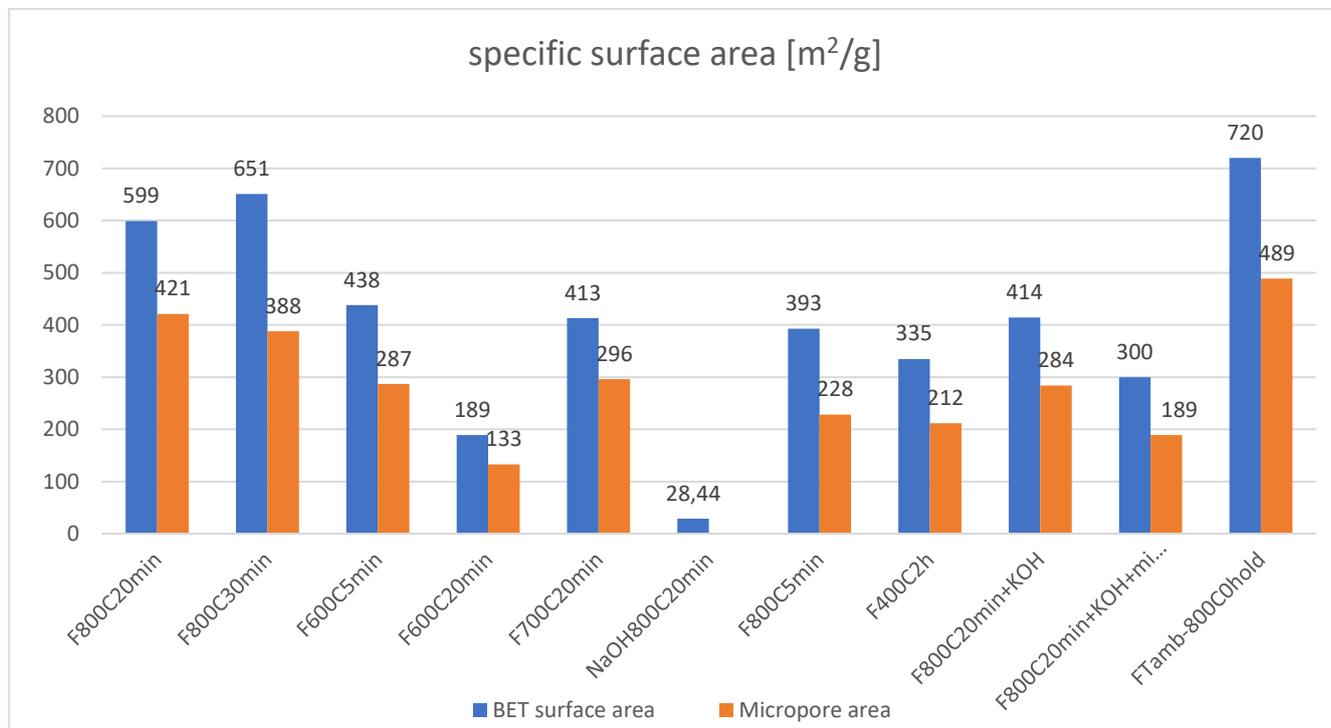
Figure [89], Micropore Area and BET specific surface area, author's elaboration.
