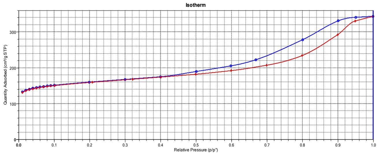
Figure [83], F800C20min isotherm adsorption-desorption curve, author's elaboration.
