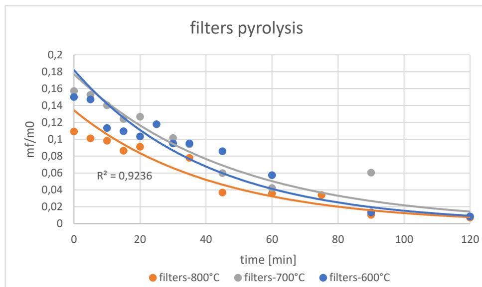
Figure [54], Evolution of the mass residue with the hold time at 800, 700 and 600°C for CBs' filters, author's elaboration.
