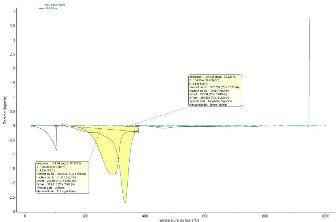
Figure [51], Comparison of TGA of filters (blue) and NaOH pre-treated filters (green), author's elaboration.
