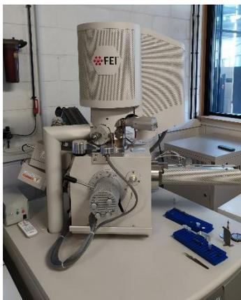
Figure [44], Quanta FEG 250 for SEM, author's elaboration.
