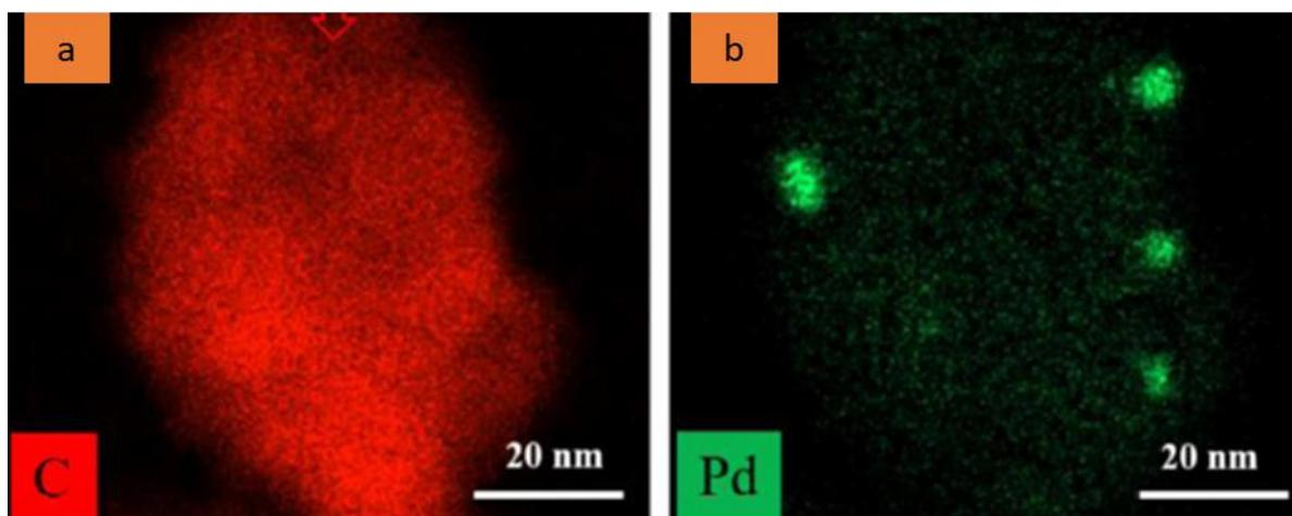
Figure [21], EDS mapping of Pd@CCB catalysts, modified from [1].
