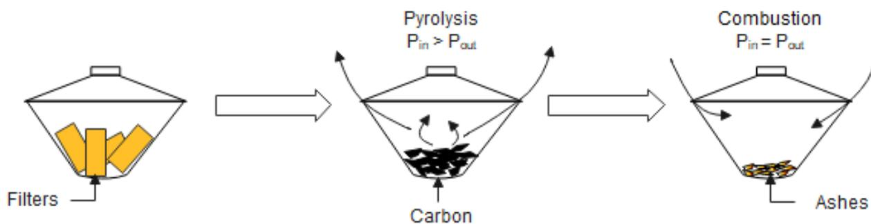
Figure [32], Simulation of the process that happens in the furnace, author's elaboration.
