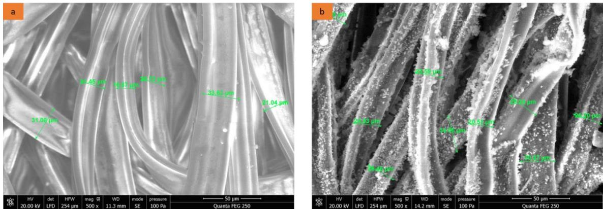
Figure [71], SEM of normal filters (a) and NaOH pre-treated filters (b), author's elaboration.
