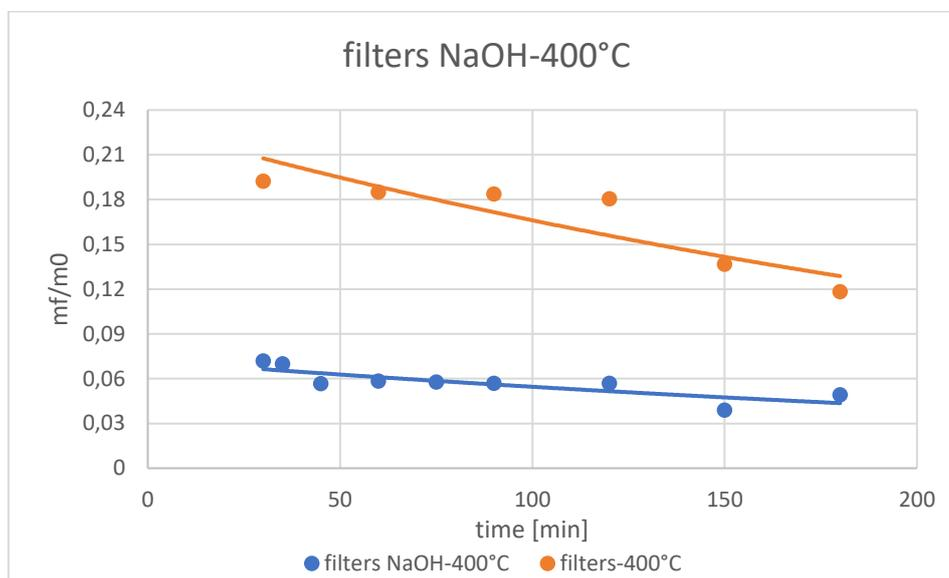
Figure [65], Evolution of the mass residue with the hold time at 400°C for NaOH filters, author's elaboration.
