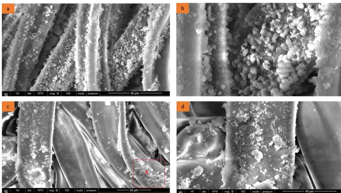
Figure [73], SEM of NaOH pre-treated filters (a, b) and rolled filters (c, d), author's elaboration.
