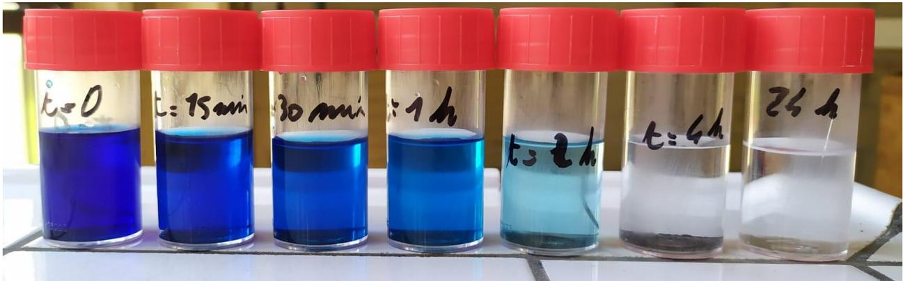
*Figure [82], Methylene blue adsorption test, author's elaboration.*
