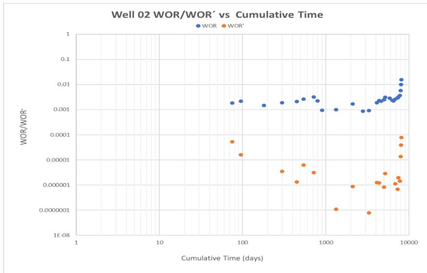
Figure 5-19 Well Diagnostic Plot showing WOR and WOR' vs Cumulative Time (Bill Bailey et al, 2000).
