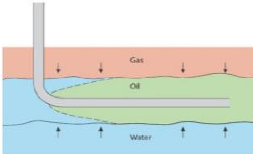
Figure 2-11 Horizontal well schematic (Anietie N. Okon et al, 2017).
