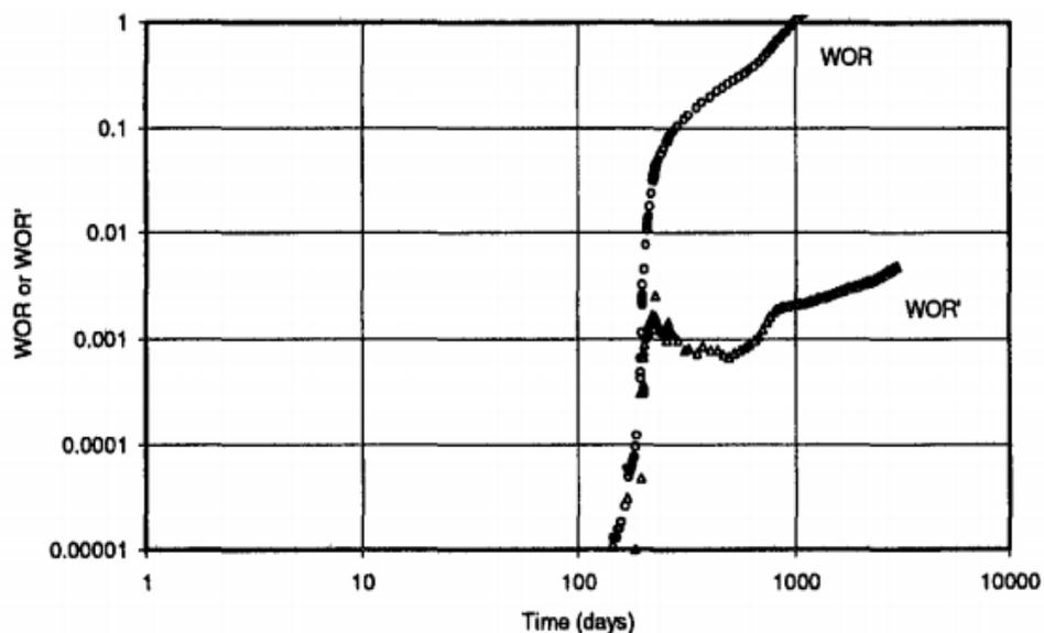
Figure 3-5 WOR and WOR' derivatives for thief layer water recycling (K.S. Chan 1995)
