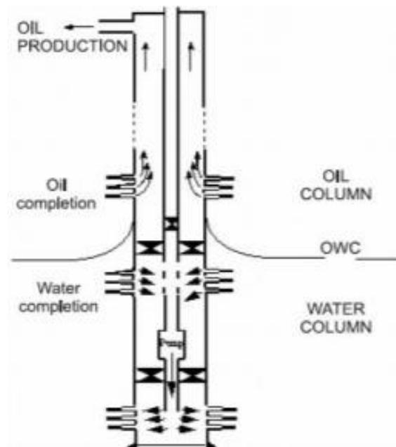
Figure 2-10 Downhole water loop schematic (Anietie N. Okon et al, 2017).
