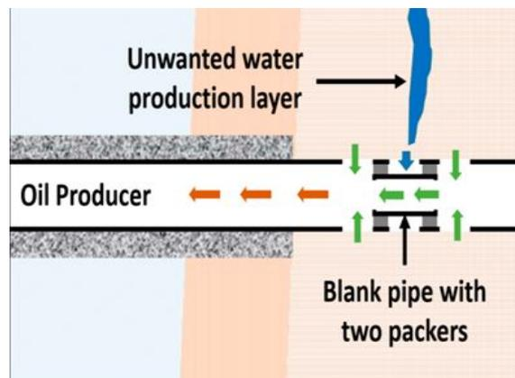
Figure 2-5 Two packers above and below a blank pipe to shut-off water production from middle and upper part (Abdullah Taha, et al. 2019)
