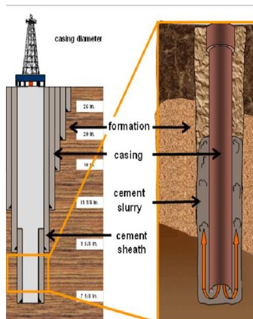
Figure 2-12 oil well squeeze cementing schematic (Drillingcourse.com, 2015)
