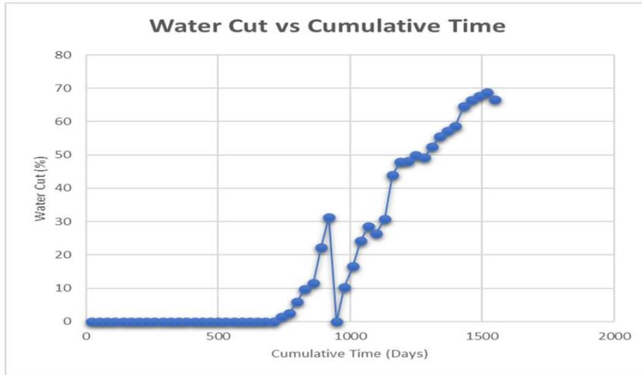
Figure 5-14 Water cut (%) vs Time graph (Mohammed Mahgoup et al, 2015).
