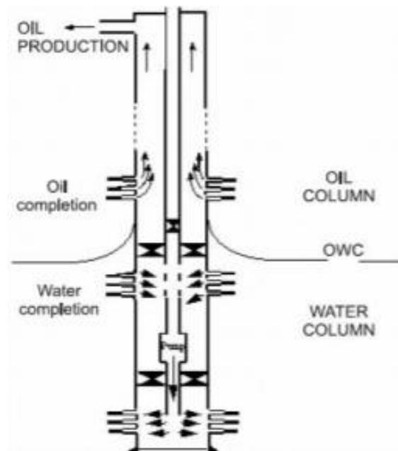
Figure 2-10 Downhole water loop schematic (Anietie N. Okon et al, 2017).
