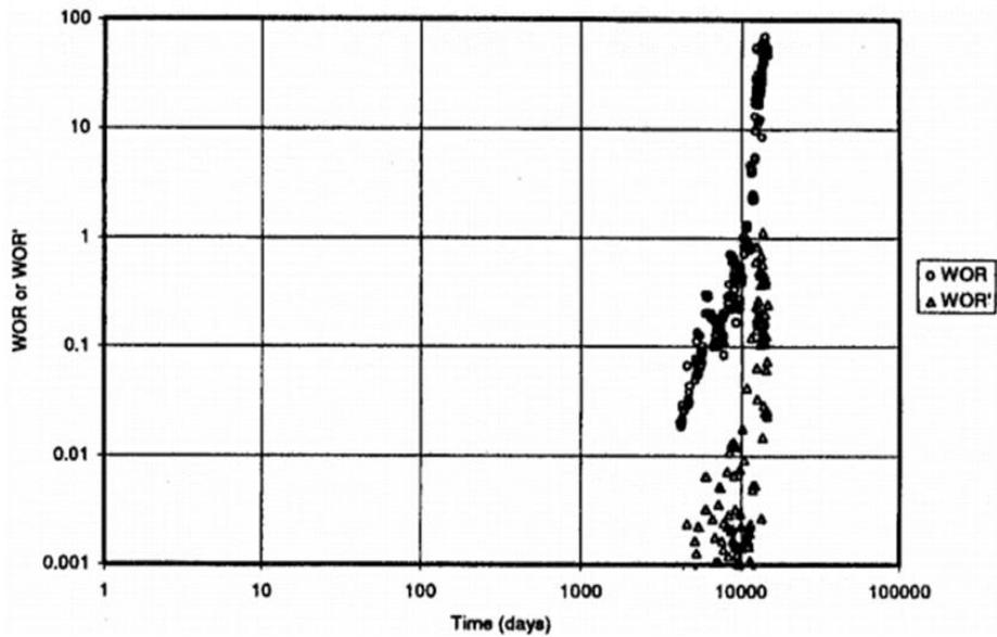
Figure 3-7 Field Example Rapid Channeling. (K.S. Chan, 1995).
