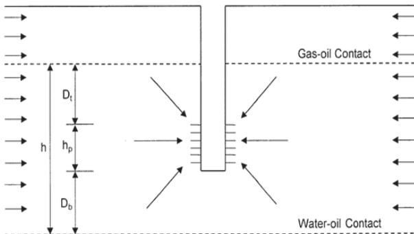
Figure 2-1 Original reservoir at static condition (Ahmed Tarek, 2010)
