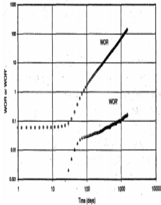
Figure 3-3 Multilayer channeling WOR and WOR' (Chan, 1995)
