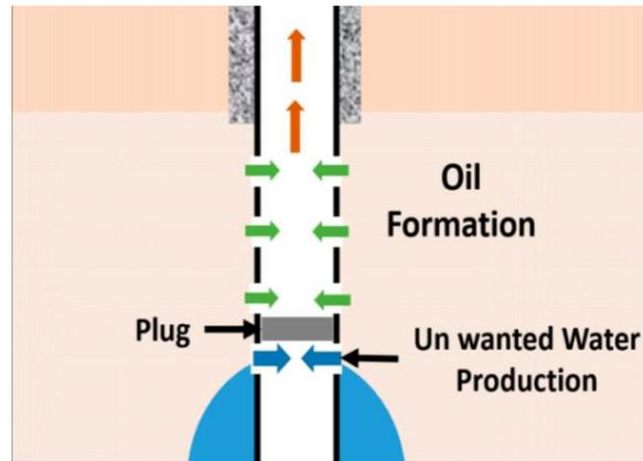
Figure 2-4 Using plug to shut off the production of water from the bottom (Abdullah Taha, et al. 2019)
