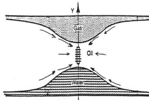
Figure 2-2 A producing well with Coning. (Ahmed Tarek, 2010)
