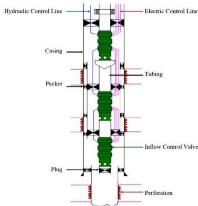
Figure 2-6 Intelligent Well Completion Schematic, showing all components (Anietie N. Okon et al, 2018).
