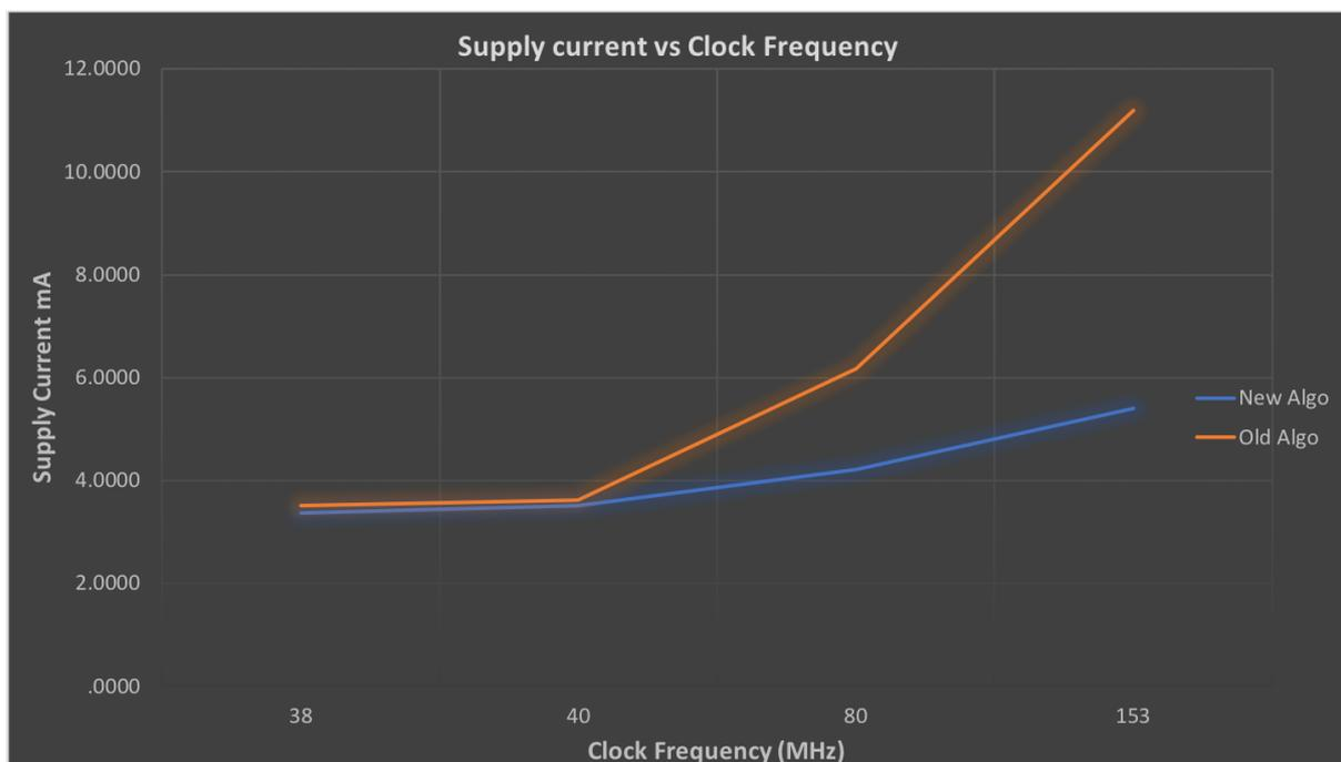
Figure 11: Current supply versus the clock frequency, running the first version of the software and the new algorithm.
