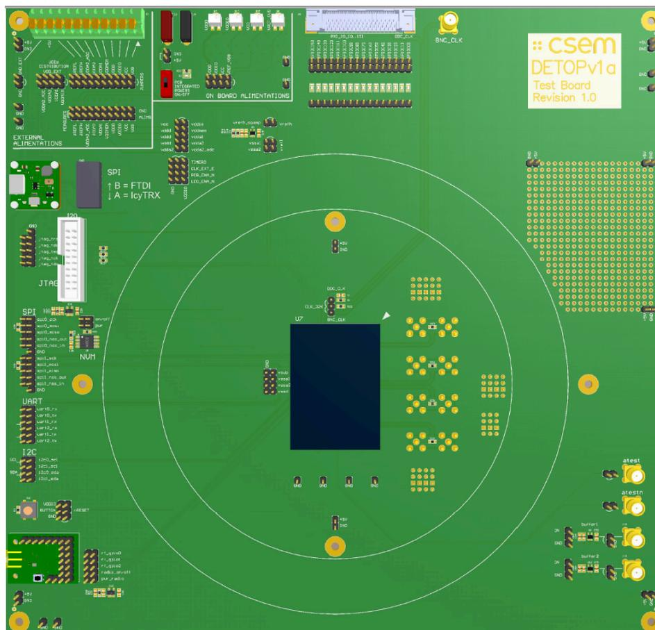
Figure 8 : Test board for the DeTOP Chip designed and assembled on CSEM. This board is providing easy access to all the peripherals and supplies of the DeTOP chip that are needed for the characterization and also has a wide area in the middle to force temperature on the chip, if it is needed to be characterized on a specific temperature regime.
