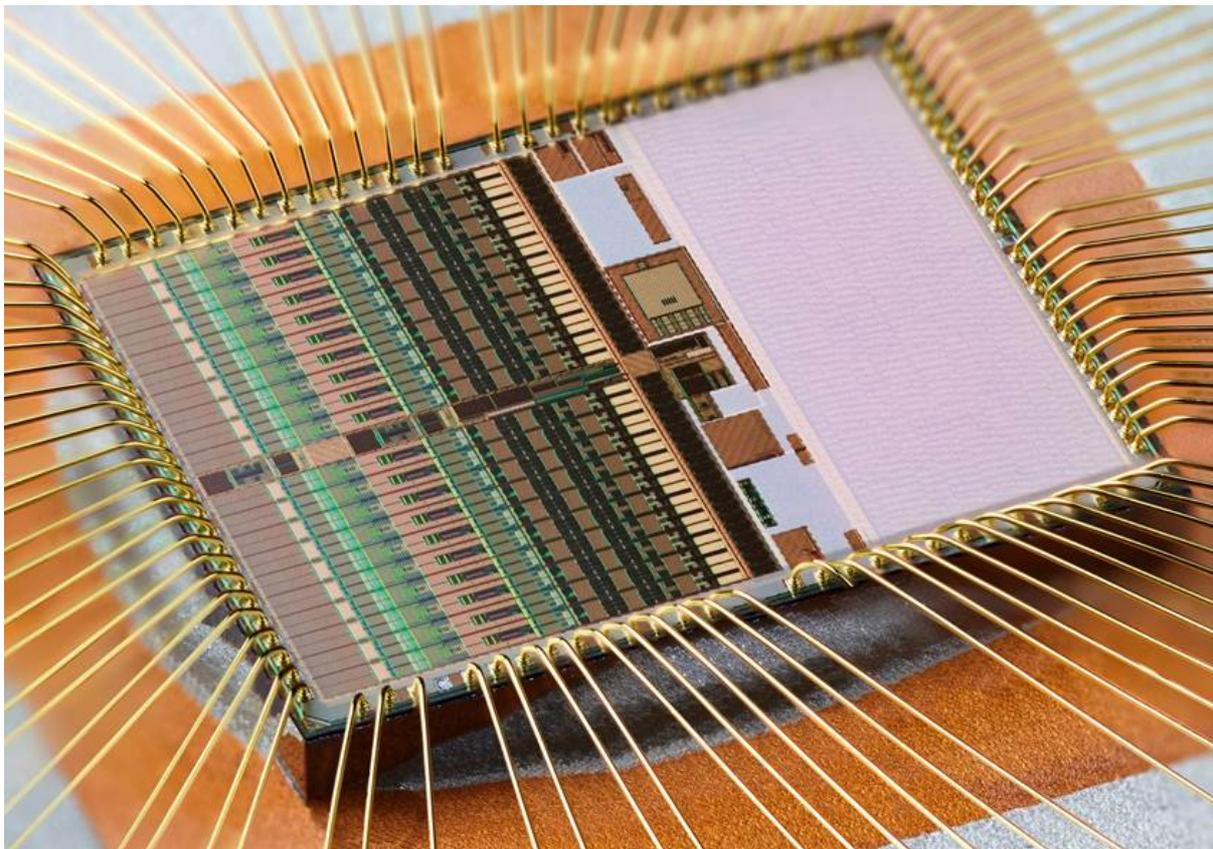
*Figure 5 : Photo of the DeTOP chip, taken before packaging. On this photo the Digital part is on the right and the Analog part is on the left, where one can see that the analog transistors are much wider. 55nm transistor technology is employed, on the TSMC fab. The process of the chip used is TT.*
