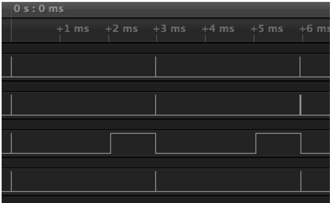
Figure 15 : Timing of the software with a clock frequency of 40 MHz
