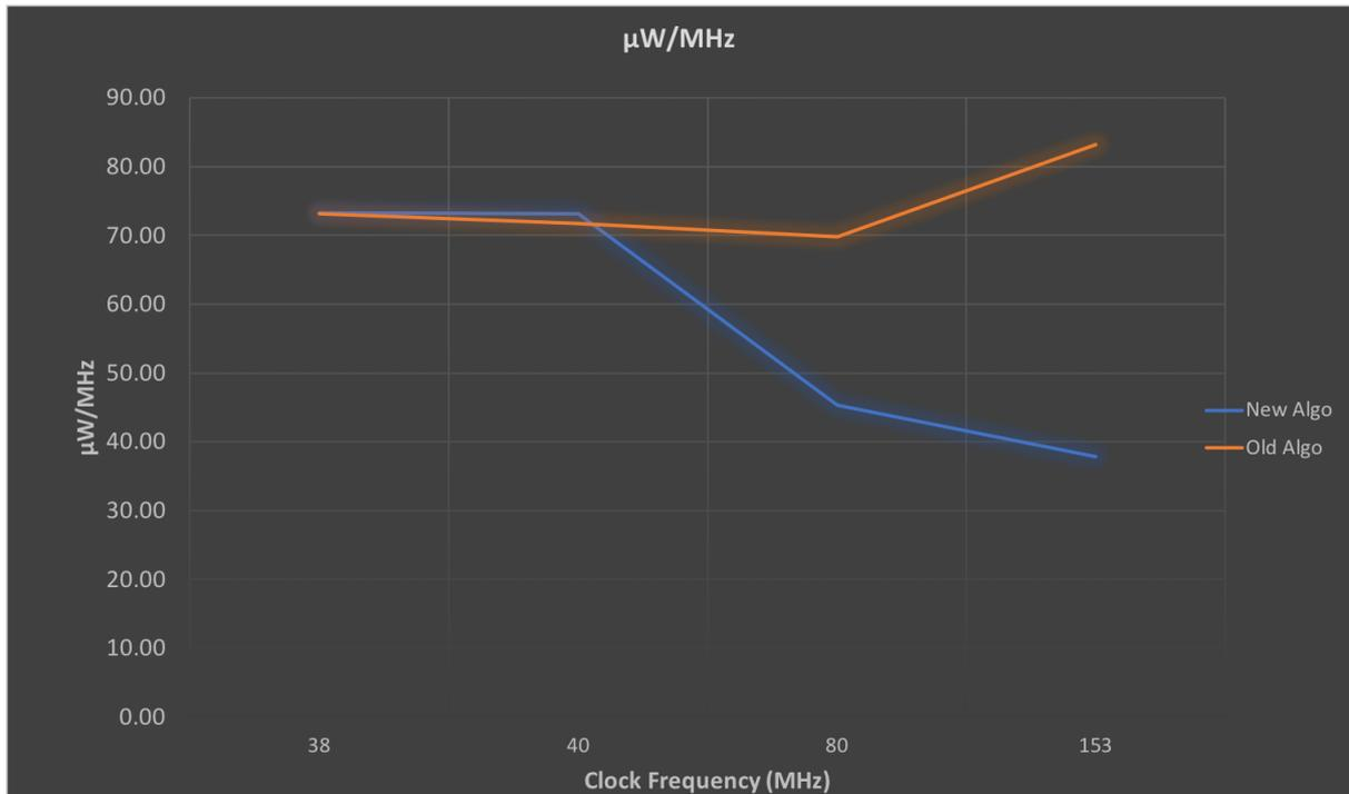
Figure 12: Dynamic Power consumption versus the Clock frequency
