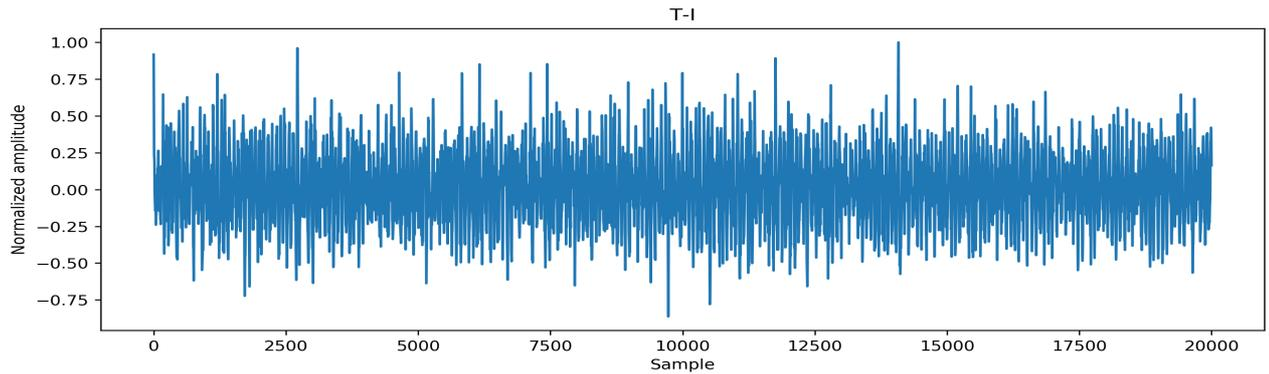
Figure 4: EMG signal of the arm muscles while the Thumb is contracting to touch the index. On the x axis one can observe the number of samples while on the y axis, it's the amplitude of the EMG signal. The amplitude is normalized to the value of 1, on a symmetric way, leaving the zero potential to be on the zero value and not from peak to peak. The data used are EMG recordings, processed and plotted by a python script.
