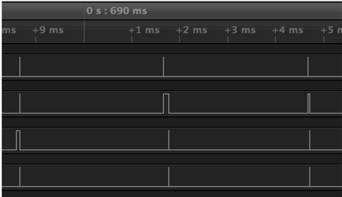
Figure 17: Timing of the software with a clock frequency of 25 MHz
