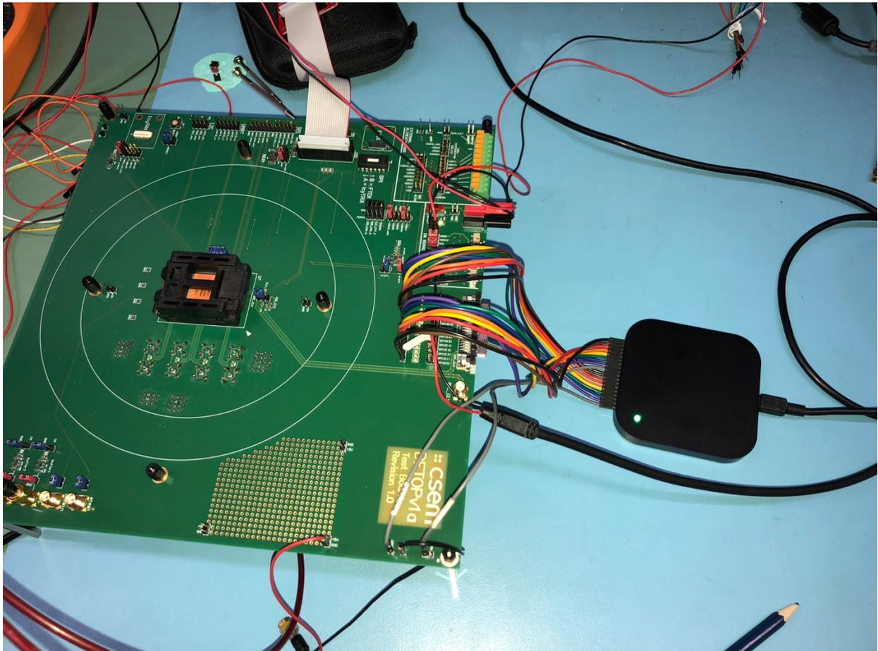
*Figure 9: Testing environment. The DeTOP chip is mounded on the test board. The software is loaded using a JTAG board, and the GPIO (General Purpose Input Output) ports are connected with a logic analyzer, used to evaluate the timing and several software flags*
