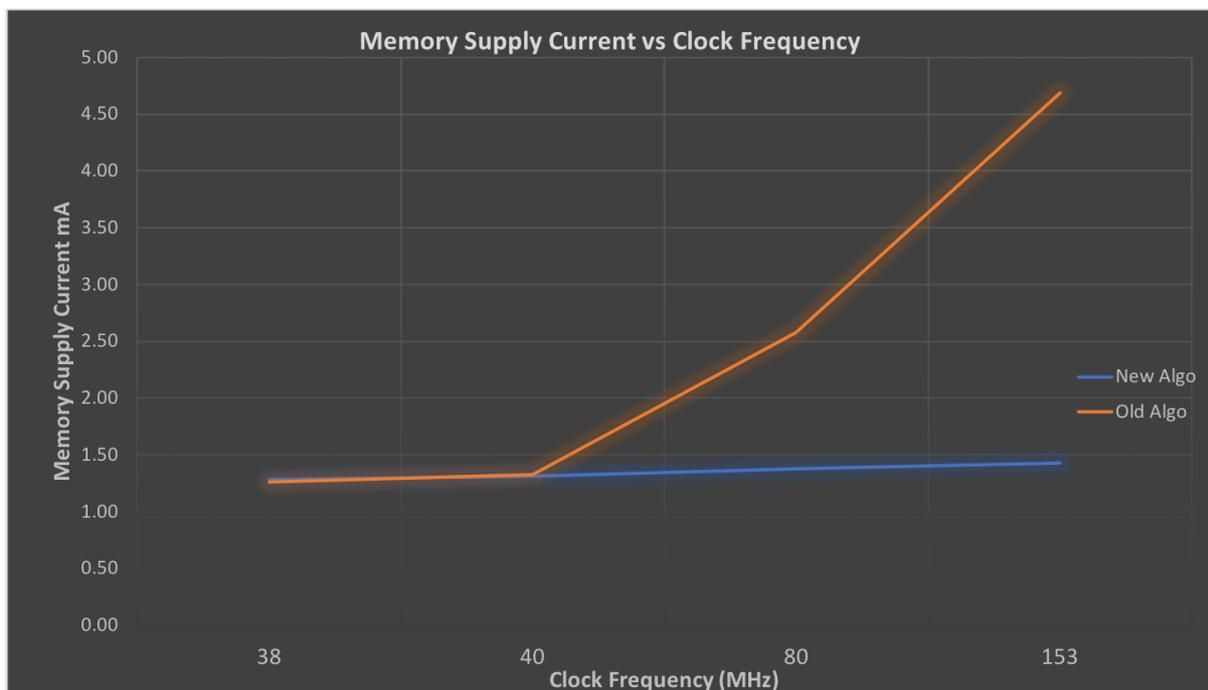
Figure 10: Current on the memory lane versus the Clock Frequency
