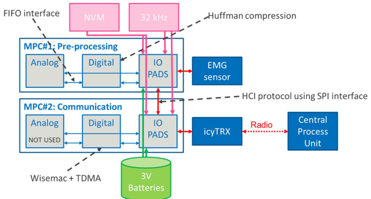
Figure 2 - Structure of the MPC node for the DeTOP project
