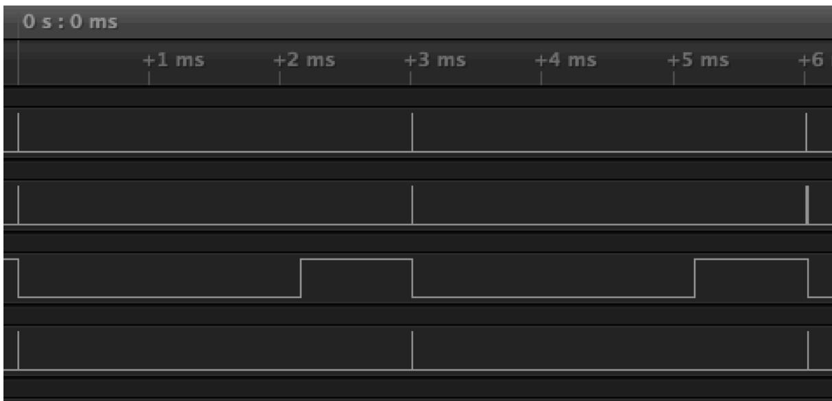
Figure 16: Timing of the software with a clock frequency of 38 MHz
