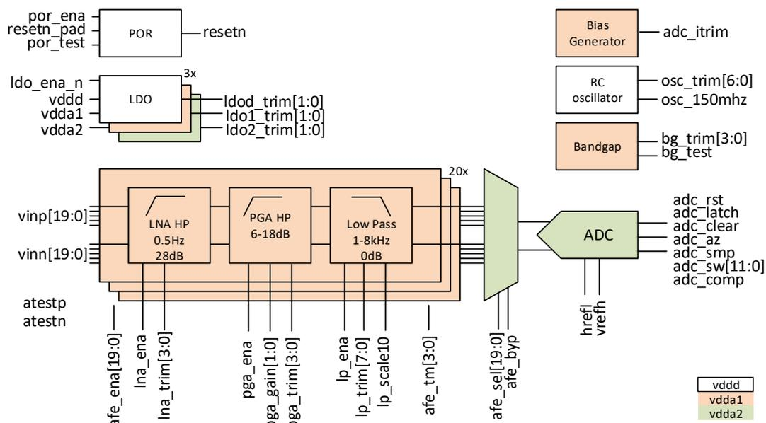
Figure 6: DeTOP Analog top-level block
