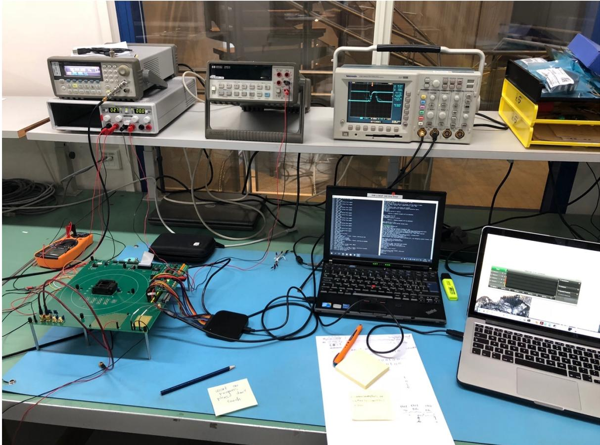
Figure 18: Instrumentation for the characterization of the DeTOP chip mounded on the first revision of the testing board.
