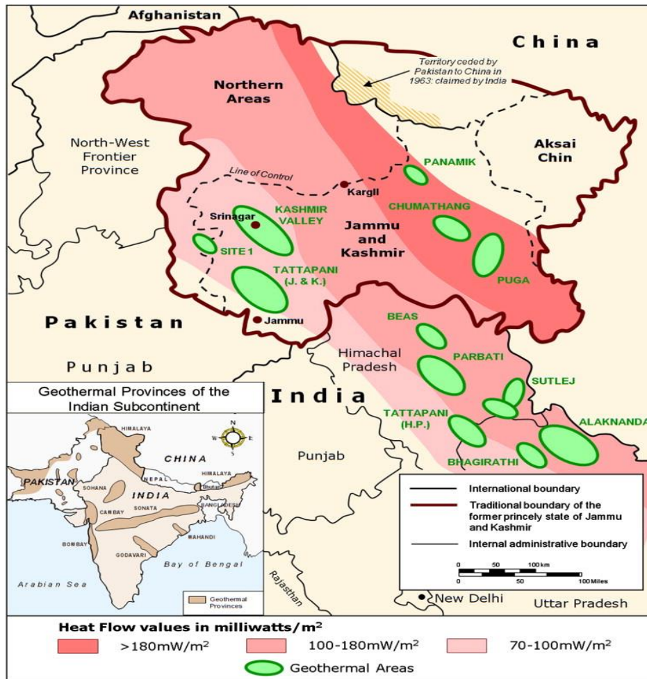
Figure 5-3 Heat flow values of potential Geothermal areas in North
