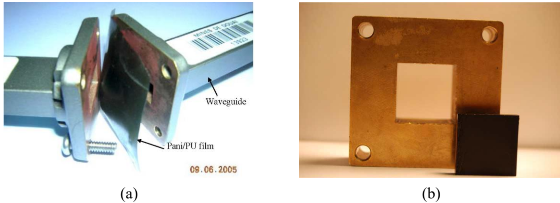
Figure 2.19: Example of a specimen (Pani/PU film) inserted between two waveguide flanges [27] (a); A MWGNP sample (black parallelepiped) cut to fit a waveguide spacer [33] (b).
