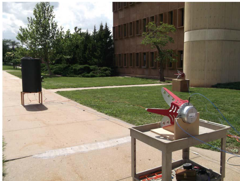
Figure 2.24: Carbon-fiber reverberation chamber in shielding effectiveness measurement configuration [38].
