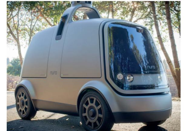
Nuro solve problem of local commerce with last-mile delivery of consumer products, groceries, and hot food from local stores and restaurants. With its specially designed size, weight, pedestrian-protecting front end, operating speed, electric propulsion, and cautious driving habits. It has been put in commerce in 2018. It can load more than 100kg.
