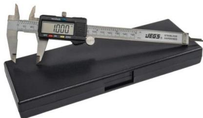
*Figure 8: A digital caliper*
