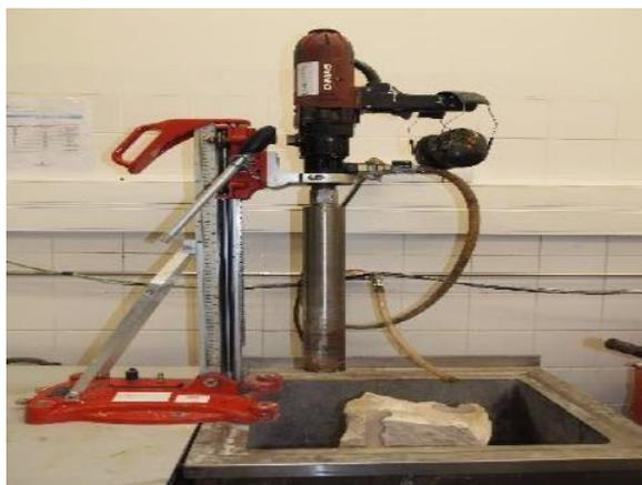
**Figure 5: The Core drill**
