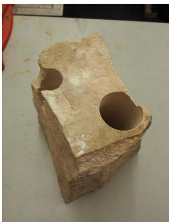
**Figure 6:Matrix From Which Core Plugs are Drilled From**
