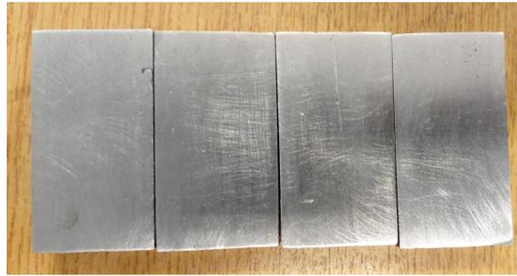
Figure 3.25: DD11 substrates after surface cleaning and preparation.
