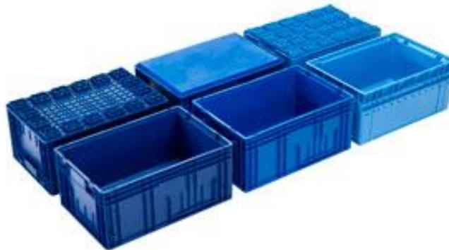
Figure 2. 1. KLT according to recommendations VDA 4500. From left: R-KLT with partially grooved floor, RL-KLT with smooth floor, C-KLT with grooved floor and double reinforced wall (web source: utzgroup.ch).
