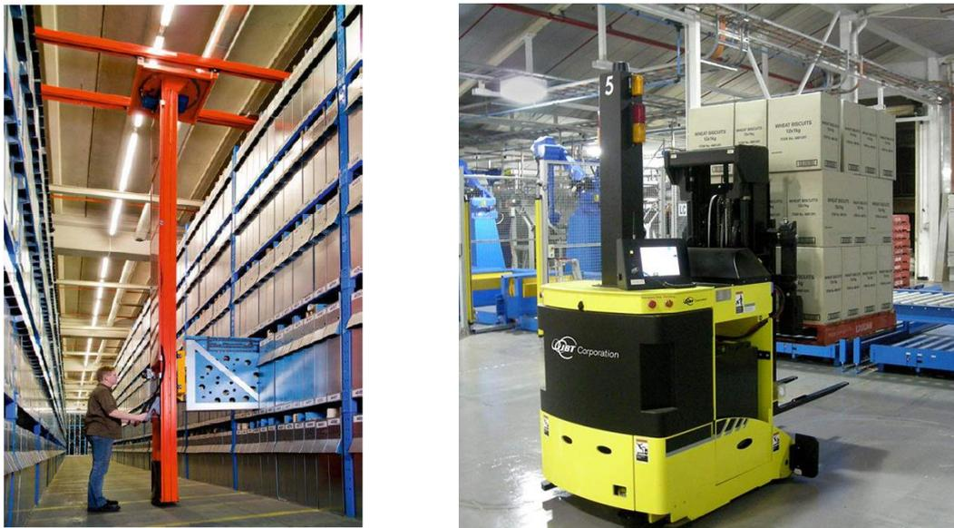
Figure 2. 2: examples of automated systems for storage of medium sized loads in pallet racking. Left: stacker crane (Martin 2016). Right: automatic guided forklift (AGV market insights 2019)
