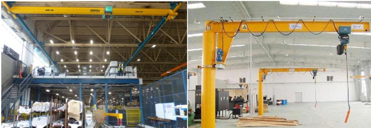
Figure 2. 3. Left: overhead crane with one girder and rope hoist stores material in a mezzanine. Right: Jib crane with chain hoist and motorised column (source: Pelloby Cranes)
