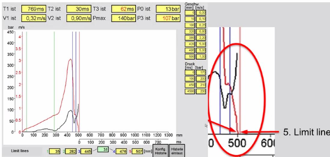
Figure 81: Focus on limit line 5 position
