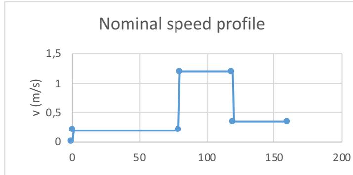
Figure 73: Example of casting speed in function of plunger displacement
