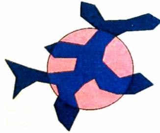
Figure 46: Equivalent diameter (diameter of a circle of equal area) [ $\varnothing_F$ ]
