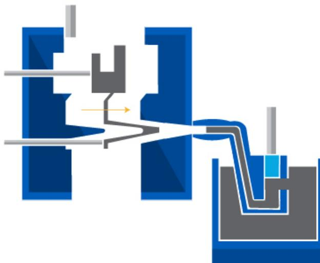
*Figure 18: Casted component ejection at the end of the casting process*
