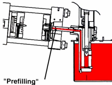
Figure 85: Molten metal (represented in red) at prefilling end, before die filling start.
