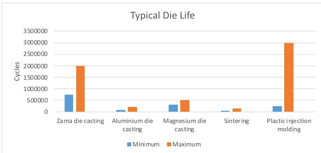
Figure 9: Die life diagram to compare different materials
