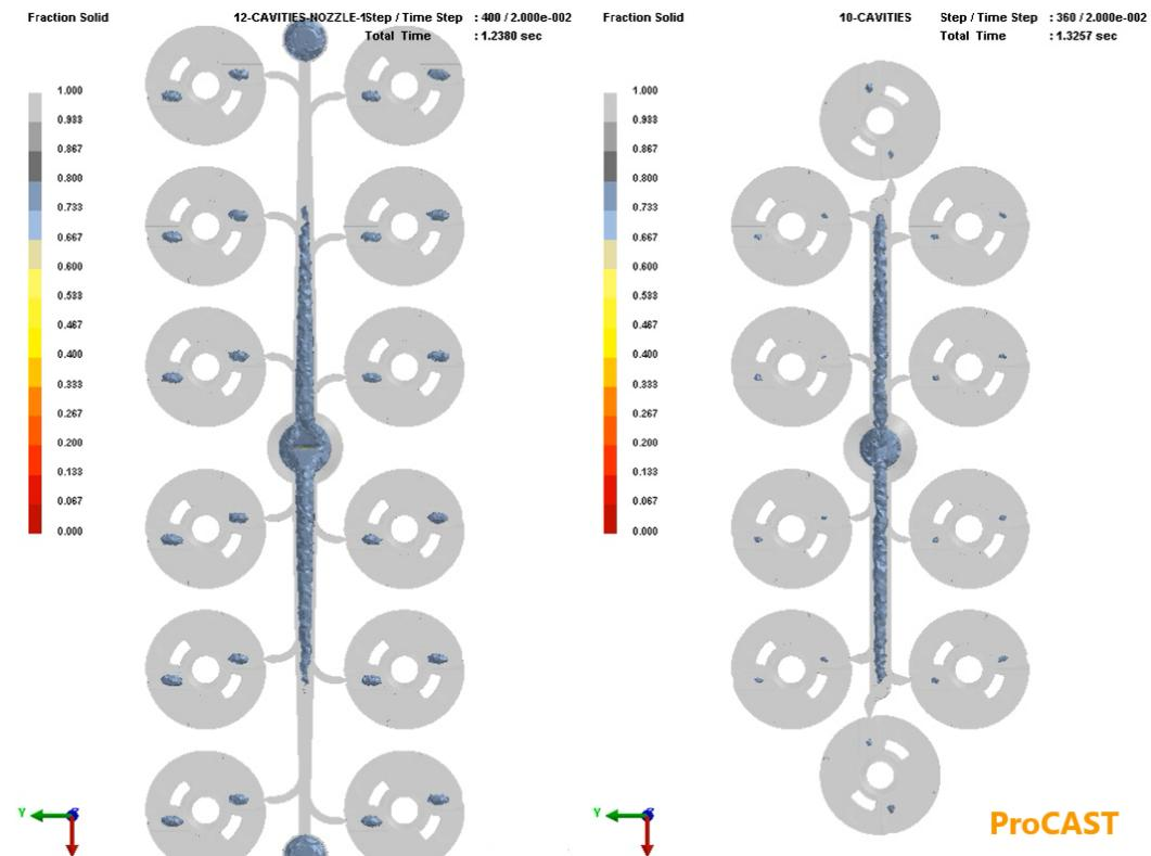
Figure 56: Representation of the end of solidification
