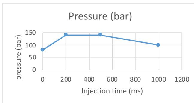
Figure 64: Representation of casting pressure in function of time (milliseconds) from piston start
