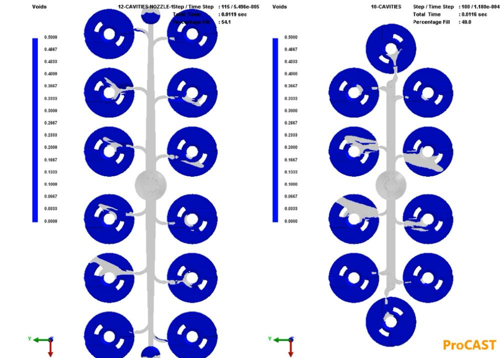
Figure 50: Representation of die filling initial phase
