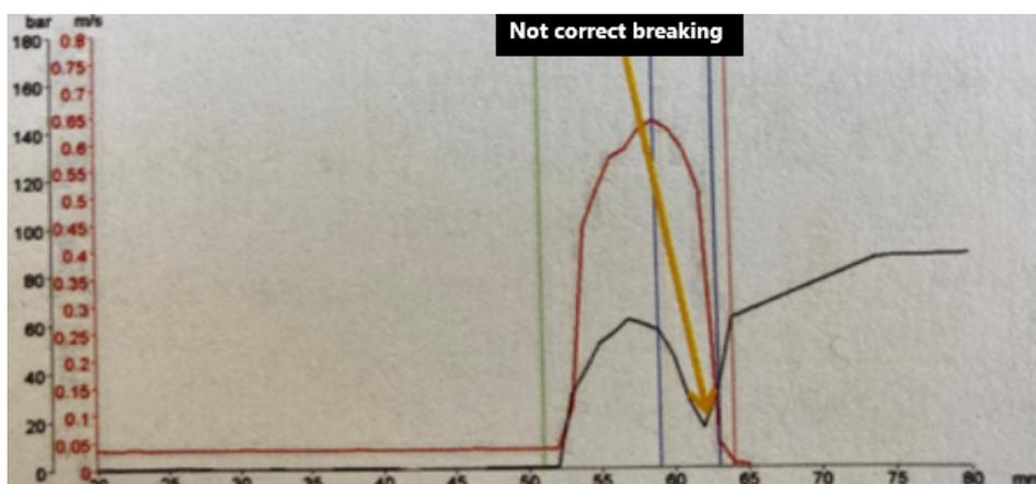
Figure 83: Incorrect braking (the black curve indicates the pressure)
