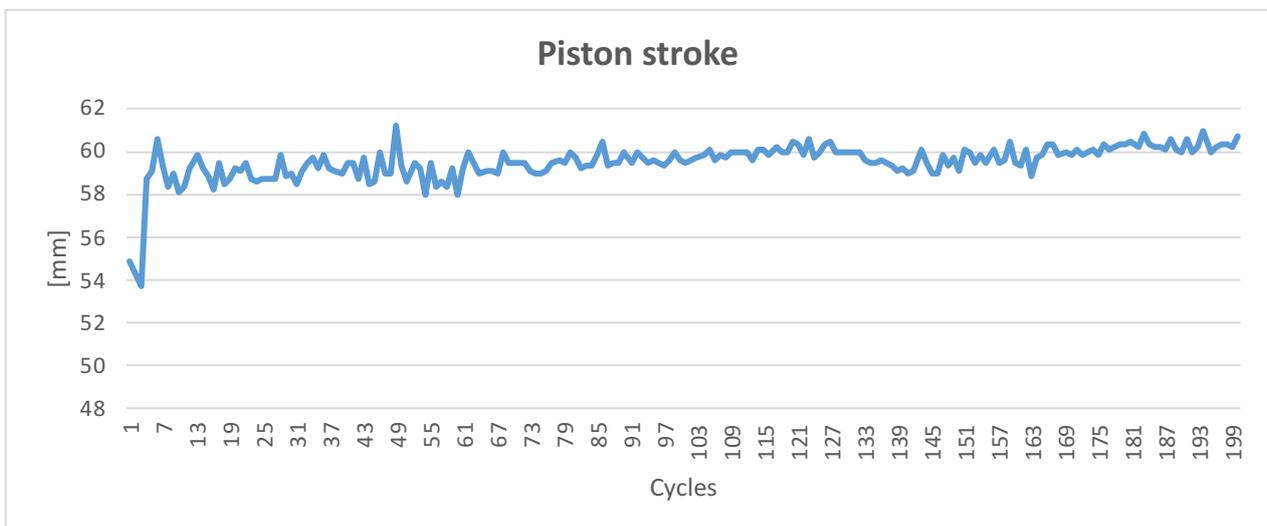
Figure 27: Piston stroke
