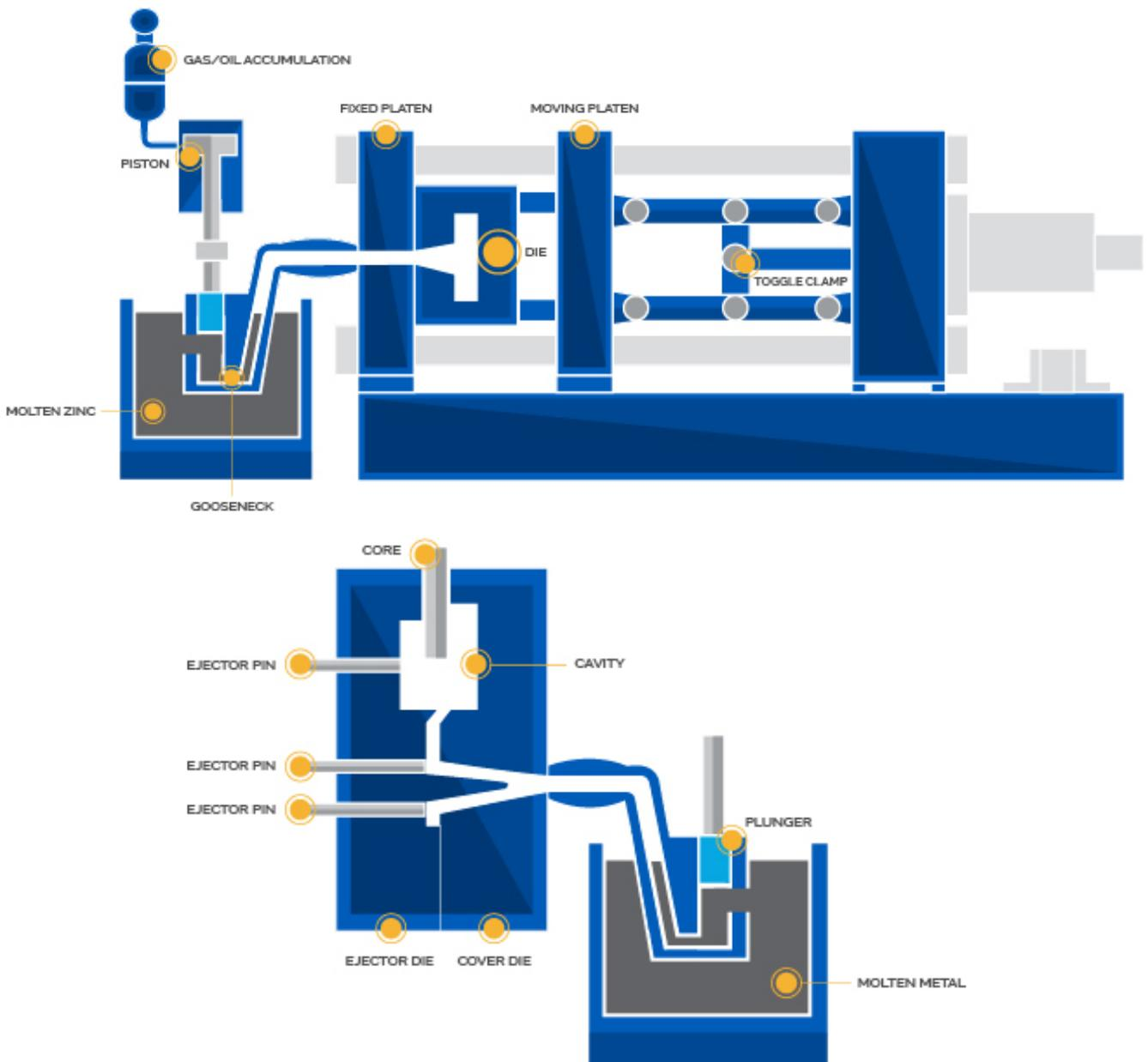
Figure 16: Hot chamber die casting machine metal injection system
