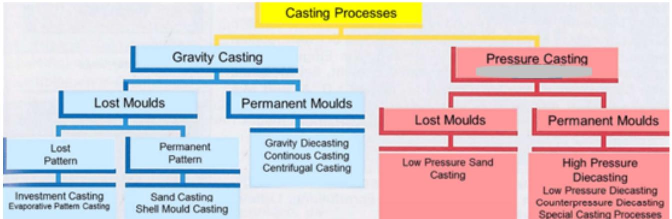
Figure 8: Casting processes – Gravity casting and pressure casting
