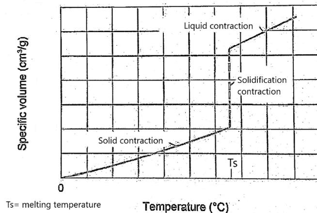
Figure 41: Specific volume in function of temperature
