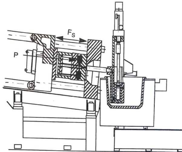
Locking force of a diecasting machine  $F_{zu} = \text{casting force } F_s \times \text{safety factor } f (1.3 - 1.6)$
