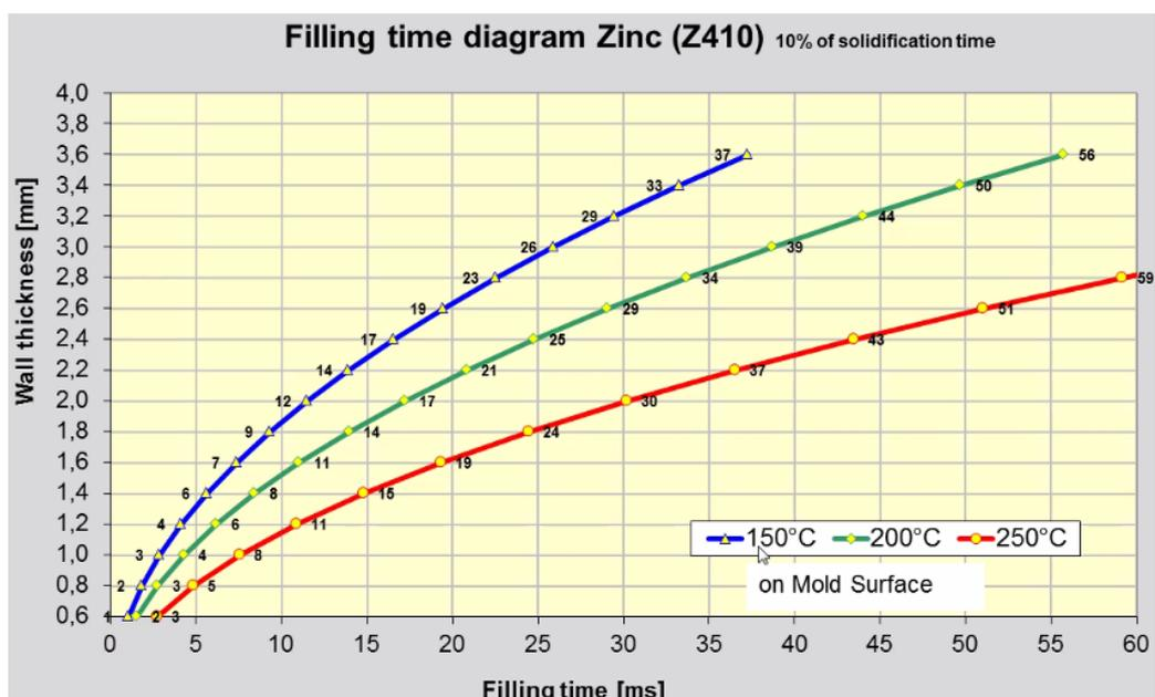
Figure 53: Filling time diagram of a Zama alloy
