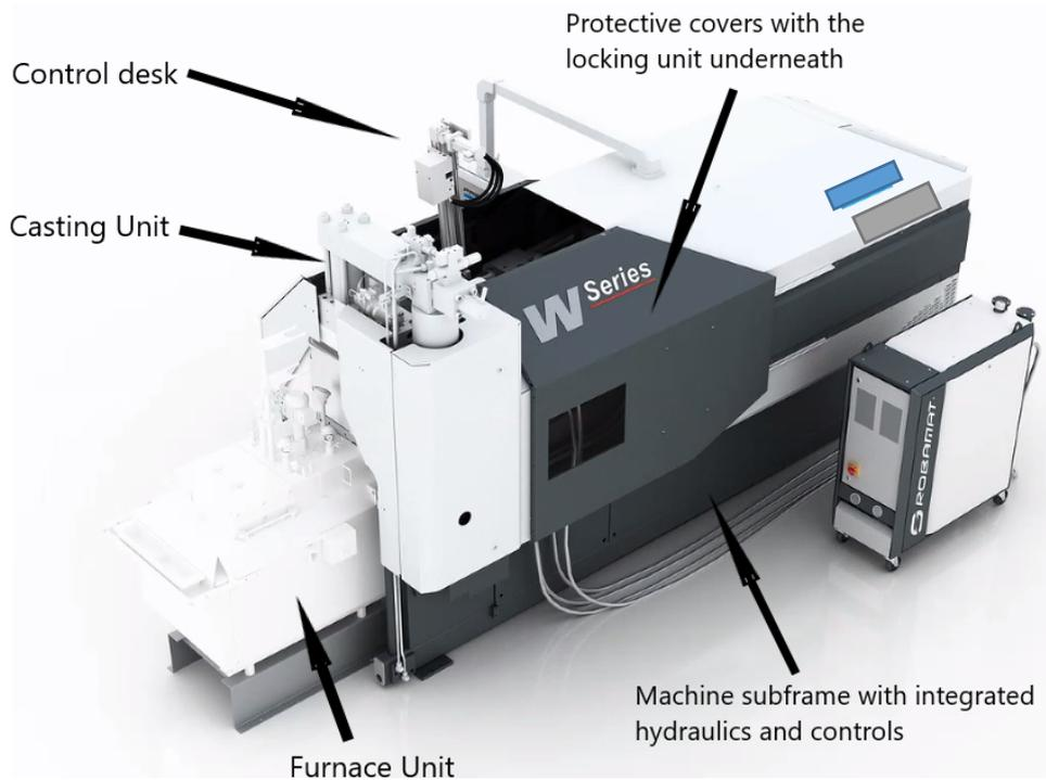
Figure 19: Schematic representation of hot chamber die casting machine main parts
