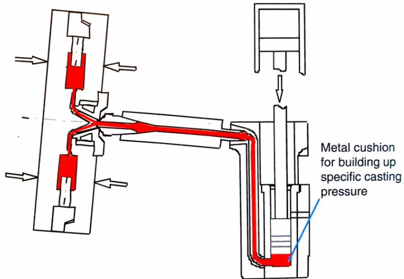
Figure 67: injected metal path in the casting unit
