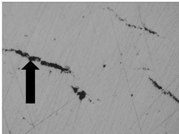
Figure 42: Shrinkage cavities on a component
