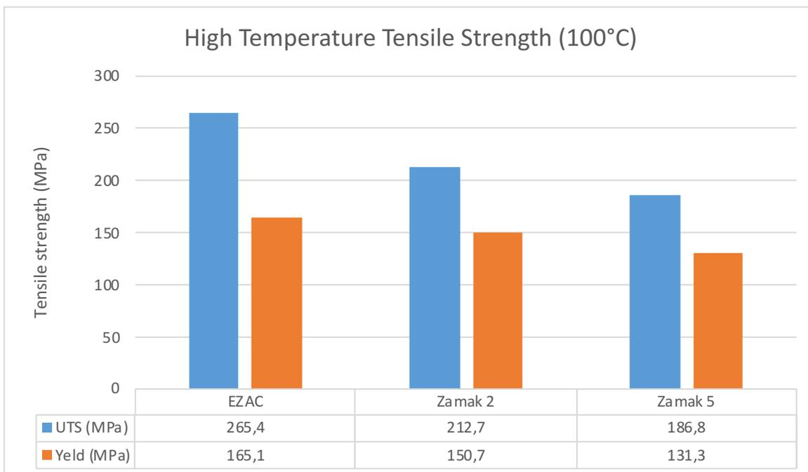
*Figure 1:* High temperature tensile strength diagram for zinc alloys
