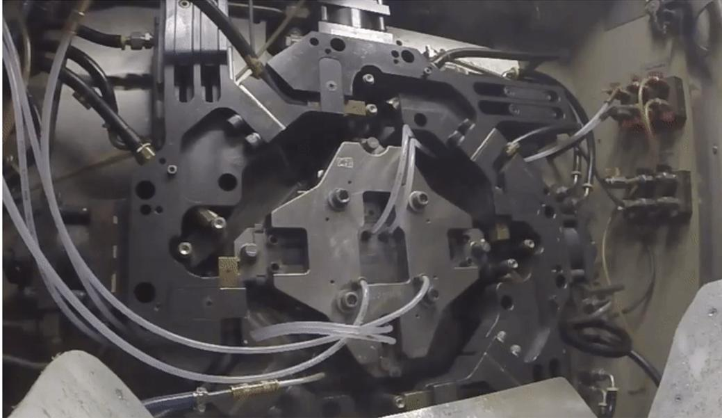
*Figure 26: Multi-slide die casting machine*
