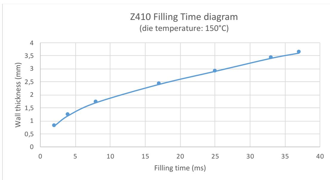
Figure 76: Die filling time of a Zama alloy in function of component wall thickness
