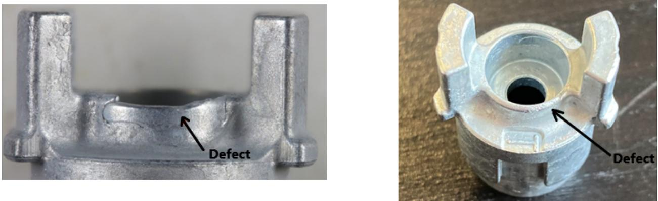
*Figure 87: Visible defect on the part*
