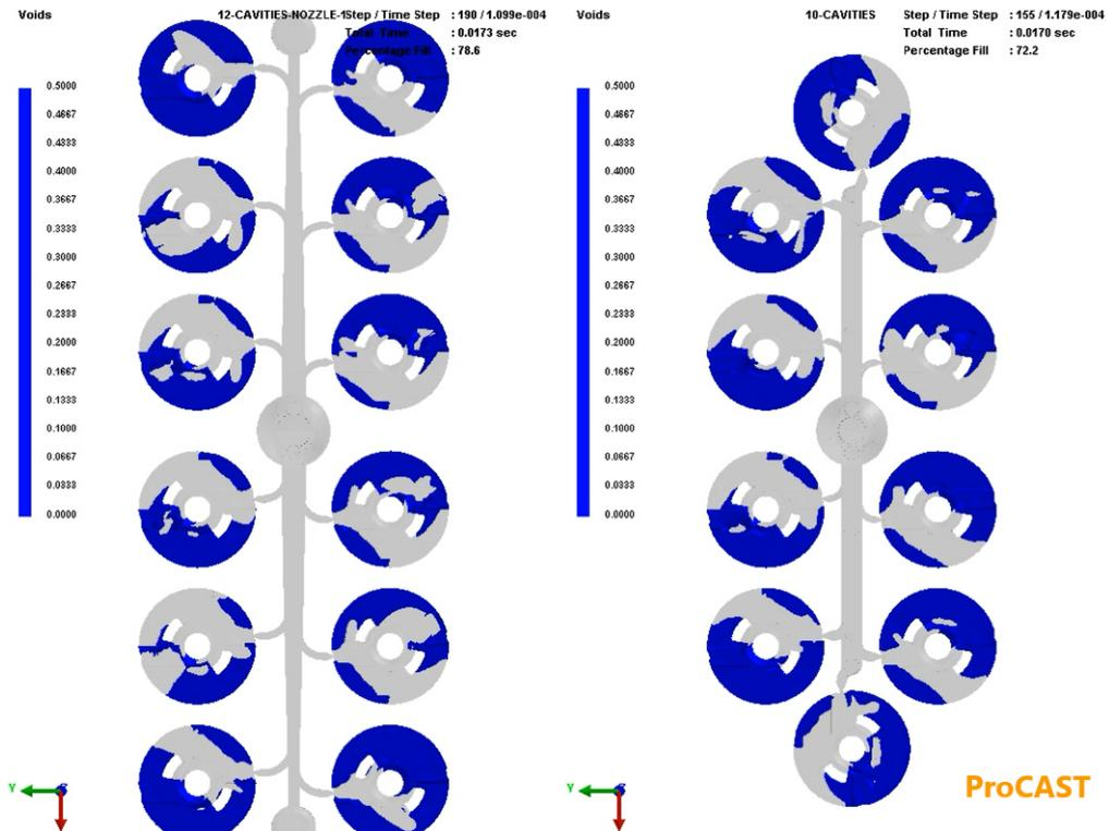
Figure 51: Representation of die filling intermediate phase
