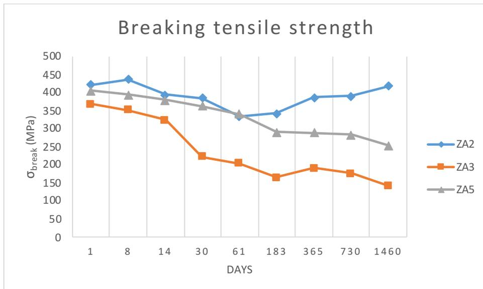
Figure 6: Zama alloys breaking tensile strength of air cooled specimens aged until 4 years
