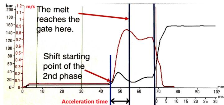
Figure 79: Second phase shift starting point
