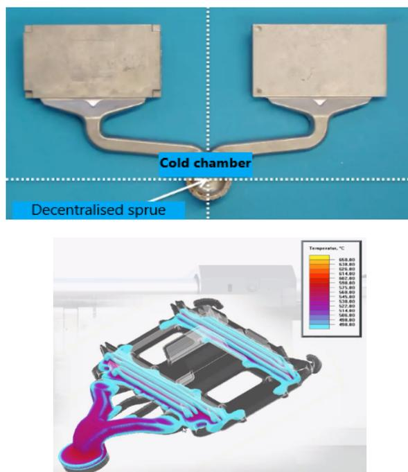
Figure 22: Illustrative images - Typical mould cavities configuration in cold chamber die casting process
