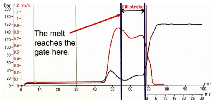
Figure 78: Graphical filling stroke representation
