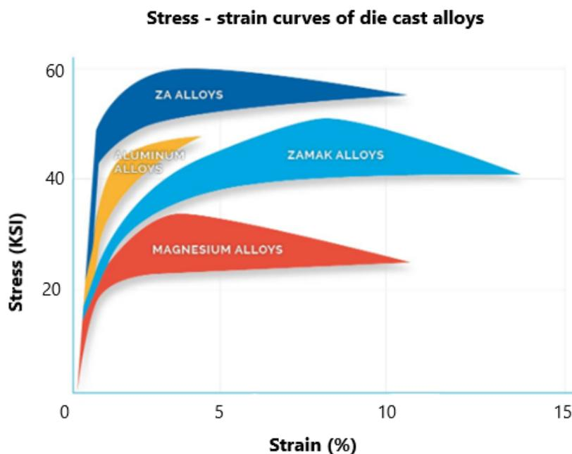
Figure 3: Stress and strain curves of die cast alloys [5]
