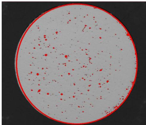
*Figure 43: Pores in the circular section of a sample*
