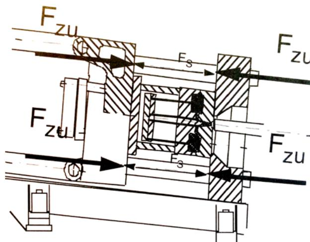
Figure 70: Schematic representations of forces acting in a casting unit
