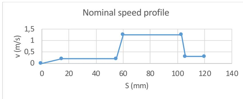
Figure 63: Representation of casting speed in function of plunger movement
