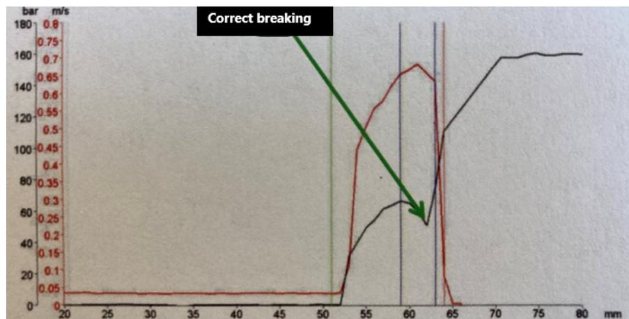
Figure 82: Correct braking (the black curve indicates the pressure)
