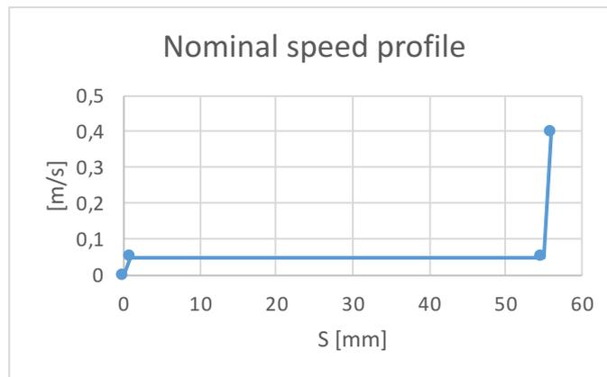
Figure 74: Casting speed in function of plunger displacement with focus on prefilling velocity
