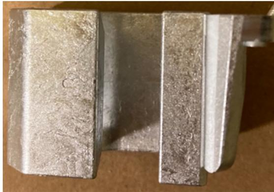
*Figure 37: flow marks defect*
