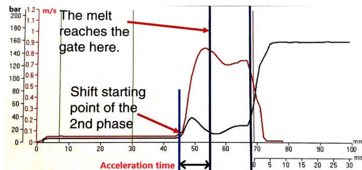
Figure 79: Second phase shift starting point
