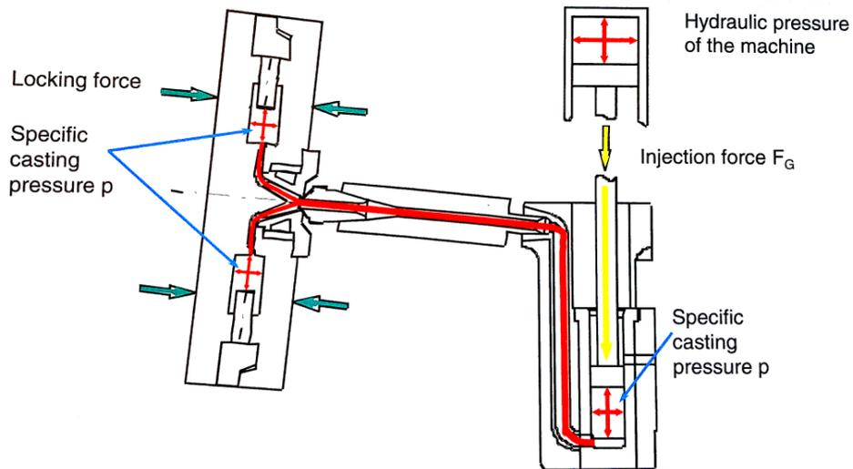
Figure 68: Casting unit representation with focus on pressures
