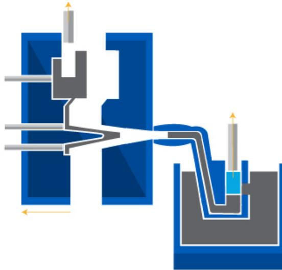
*Figure 17: Die opening phase in the casting process*
