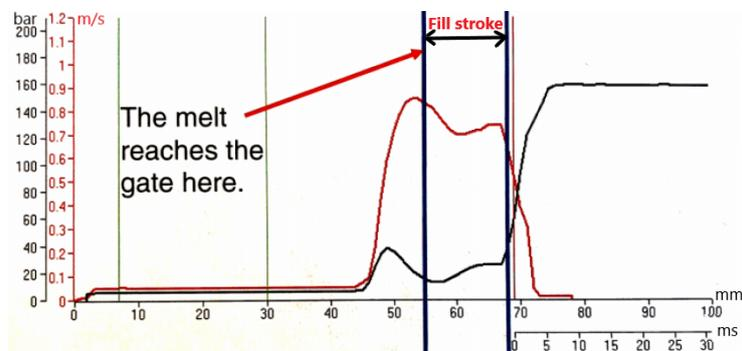
Figure 78: Graphical filling stroke representation
