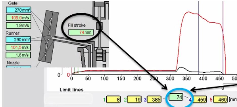
Figure 80: Casting curve, fill stroke and limit lines
