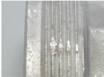
*Figure 40: Dents on a cast part*
