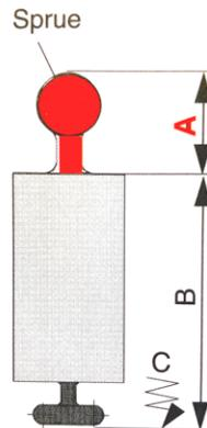
Figure 72: Representation of the filling level reached in the 1<sup>st</sup> phase, indicated with letter "A"
