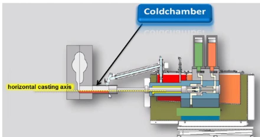
*Figure 15:* Cold chamber machines configuration
