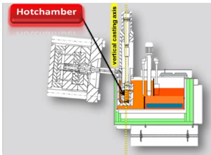
Figure 14: Hot chamber machines configuration
