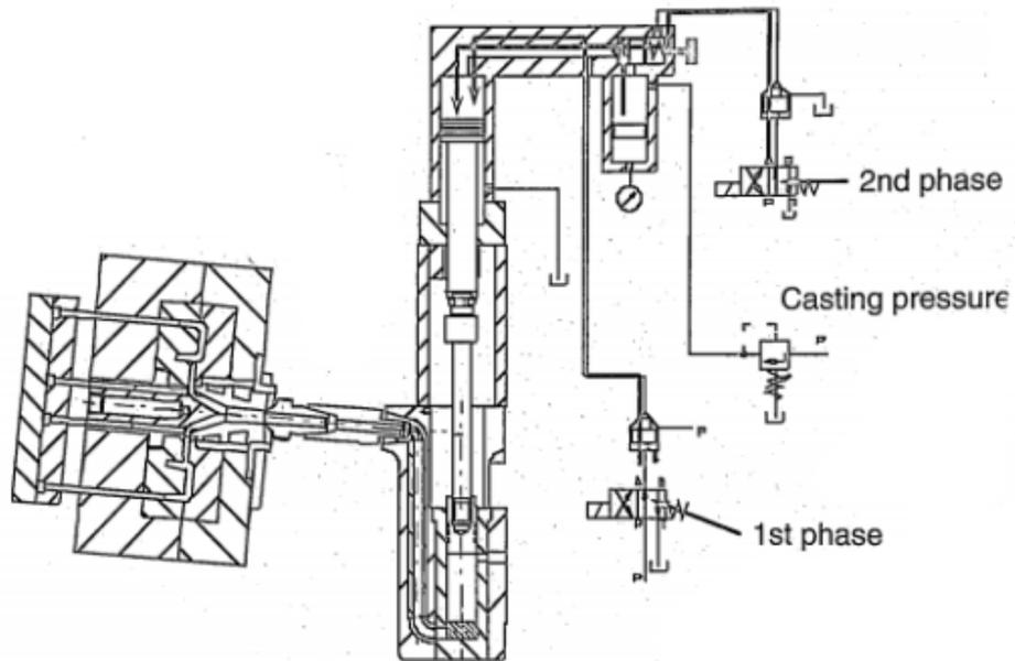
Figure 60: Schematic representation of Standard casting unit functioning
