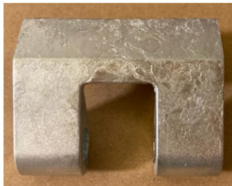
*Figure 38: cold flow defect*
