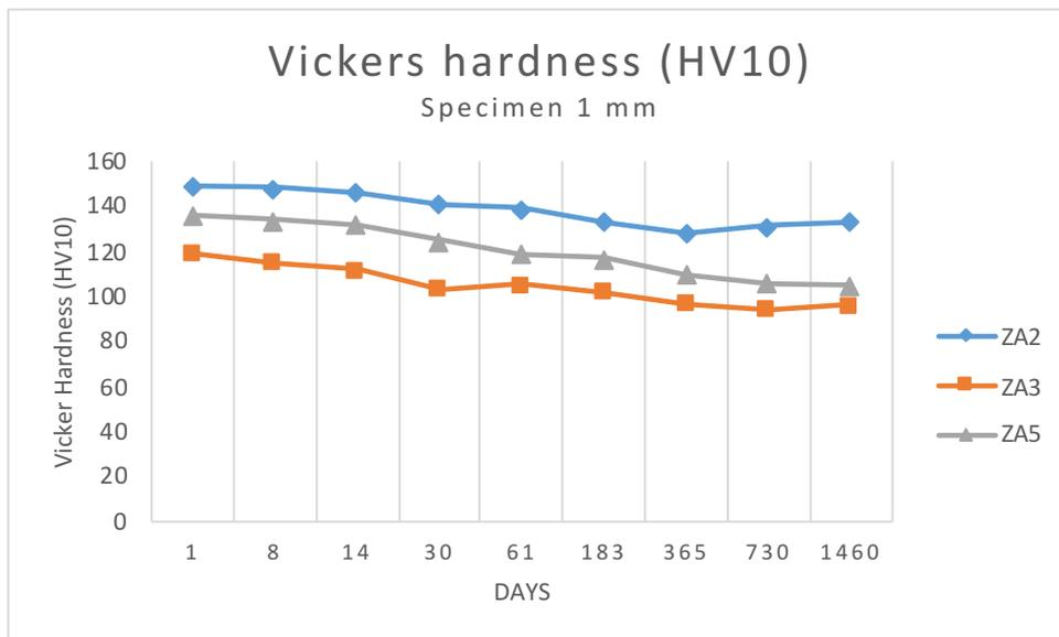
*Figure 7:* Diagram of Zama alloys Vickers Hardness in function of ageing time of air cooled specimens
