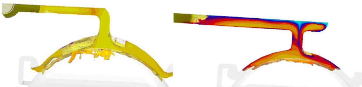
Figure 57: Asymmetrical filling without damper (left) and symmetrical filling with damper (right)
