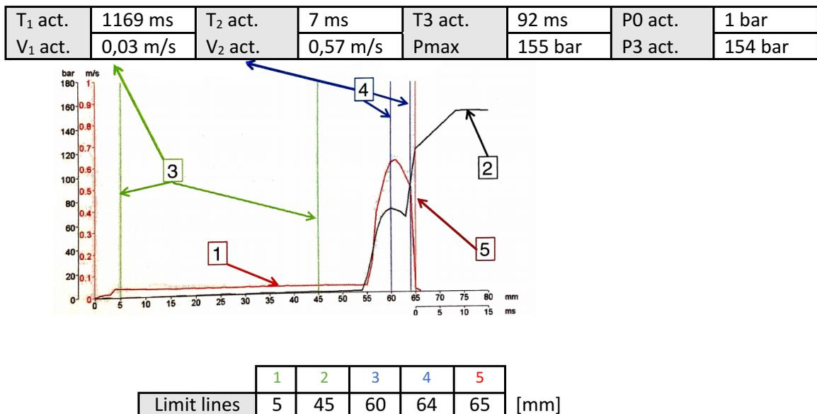
Figure 77: Representation of casting limit lines
