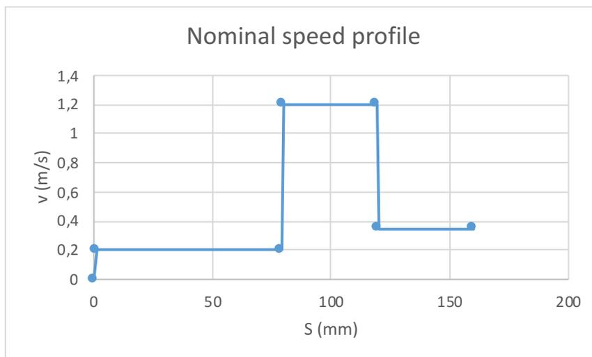
Figure 62: Representation of casting speed in function of plunger movement
