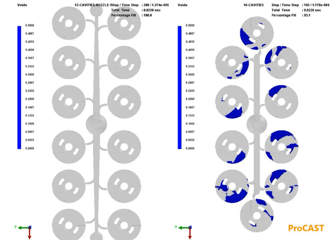
Figure 52: Representation of the end of die filling phase
