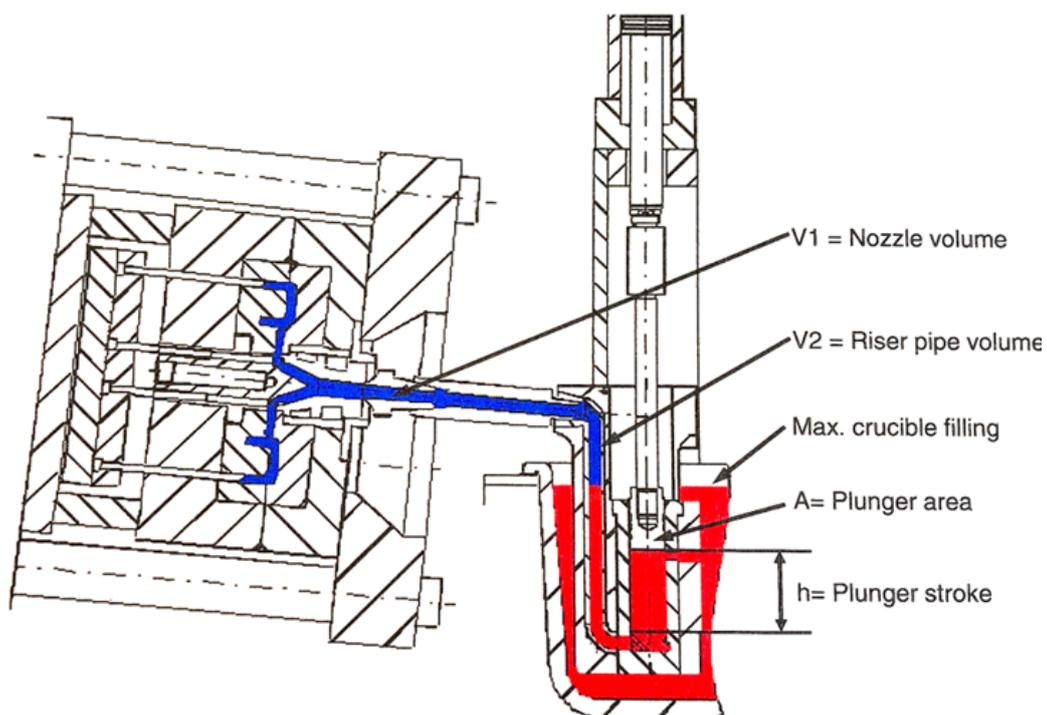
Figure 66: Casting unit schematic representation
