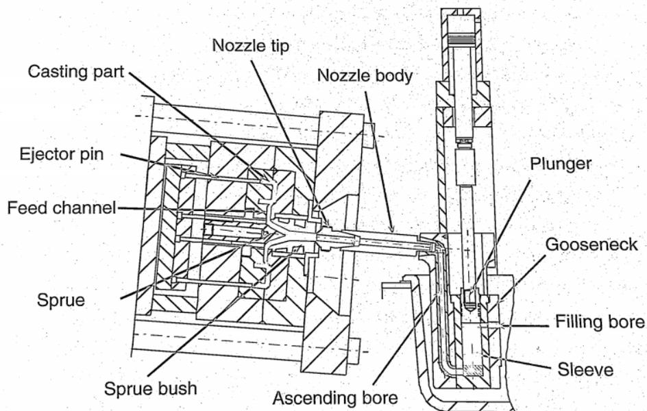
Figure 59: Standard casting unit representation
