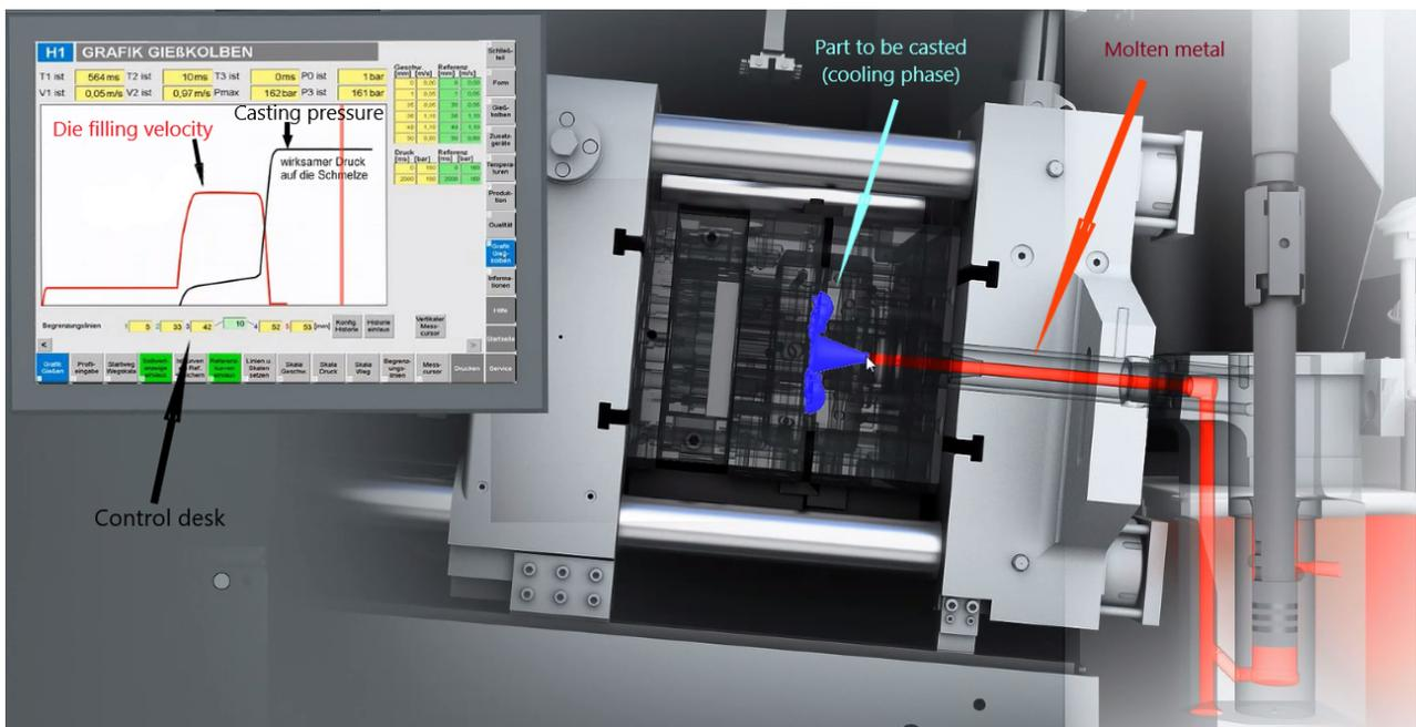
Figure 20: Internal view of the casting unit of an hot chamber die casting machine
