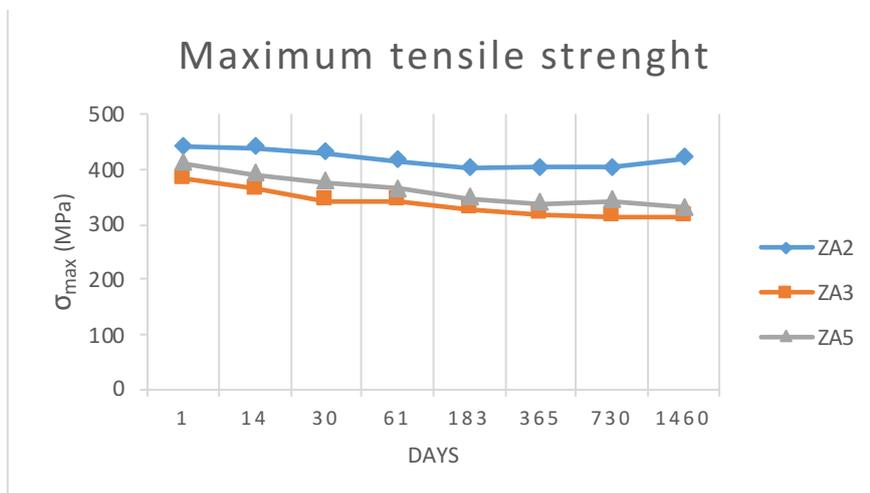
Figure 4: Zinc alloys maximum tensile strength in function of ageing time
