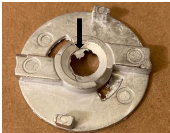
*Figure 35: flash defect*
