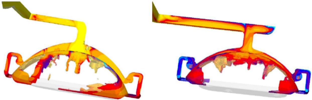
Figure 58: Divergent feeder (left side) and convergent feeder (right side)
