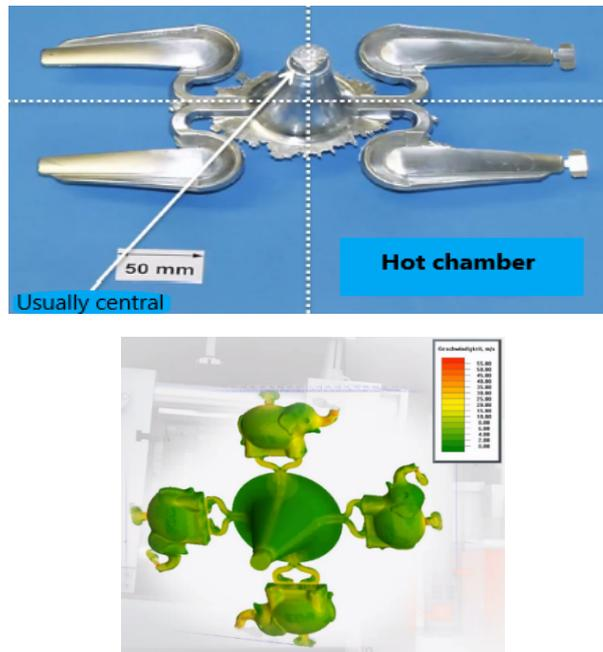
Figure 21: Illustrative images - Typical mould cavities configuration in hot chamber die casting process
