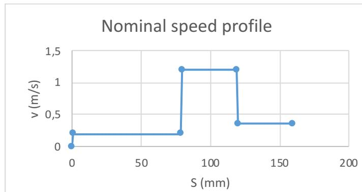
Figure 75: Representation of casting speed in function of plunger displacement
