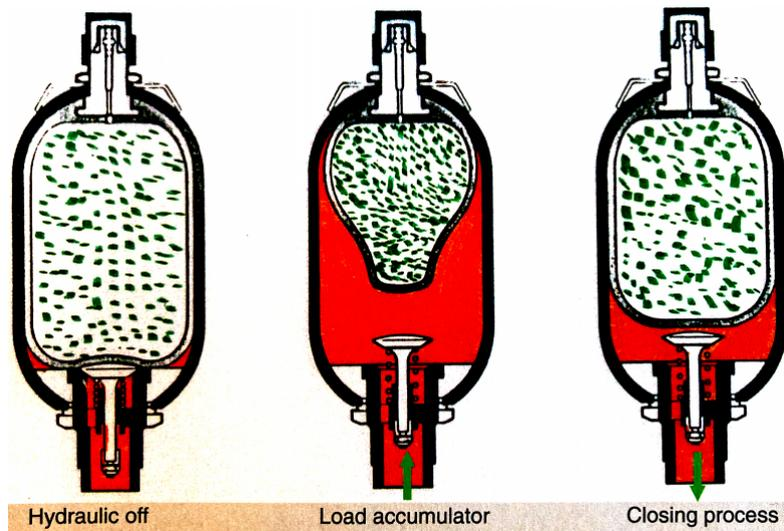
Figure 71: Representation of N<sub>2</sub> pressure in bladder accumulator
