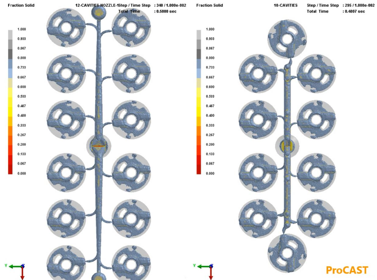
Figure 54: Representation of the first stage of solidification
