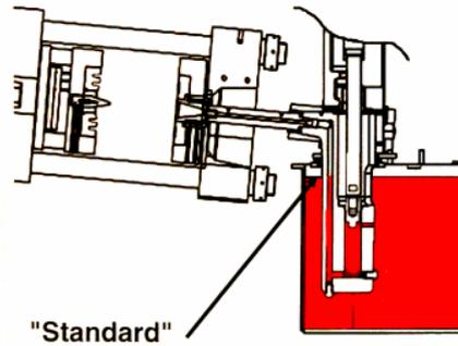
Figure 84: Standard filling system, in which molten metal is represented in red
