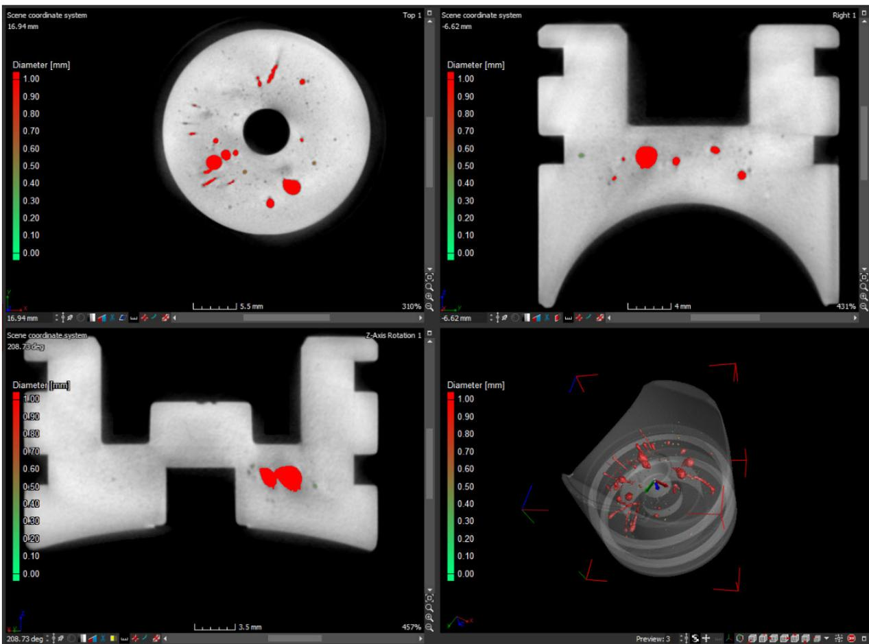
Figure 44: Pores on Zama casted component detected with a tomography
