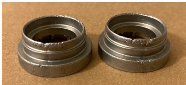
*Figure 34: Not completely filled parts*
