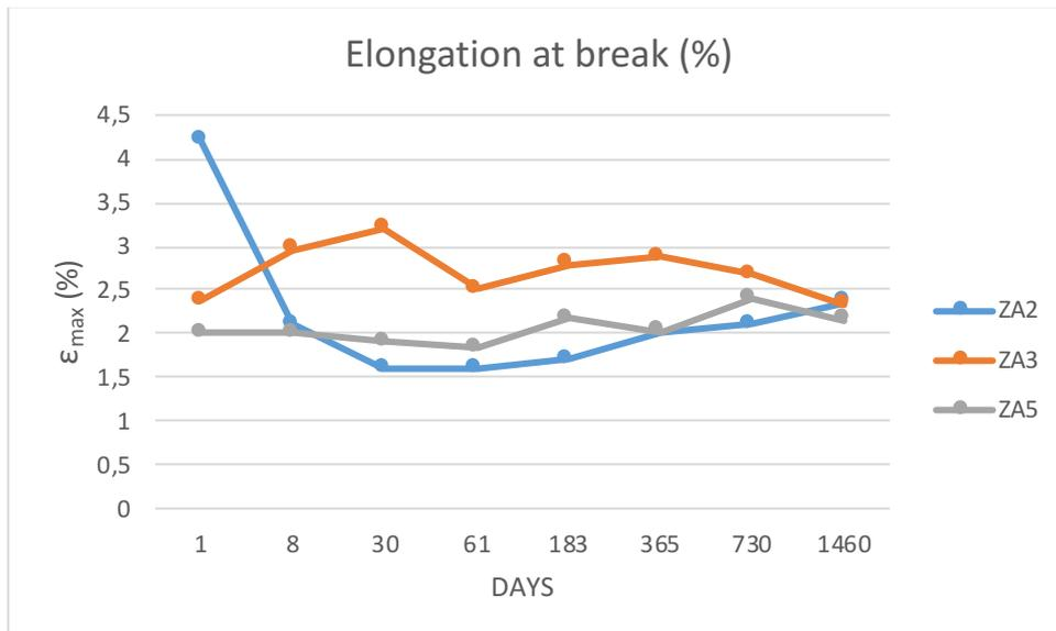
Figure 5: Diagram of Zinc alloys elongation at break ( $\epsilon_{\max}$ ) in function of ageing time
