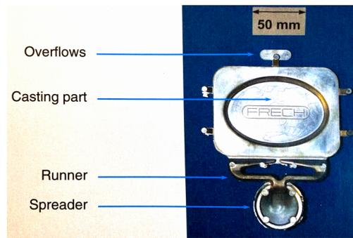
Figure 69: Casting area of a die casted part
