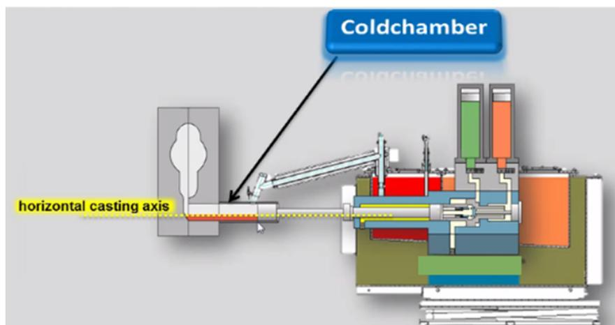
*Figure 15:* Cold chamber machines configuration
