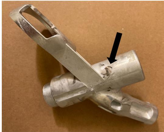
*Figure 36: Surface deposits on the component*
