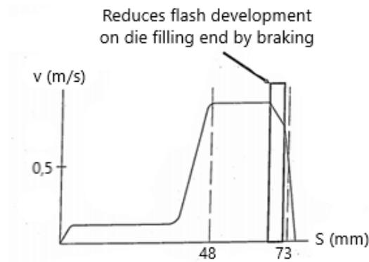
Figure 61: Representation of braking at the end of die filling
