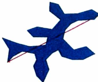
Figure 47: Pore length or analogy diameter [ $\varnothing_L$ ]
