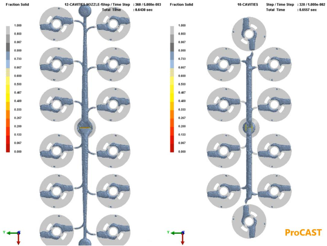
Figure 55: Representation of intermediate phase of solidification
