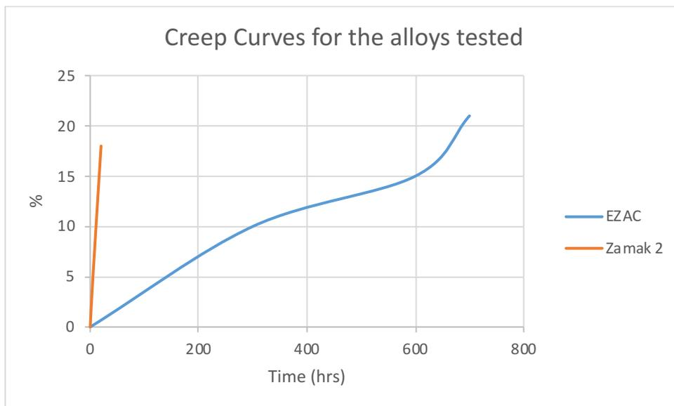
*Figure 2:* Creep curves for the tested Zinc alloys
