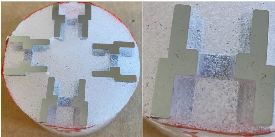
Figure 45: Destructive porosity test on Zama die casted samples
