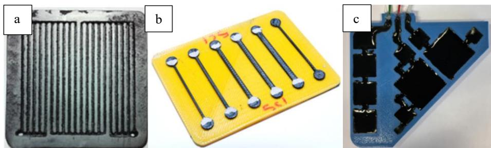
Figure 8 - Examples of AM electronic components. a) Graphite composite bipolar plates for PEM fuel cell fabricated by SLS [13]; b) 3D printed sample of an x-axis expansion testbed [19]; c) A touch pad 3D printed using conductive paint [20].
