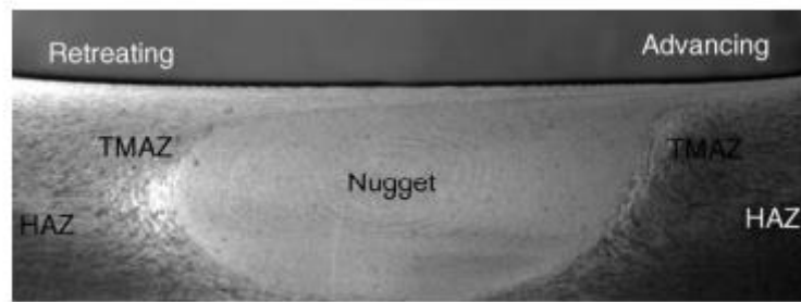
Figure 7 - Microstructural zones of FSW done on 7075Al-T651 aluminium alloy [1].
