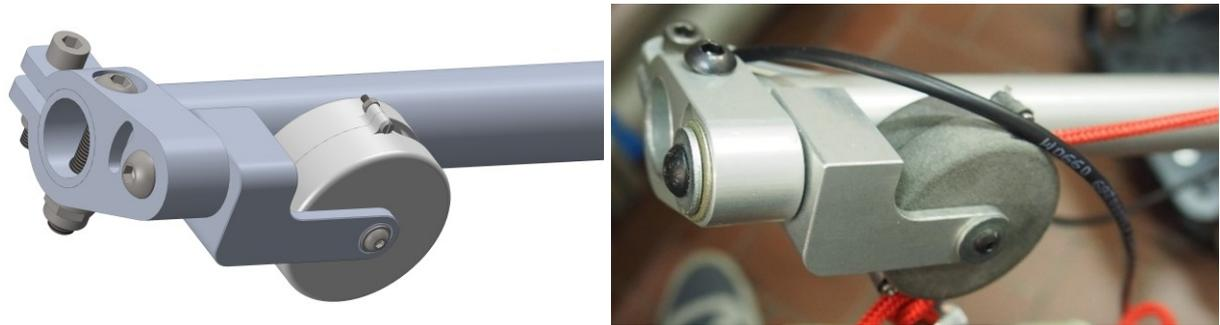
Figura 137: Confronto Handwheelchair.q CONNECTOR RETURN PULLEY SUPPORT ROD
