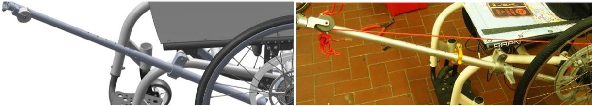
Figura 136: Confronto Handwheelchair.q SUPPORT ROD
