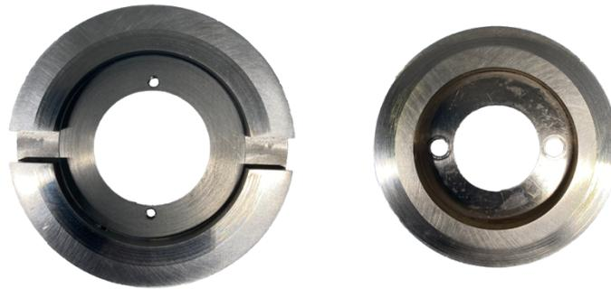
Figure 3.1: Photos of the two sample. The stationary steel disc is on the left and the rotating brass disc is on the right.
