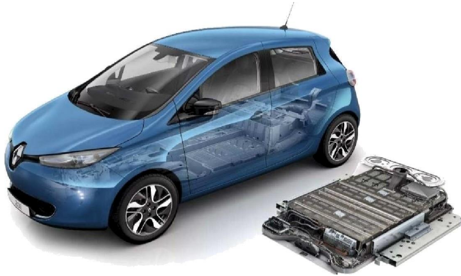
Fig 3.2.1 Renault Zoe R100 Z.E.40 and its battery pack
