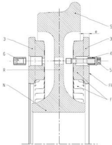
Figure 35 - Disk mounted on Wheel configuration
