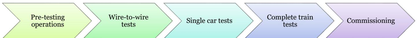
Figure 13 - Testing sequence
