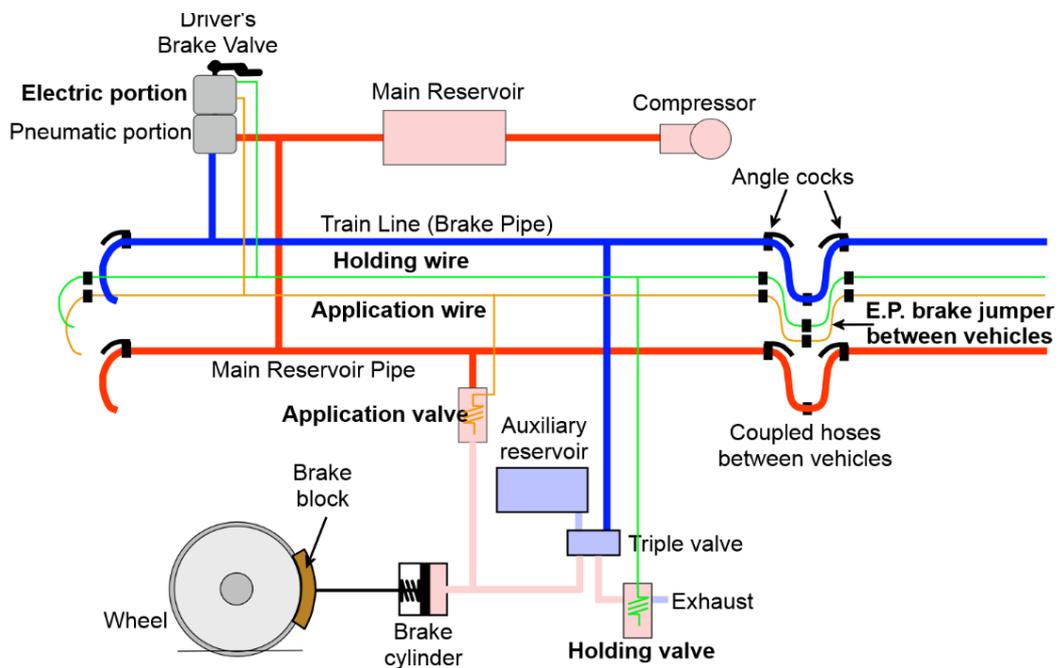
Figure 17 - Schematic for EP brake control
