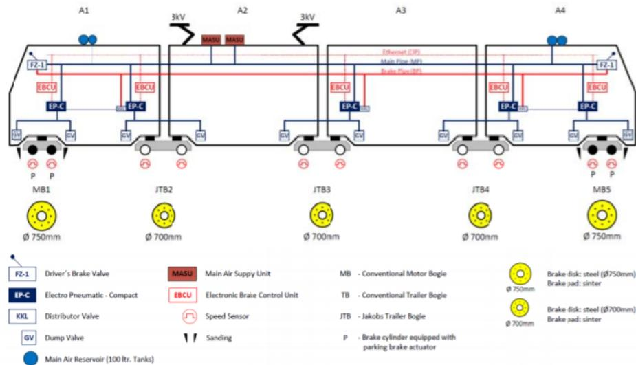
Figure 28 - Braking system Smart Coradia
