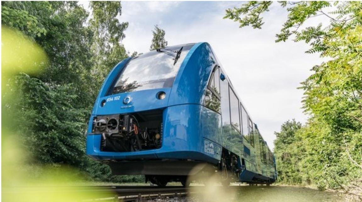
Figure 11 - iLint Hydrogen powered train
