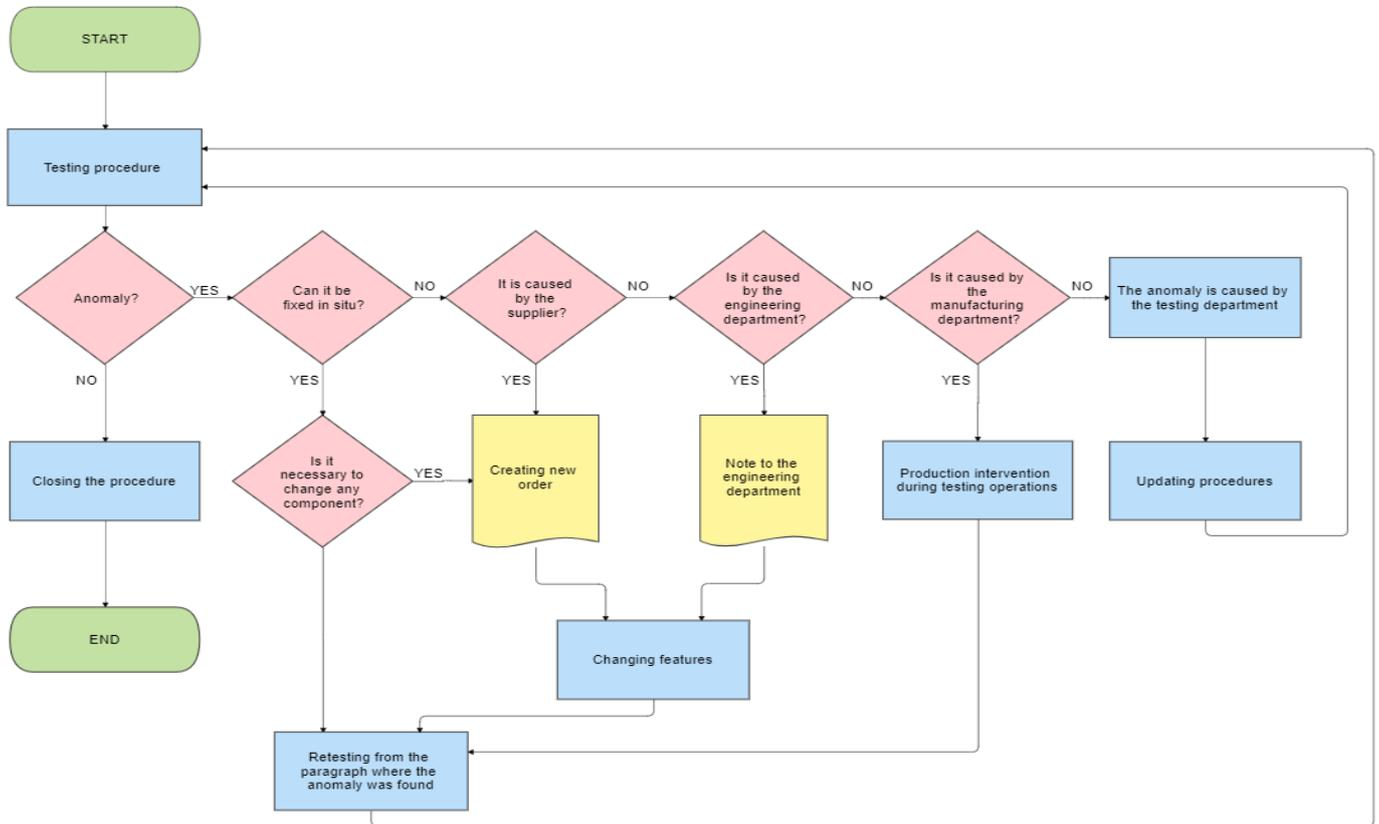
Figure 12 - Flow-chart Testing Operations
