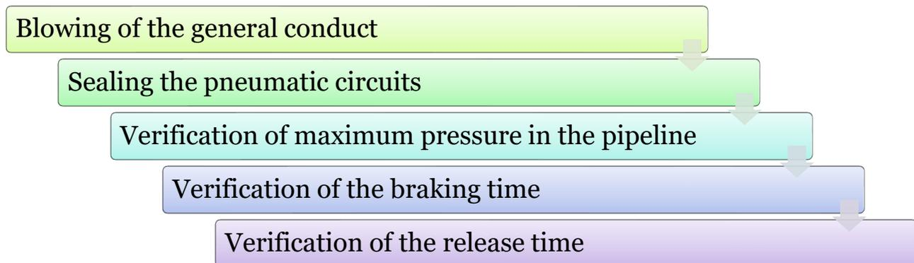
Figure 20 - Example of testing of the EP brake
