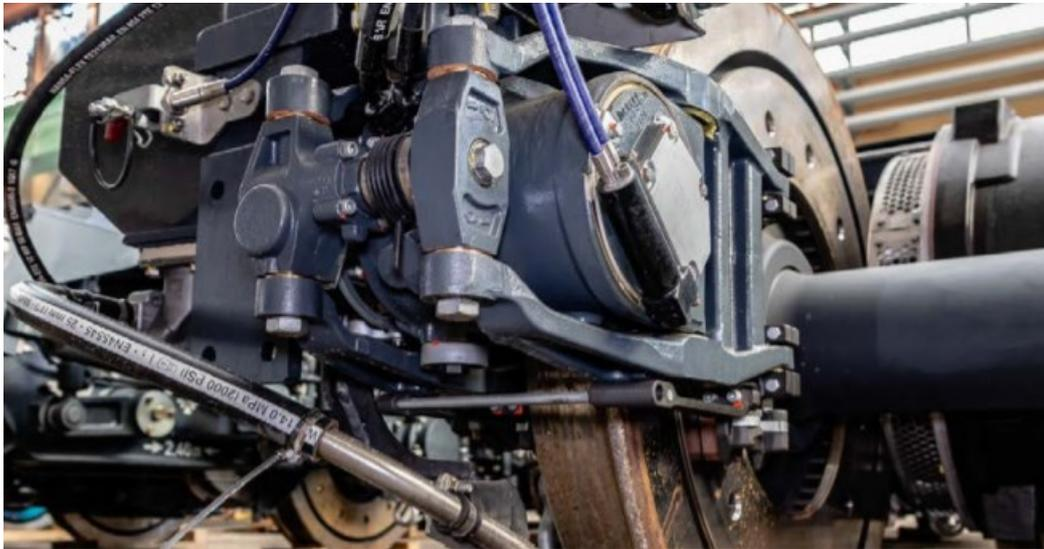
Figure 18 - Parking brake on a train wheelset
