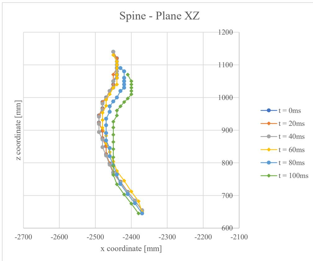
Figure 5.35 - Spine deformation on plane XZ at 0ms, 20ms, 40ms, 60ms, 80ms and 100ms
