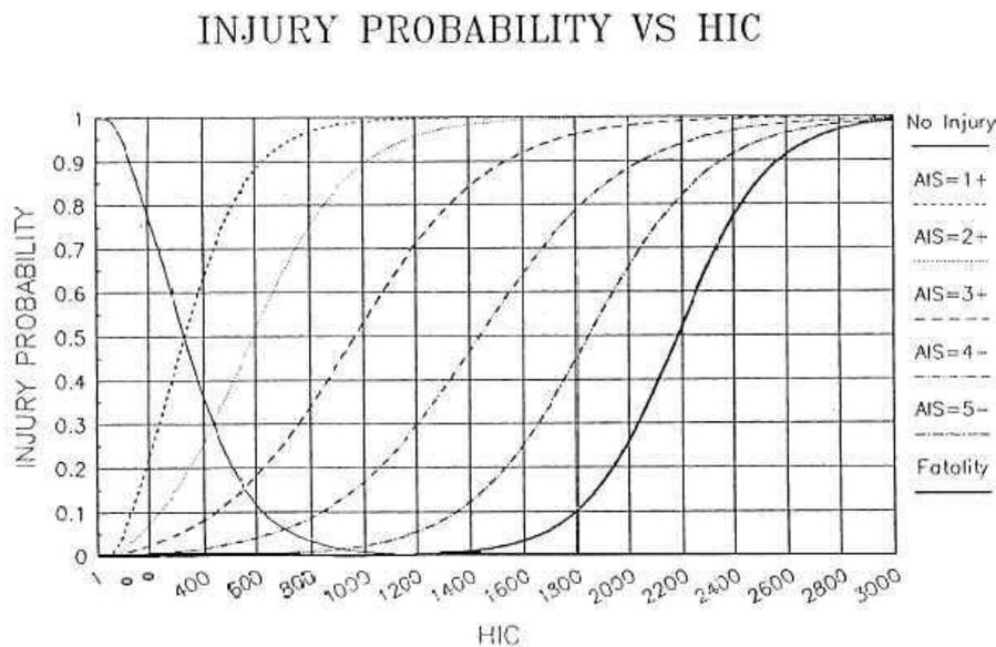
Figure 5.11 - Prasad-Mertz Injury probability vs HIC curve
