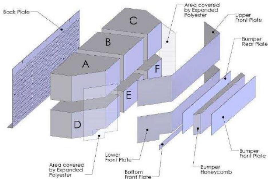
Figure 3.1 - AE-MDB barrier details
