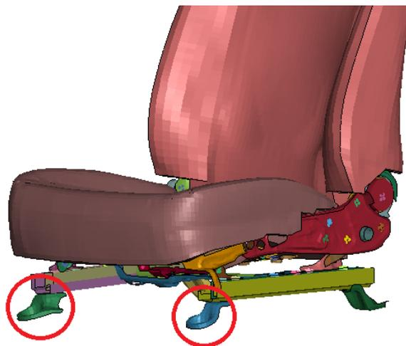
Figure 4.5 - Details of the seat attacks constrained
