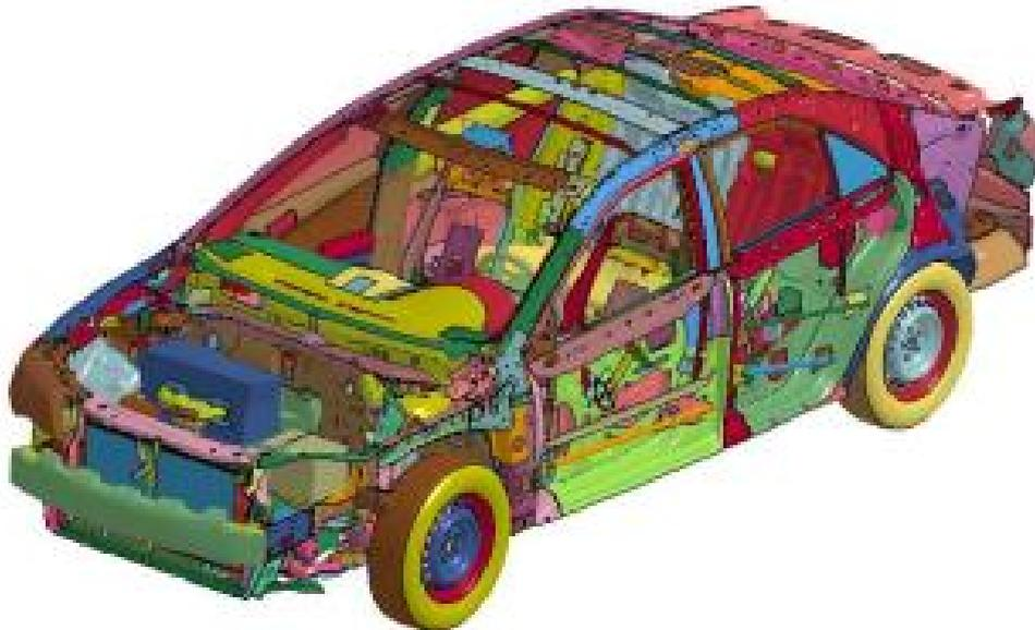
*Figure 3.5 - Detail FE model*
