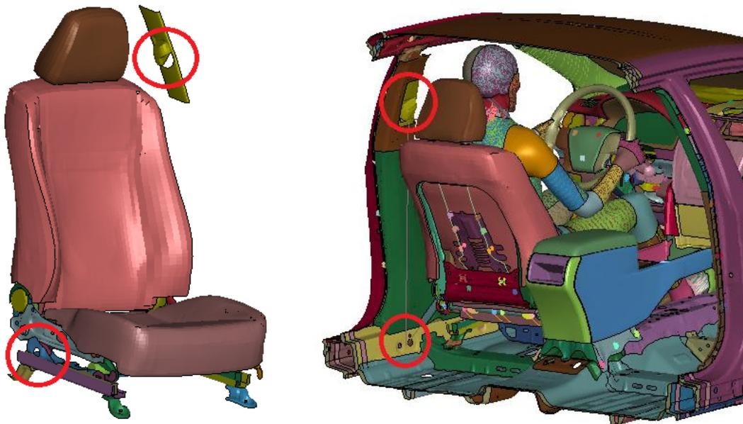
Figure 4.14 - Anchors in the FE model
