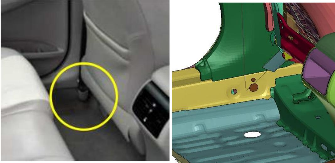
Figure 4.16 - Comparison of the position of the retractor in the real car and in the FE model
