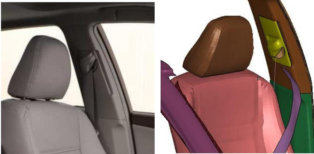
Figure 4.17 - Comparison between the D-ring in the real car and in the FE model
