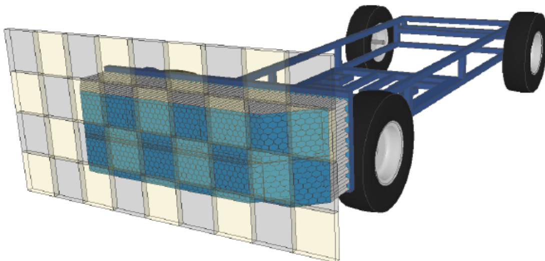
Figure 3.2 - AE-MDB FE model
