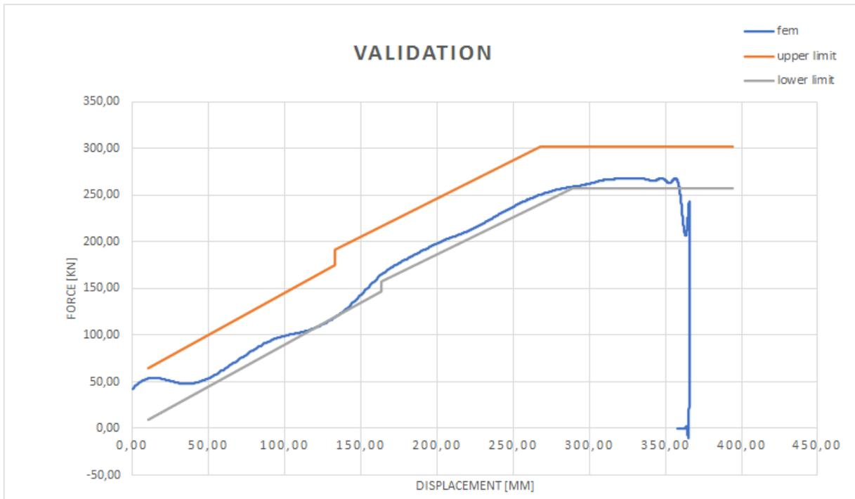
Figure 3.3 - Validation AE-MDB FE model
