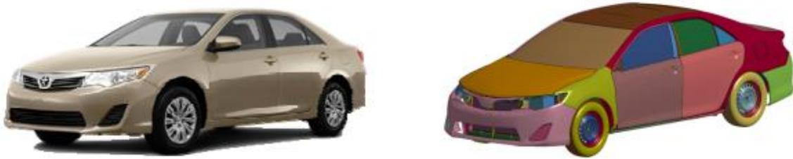
*Figure 3.4 - Comparison between the real Toyota Camry and the FE model*
