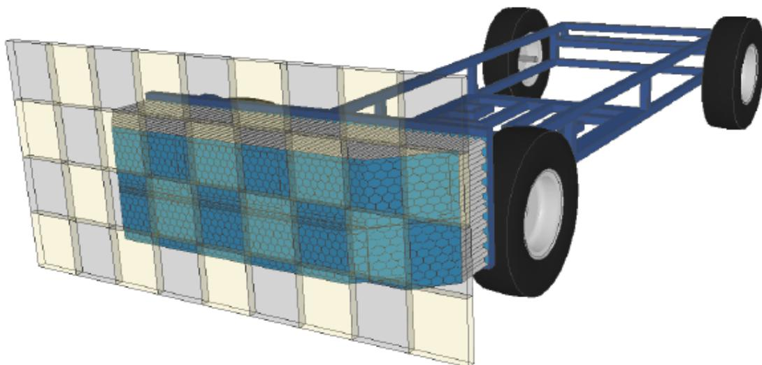
Figure 3.2 - AE-MDB FE model
