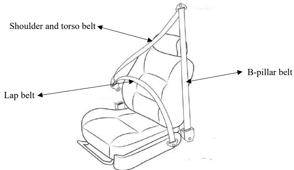
Figure 4.13 – three-point-seatbelt components
