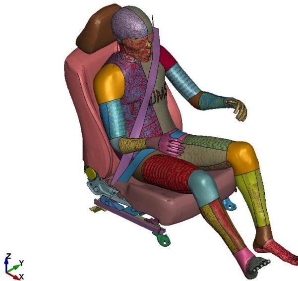
Figure 4.18 - THUMS positioned with the seatbelt model
