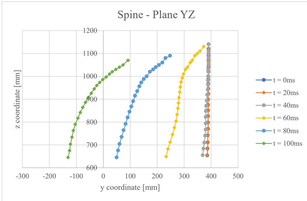
Figure 5.36 - Spine deformation on plane YZ at 0ms, 20ms, 40ms, 60ms, 80ms and 100ms
