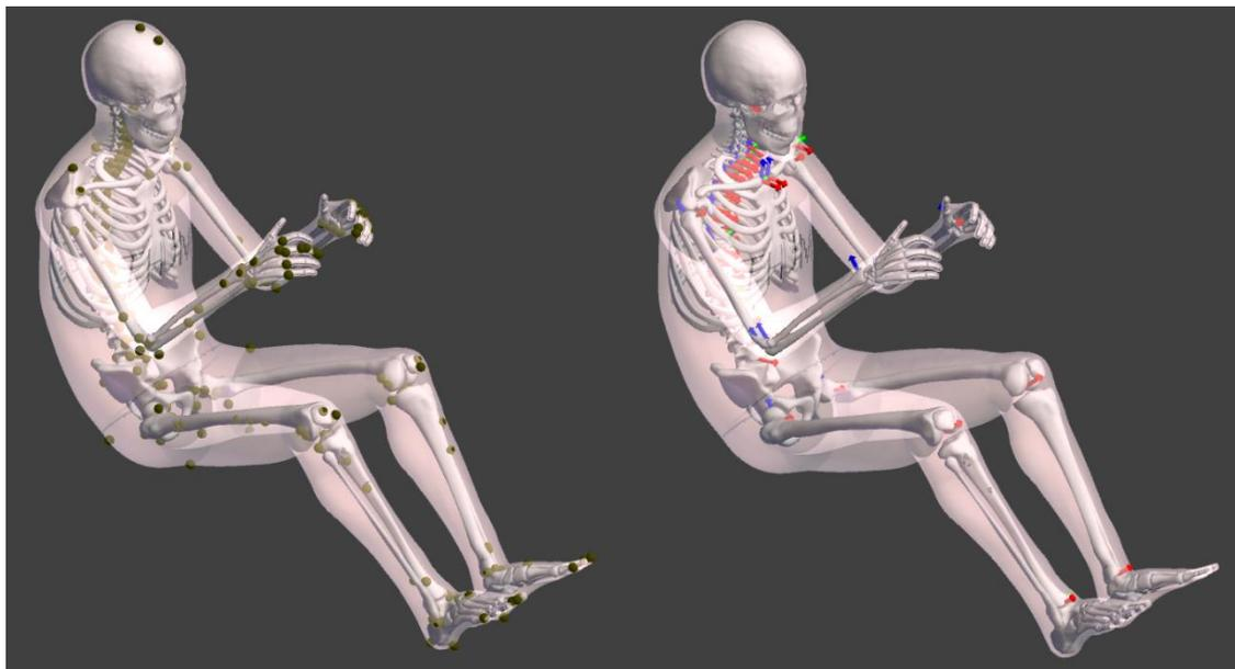
Figure 4.10 – Landmark and joint visualization in PIPER
