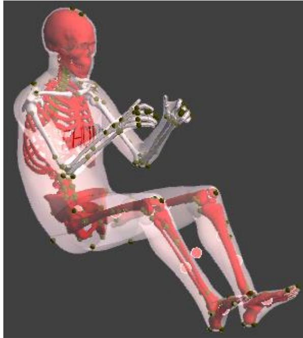
Figure 4.11 - Fixed bones example for upper limb positioning
