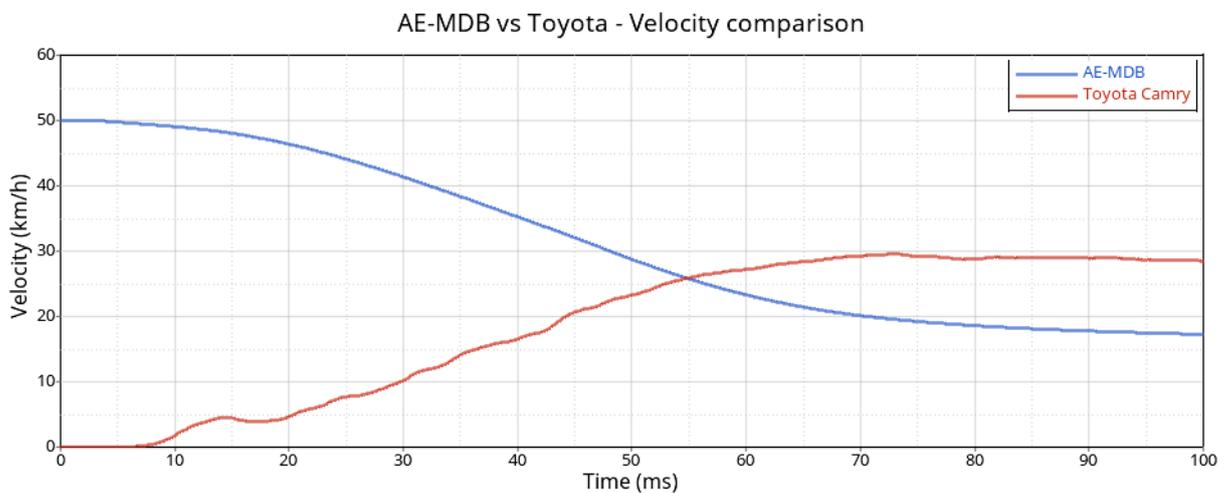
Figure 5.9 - AE-MDB vs Toyota - Velocity comparison
