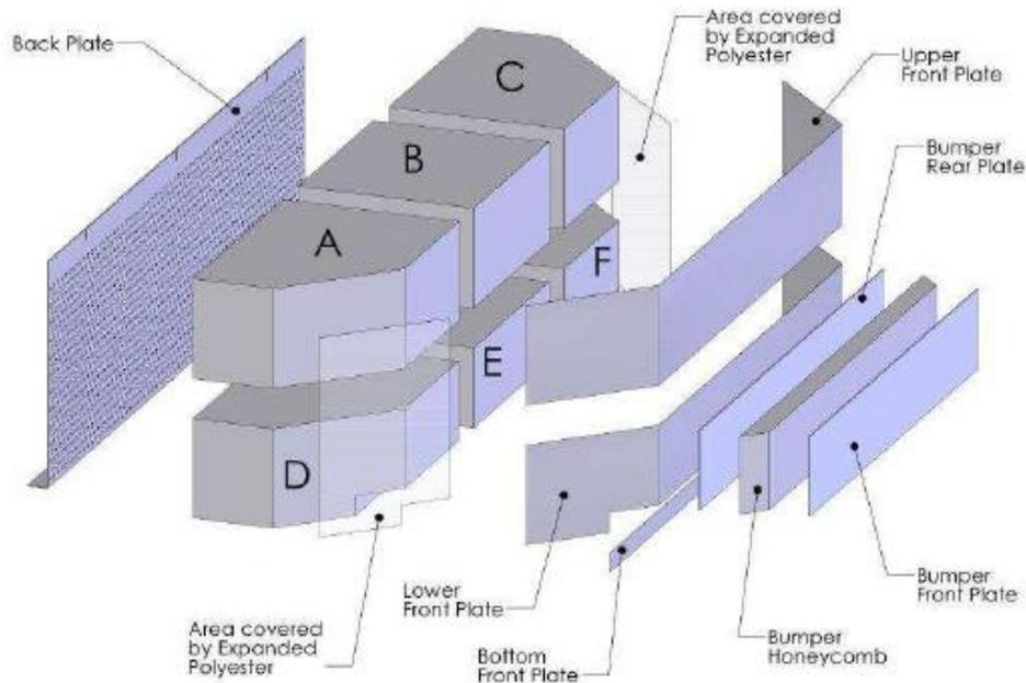
Figure 3.1 - AE-MDB barrier details
