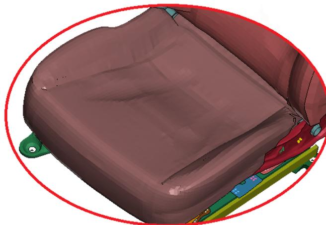
Figure 4.7 - Detail of the deformed seat cushion
