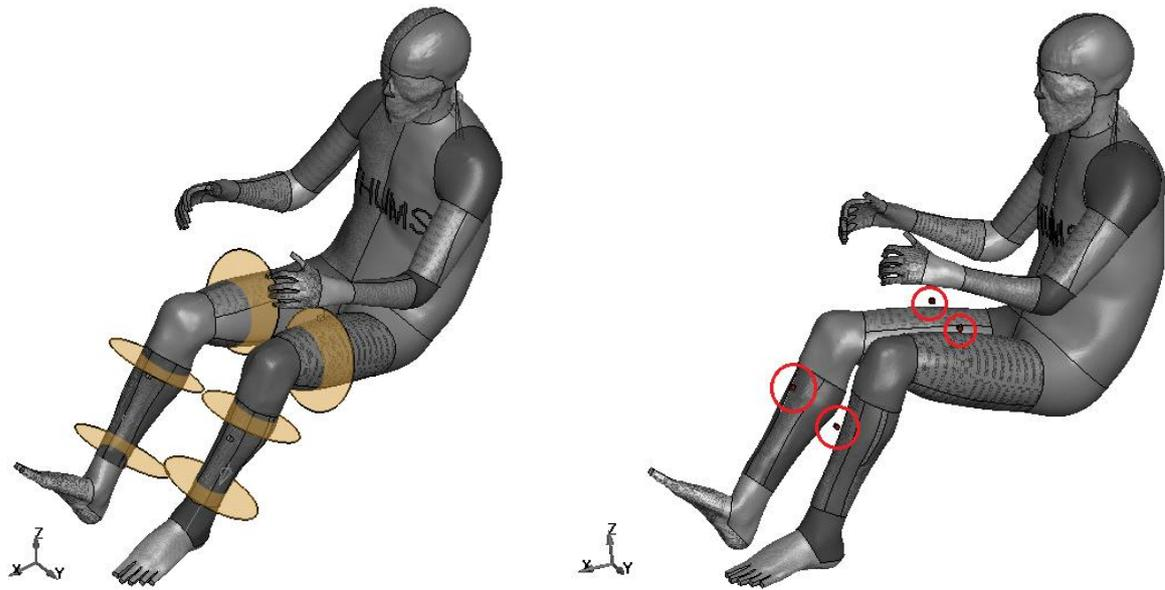
Figure 4.25 - Lower limbs sensors: cross\_section\_planes (left), accelerometer (right)
