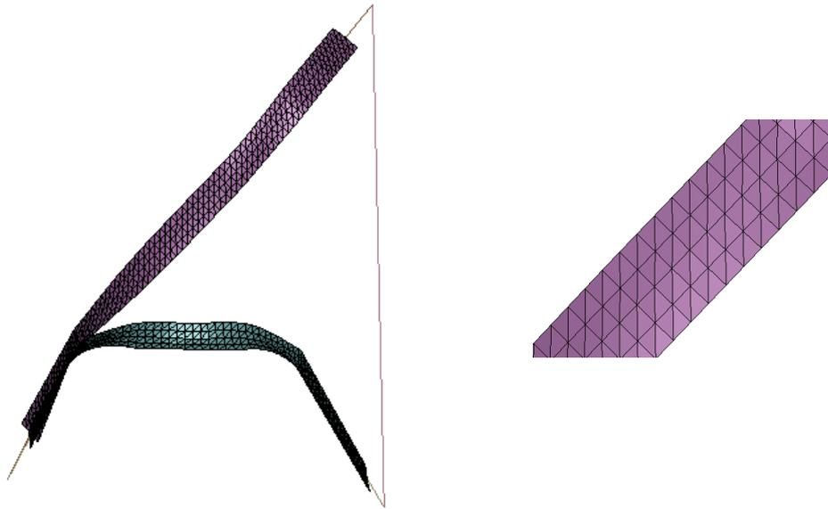
Figure 4.15 - Seatbelt model and detail of the seatbelt mesh
