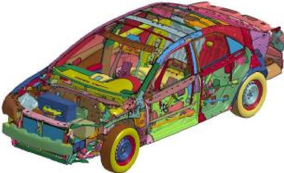
*Figure 3.5 - Detail FE model*
