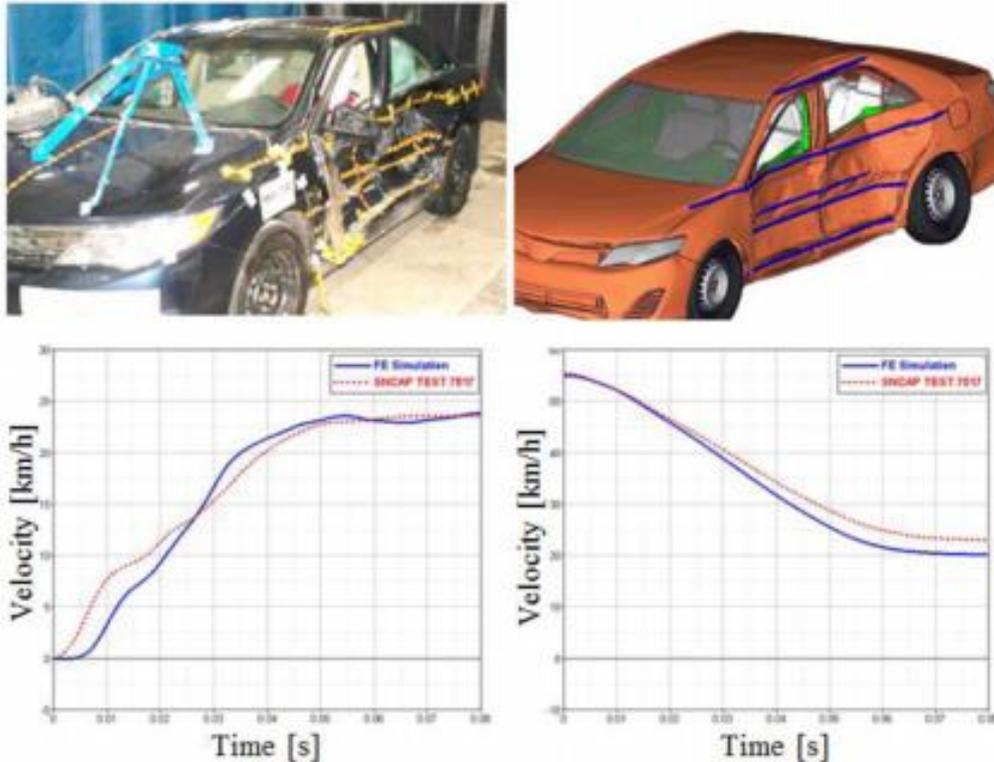
Figure 3.6 - Validation of the FE model in a SINCAP test
