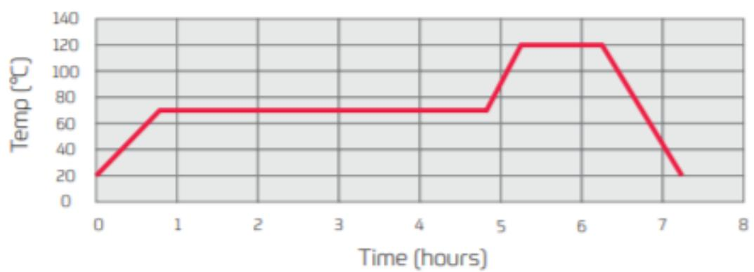
Figure 4.13: Curing cycle of XC110 Twill Prepreg Carbon fiber
