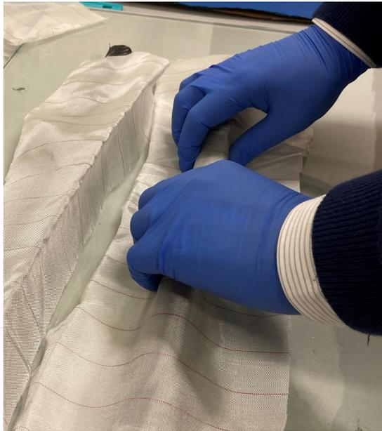
**Figure 4.9:** Peel ply adjusting
