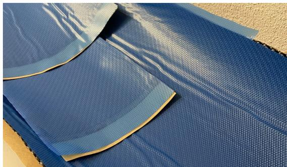
**Figure 4.1:** Sheets of Prepregs XC110 Twill Prepreg Carbon fiber
