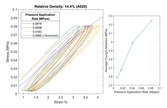
**Figure 3.10:** a) The hysteresis cycle changes shape at different force application rates. Static test on specimen A020 is added for comparison. b) The stiffness calculated from the average slope of the cycles.
