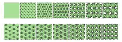
**Figure 3.1:** Two approaches of controlling the density: a) Fixing the thickness and varying the cell size; b) Fixing the cell size and varying the thickness.
