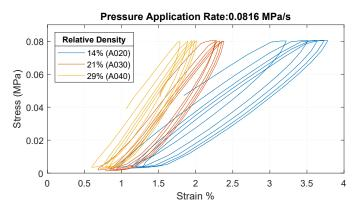
Figure 3.11: High-strain cyclic behaviour at different relative densities.
