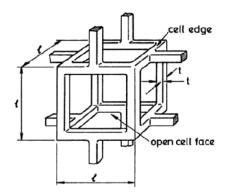
Figure 2.6: The model of foam invented by Gibson [1] to extract the theoretical equations for the stiffness and strength of foams.
