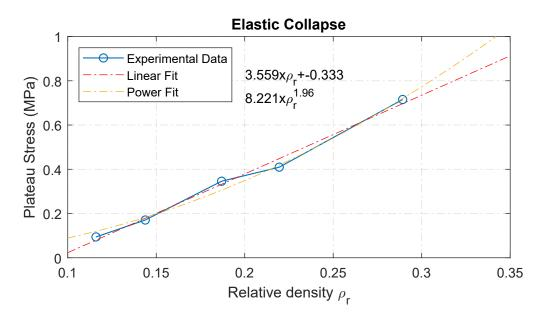
Figure 3.8: The lattice shows a constant stress over a major strain interval and depends on the relative density.
