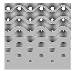
Figure 2.4: Grading thickness of a gyroid lattice in the z direction. $t^* = k \cdot z + t_0$
