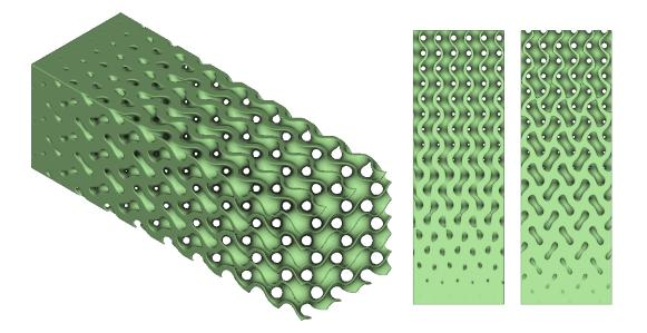
**Figure 3.17:** 'RAMP' specimen has a density that varies linearly between two opposite faces (direction z). As soon as the top layers enter the densification region, the lower layers enter the collapse region.
