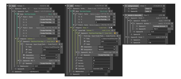
**Figure 4.1:** nTopology workflow. Surface integral is performed on the pressure field to calculate total weight and impression area. From this variables it's easy to figure out the required lattice thickness.
