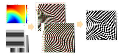
Figure 2.5: In this 2d example, the planar XY grating is varied with an orientation map to obtain a new spatially varied grid. The principal grating vector  $\vec{K}$  has unitary length and direction controlled by a 2d angular map (first graph). The grating vectors  $\vec{K_x}$  and  $\vec{K_y}$  are integrated separately and then recombined in the final grating.
