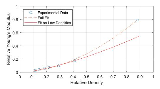
Figure 3.7: Two different Gibson Fit, one on full data and one restricted to low densities.
