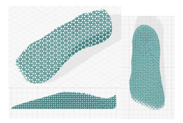
Figure 4.3: This image shows an insole engineered from practical example illustrated at step 4. The lattice density was designed to be 0.098. In our example, the dangerous peak of pressure was situated on the hill of the patient, so the insole was reduced in size with a cut in the middle to target specifically that area.
