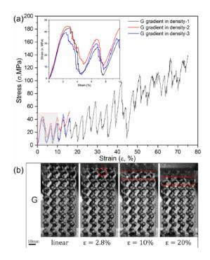
Figure 3.19: From Liu et Al. [15] shows a specimen with linear density ramp manufactured from Titanium. The material is quite brittle and fails layer by layer, bu it is possible to see how the stress-strain curve follows a linear trend.
