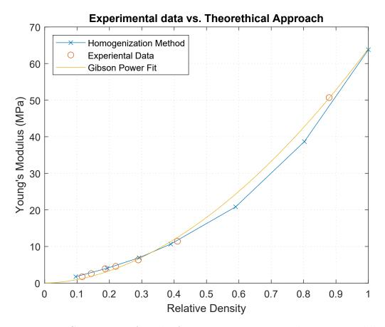
**Figure 3.14:** Comparison of results form Homogenization and experimental data (orange dots). Even without taking into account the edge effects, there is a great match between theory and specimens.
