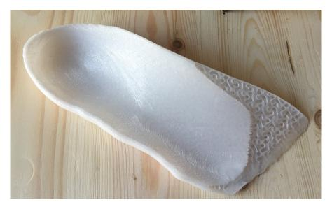
Figure 4.5: The prototype printed with a 0.3 mm nozzle in around 8 hours. A thin skin was added during design to increase comfort to the user, but trough the slice it's possible to see the lattice geometry.
