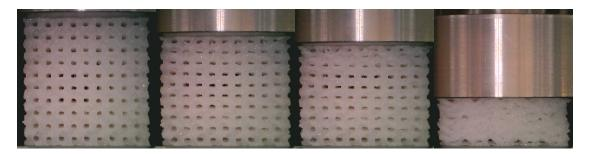
**Figure 3.3:** Crushing behaviour of specimen A020: a) initial contact; b) linear elastic compression; c) asynchronous collapse of lattice layers; d) full collapse and densification.
