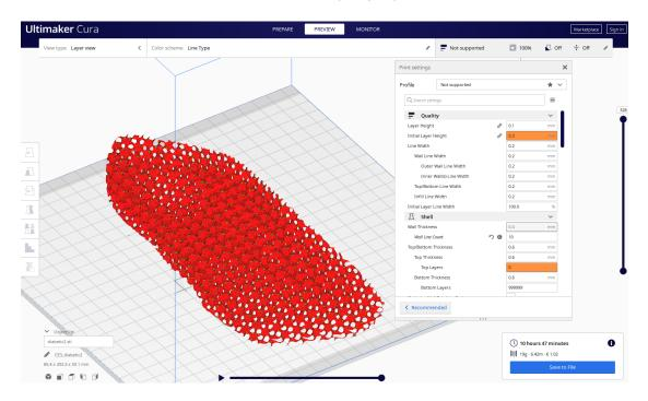
Figure 4.4: Cura 4.8 interface showing the insole for diabetic foot ready to be printed. On the right it's possible to control various parameters and after the slicing is done the software shows the estimated time and filament length.
