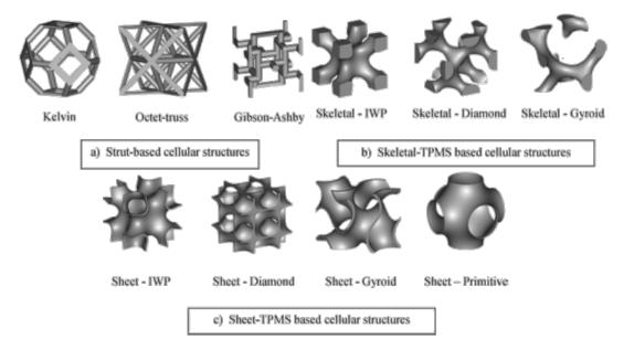
**Figure 2.1:** Different topologies of unit cells, some based on trusses and others on Triply Periodic Minimal Surfaces. Image from [8]
