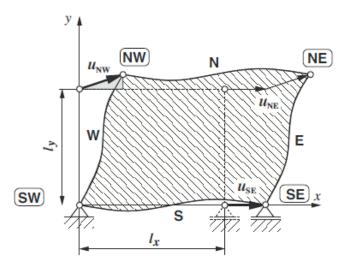
**Figure 2.7:** Idealized representation of a 2d unit cell in undeformed and deformed configuration. Boundary conditions are applied between opposite edges. Image from [11]
