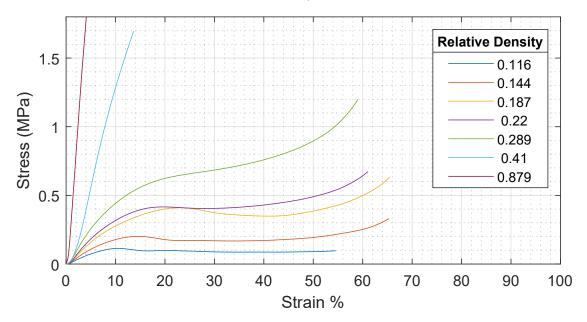
Figure 3.4: Stress/Strain plot for cubic samples of dimension 5x5x5 unit cells.
