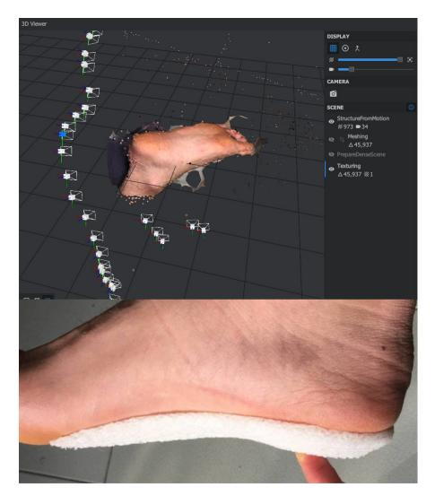
**Figure 4.6:** The photogrammetry used to extract the foot shape is meshroom and a video made with the camera of a cheap phone. The final insole shows a tight fit with the foot.
