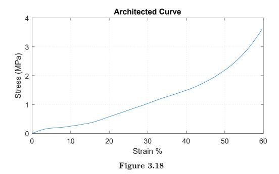
occurs. During testing, the first layers were soft and started to crush at around 5% total strain, but since their thickness was really limited to few millimeters, the
