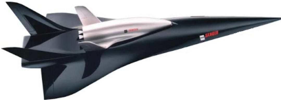
Figure 3.37. Saenger vehicle configuration [14]
