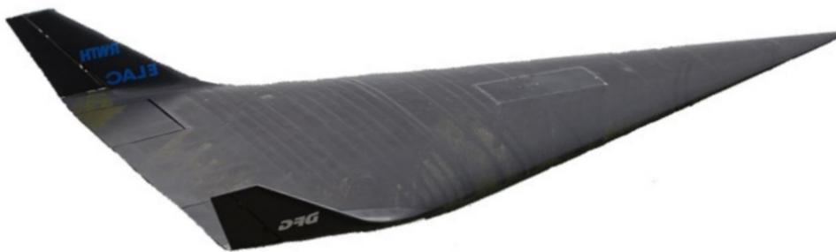
Figure 3.36. ELAC vehicle configuration [25]
