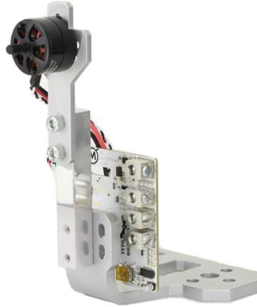
Figure A.1: RCbenchmark Series 1520 Thrust Stand [45]
