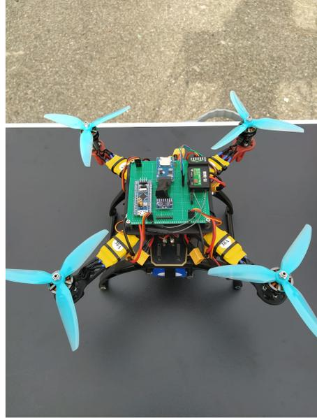
Figure 7.4: Picture of the quadcopter and Flight Controller before flight tests
