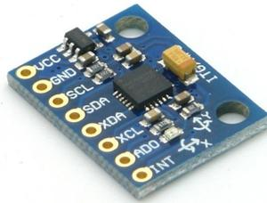
Figure 2.1: MPU-6050 gyroscope/accelerometer MEMS
