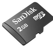
Figure 6.8: 2 GB micro SD card used to log flight data
