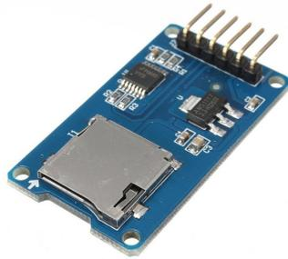
Figure 6.7: SD card adapter used to interface STM-32 board
