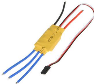
Figure 3.7: Electronic Speed Controller
