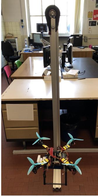
Figure A.4: Pendulum used to measure  $I_x$  and  $I_y$
