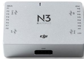
Figure 1.22: N3 flight controller
