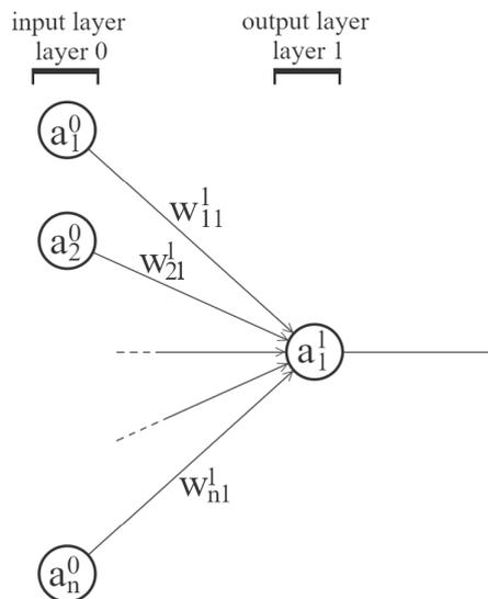
**Figure 2.3:** A perceptron immersed in a network - it is shown its connection with the input layer. The input layer has  $n$  several units which are activated from an external source:  $a_1^0, a_2^0, \dots, a_n^0$ . The input propagates toward the perceptron using the edges, where the Equation 2.1 computes the output  $a_i^1$ . Noticed that while the weight values are proper of each edge, the bias term is contained in the perceptron and not visible, as well as the activation function.
