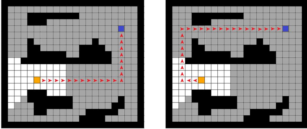
**Figure 4.11:** Traditional A\* and Explorative A\* in comparison, same situation. The UAV is located in the orange square; the goal cell to reach is represented in blue. The left figure shows the path with Traditional A\*, which is the shortest path; the right figure shows the path with Explorative A\*, which accounts for both the length of the path and the exploration of new cells (in grey).
