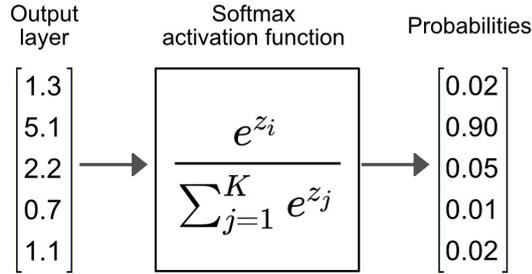
**Figure 3.6:** Softmax application example - each component of the input vector is transformed into an exponential probability distribution using Equation 3.1.
