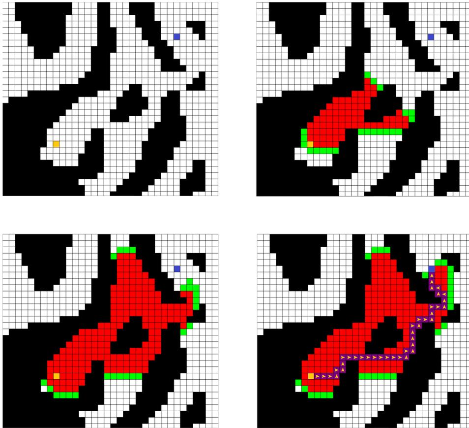
**Figure 4.10:** Traditional A\* finds the path - the start cell is represented in orange; the goal cell is represented in blue; red cells are the nodes visited by the algorithm; green cells are the cells that the algorithm can expand; the final purple cells represent the minimum and optimal path to reach the goal from the start.
