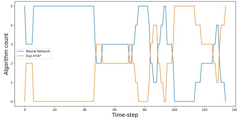
**Figure 5.5:** Case study I, 5 agents - On the x axis, the time-steps. For each time-step, the graphic shows the number of agents that use the neural network approach, in orange, and the explicit path-finders, in blue.
