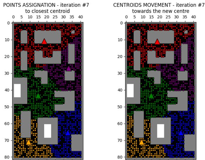
**Figure 4.7:** Seventh and last iteration of the K-means. In the left figure, each point is assigned to the closest centroid. In the right figure, each centroid is moved toward the averaged points' position.
