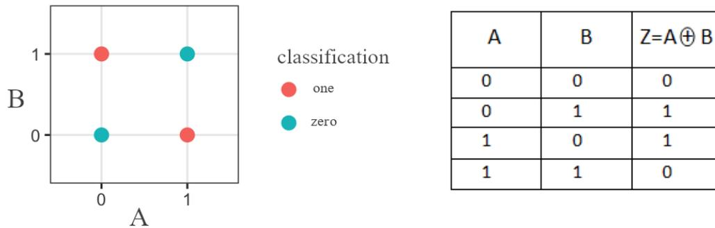
**Figure 2.4:** On the right, the XOR Boolean truth table. On the right, the function represented on the Cartesian plane.
