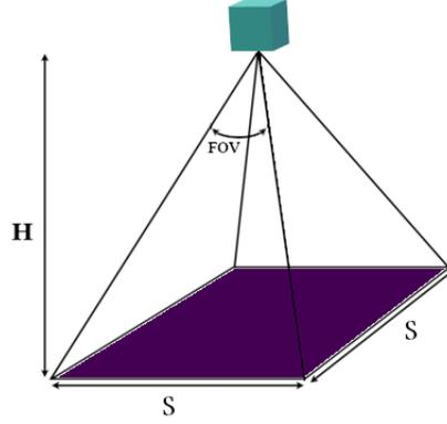
**Figure 4.1:** UAV's camera cone of visibility: in purple, according to the Field Of View, the camera ground footprint; in teal, a single UAV.
