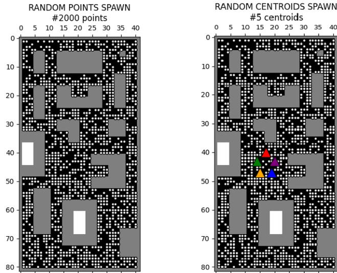
**Figure 4.4:** In the left figure, 2000 white points are spread over the unexplored target area. In the right figure, five centroids, represented as triangles, are positioned in each UAV's starting position.
