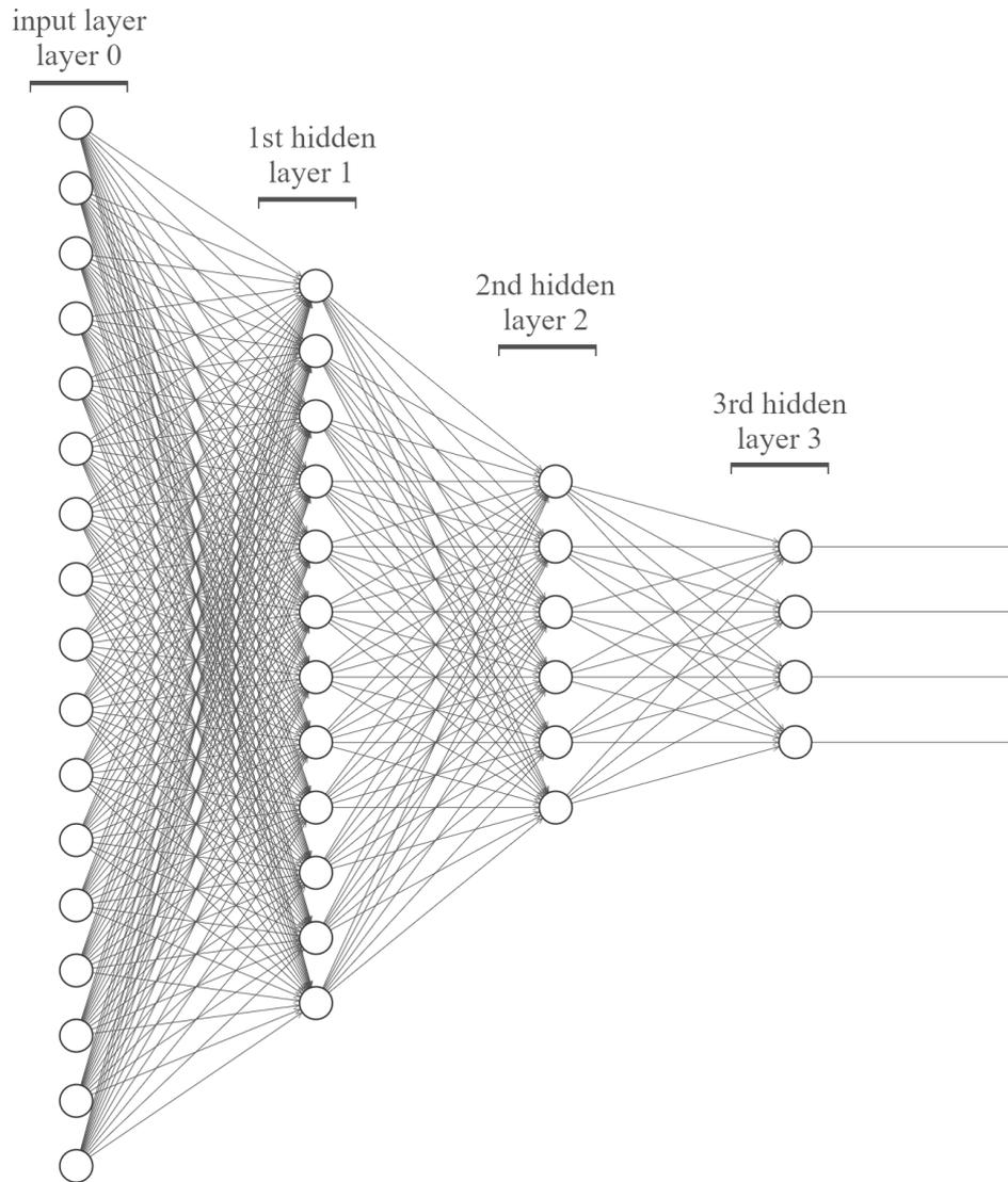
**Figure 2.5:** A Standard Fully Connected Artificial Neural Network with four output. This network has an architecture with 3 computational layers, two of which are hidden and the last one is the output. The input vector contains 17 feature information, each of which constitutes the activation of a neuron.
