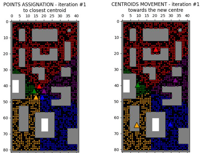
**Figure 4.5:** In the left figure, each point is assigned to the closest centroid. In the right figure, each centroid is moved toward the averaged points' position. This process represents one complete iteration of the K-means algorithm.
