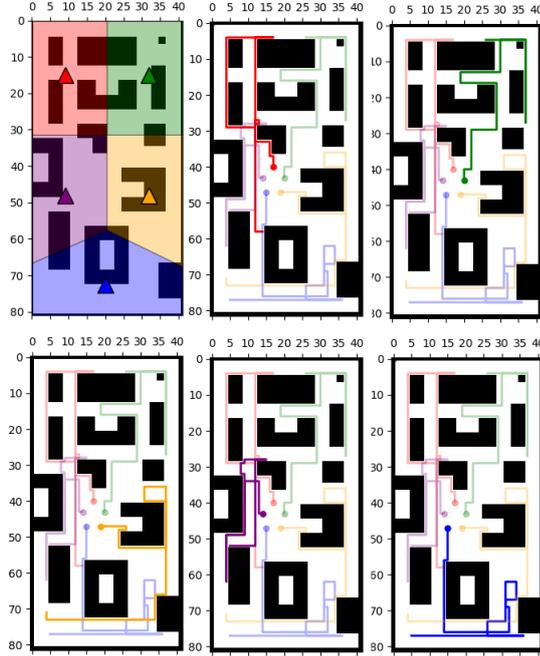
**Figure 5.4:** Case study I - trajectories in the simulation with 5 agents. The upper left image shows the area division, according to the K-means algorithm . In the other images, the overall UAVs' track, where each singular UAV trajectory is highlighted.
