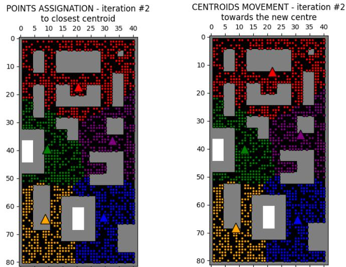
**Figure 4.6:** Second iteration of the K-means. In the left figure, each point is re-assigned to the closest centroid. In the right figure, each centroid is moved toward the averaged points' position
