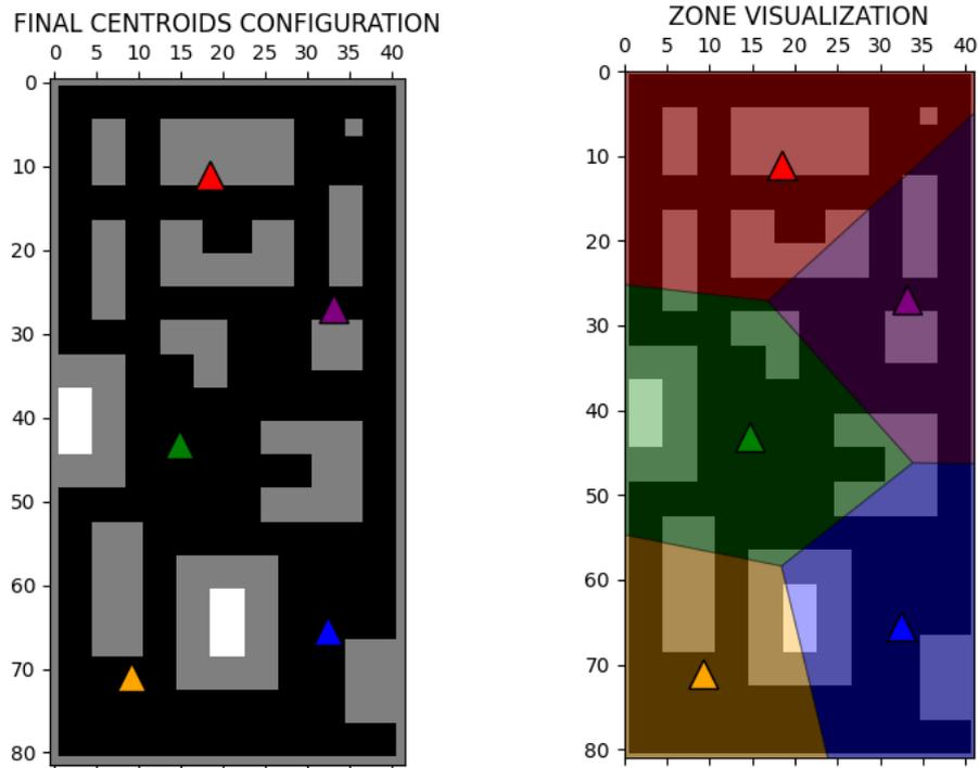
**Figure 4.8:** In the left figure, the centroids' final position cleared from the points. In the right figure, the correspondent Voronoi tessellation.
