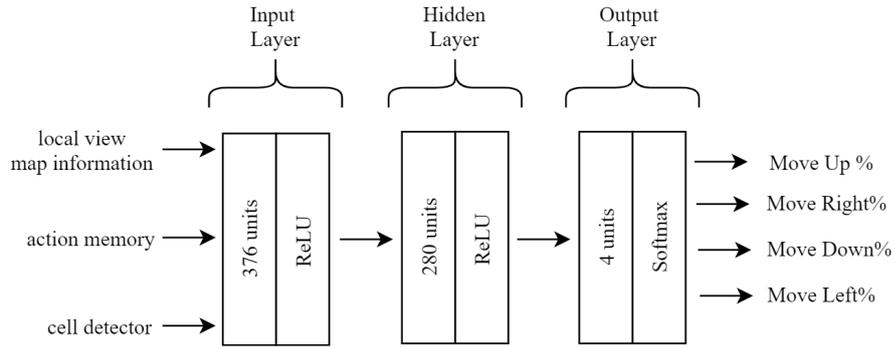
**Figure 3.4:** Neural Network’s architecture. From left to right: the feature vector (state) is fed in the input layer. Then it gets propagated forward in the hidden layer and finally reaches the output layer, where the softmax function normalizes the probability distributions. For each of the four actions, it is possible to read the percentage of prediction of the network and use it to in the algorithm to move the correspondent agent.
