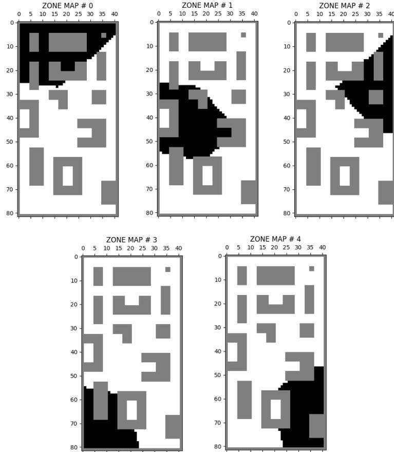
**Figure 4.9:** Zone visualization - every single zone is highlighted, showing in black the correspondent target area, and in white the non-target cells. In this example, five UAVs will explore the map, each one assigned to a particular zone.
