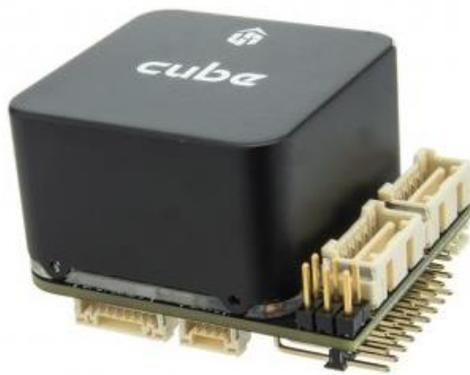
*Figura 6-11 – Flight Controller Cube black+ su mini Carrier Board*
