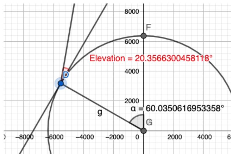
**Figure 6 - GEO coverage at the equator with 20 degrees of elevation**
