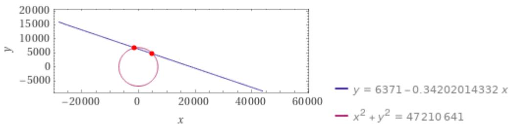
**Figure 12 - Radius of the visibility cone at the satellite entry points**
