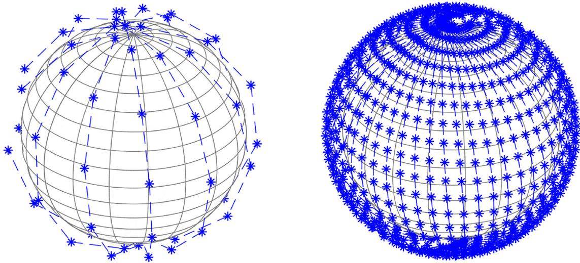
**Figure 23 - Routing in Iridium vs Mega-constellations [26]**
