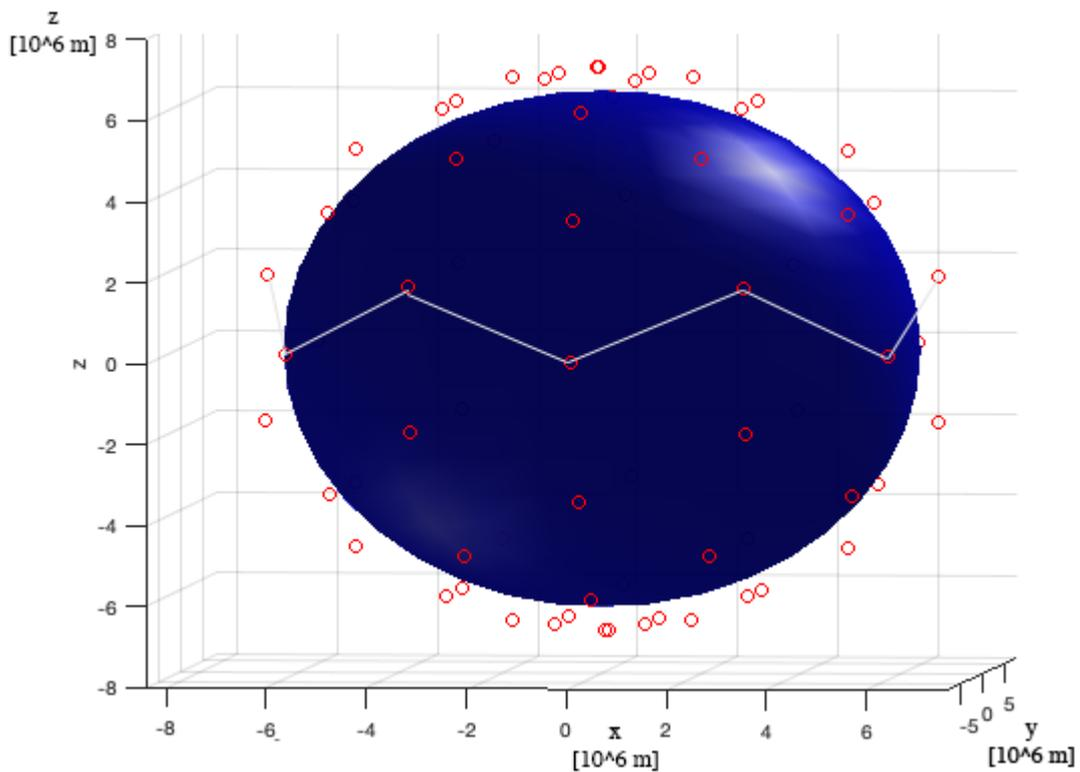
**Figure 22 - Signal path in inter-satellite links**
