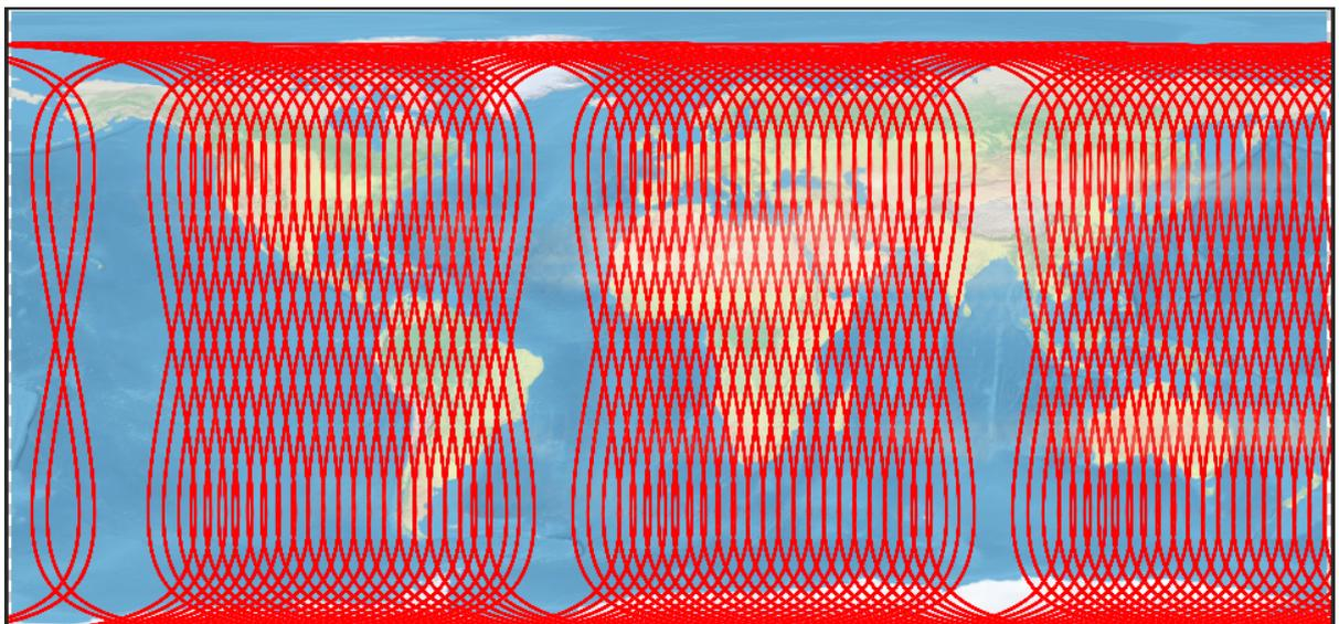
**Figure 5 - Polar orbit RGT Simulation [11]**
