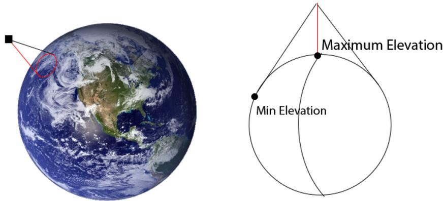
**Figure 2 - Minimum and maximum elevation angles**
