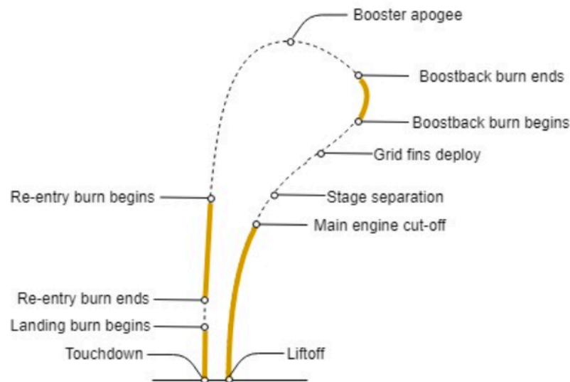
Figure 18 Return-to-launch-site flight profile – [31]
