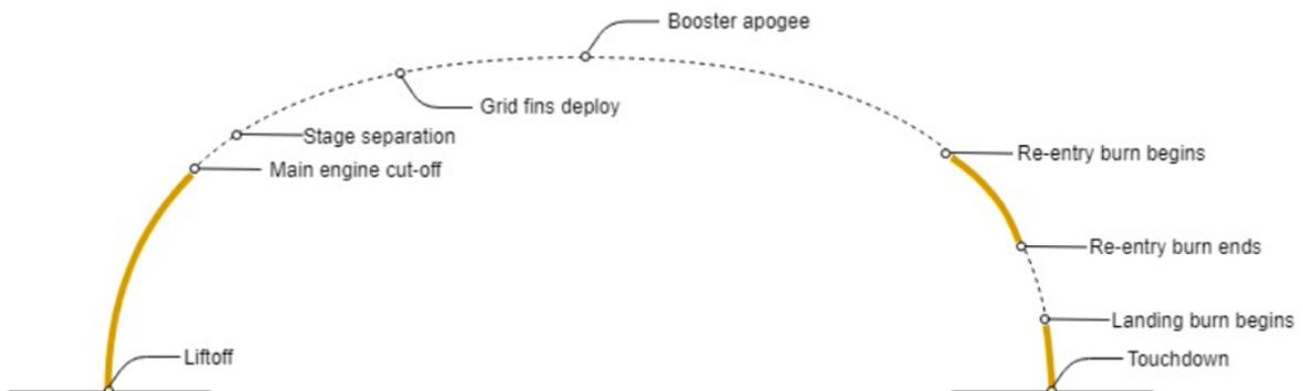
Figure 17 Downgrade landing flight profile [31]
