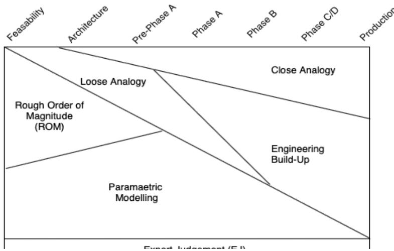
Figure 10 Qualitative application of CEMs according to project phase [36]
