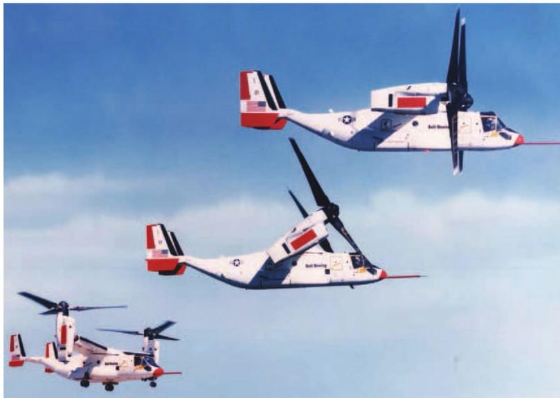
Figure 1.1: V-22 Osprey in Helicopter, Conversion and Airplane Mode, from Left to Right, Ref. [1]
