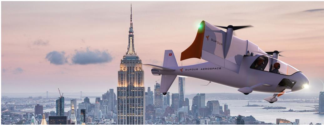
**Figure 1.14:** Rendering of the Electric Tilt-Wing Aircraft Being Currently Developed by Dufour Aerospace, Ref. [12]
