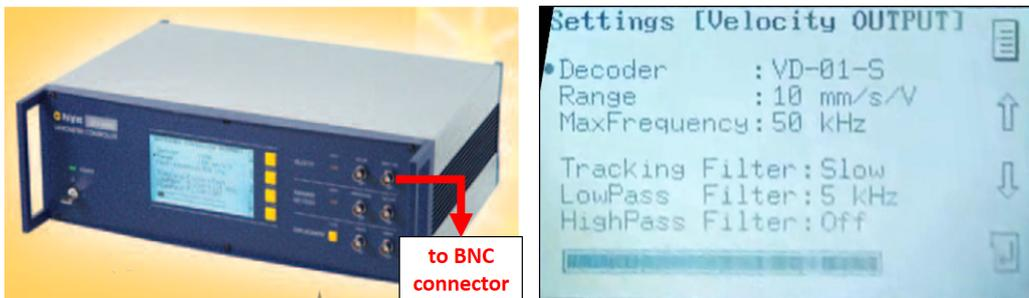
Figura 2.10: Polytec OFV-5000 Vibrometer controller
