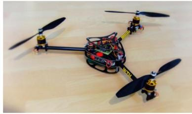
**Figure 2.11:** Example of Tricopter "Y" shaped
