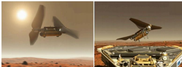
**Figure 1.12:** View of Entomompter designed by Colozza [1] for Mars exploration
