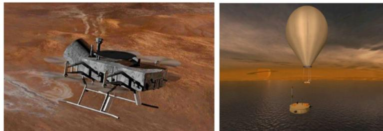
**Figure 1.5:** Titan's drone concepts: Dragonfly and Montgolfiere balloon flagship [1]
