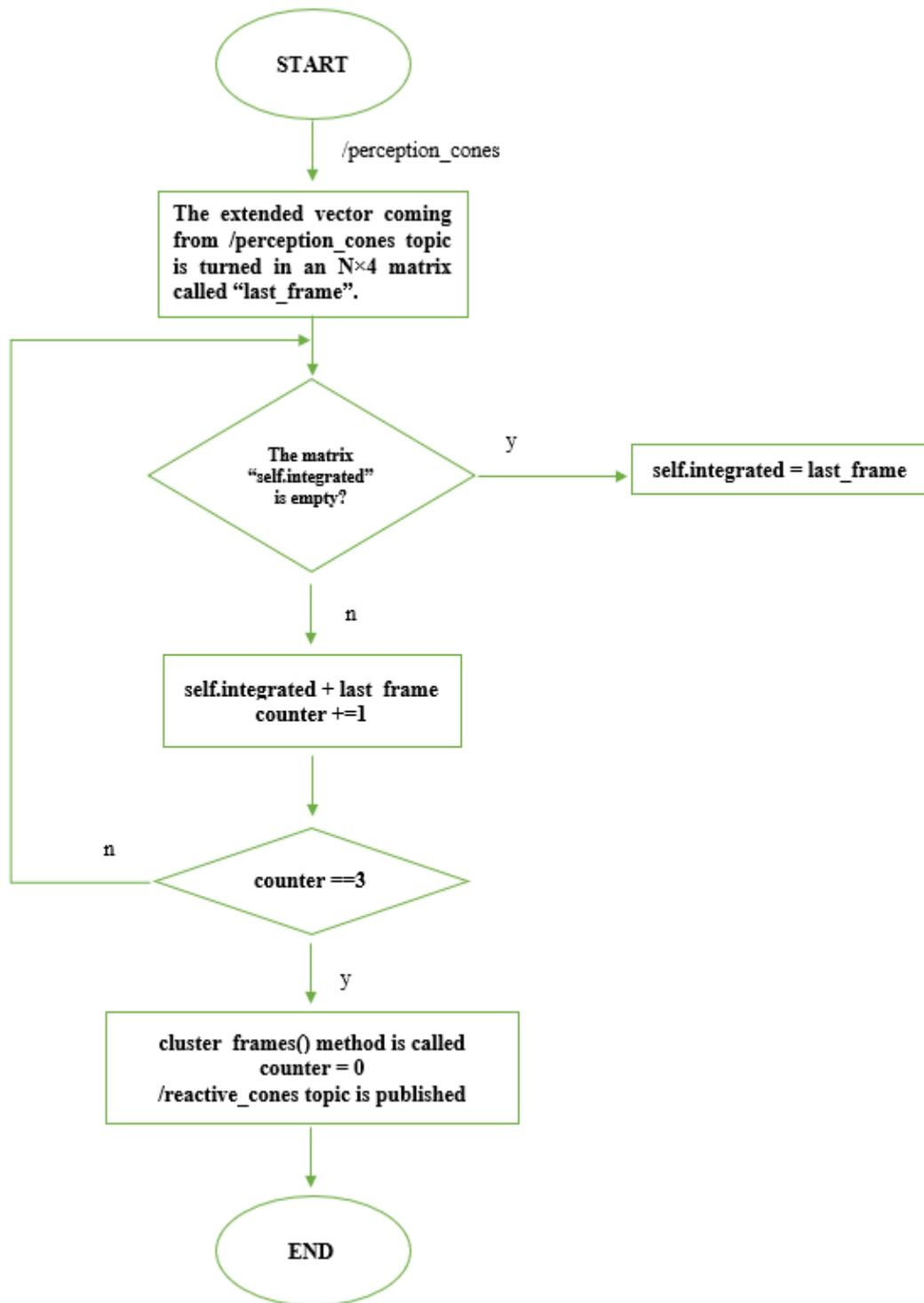
Figure 30: `callback_perception()` method flowchart, N.B. `self.integrated + last_frame` means that if the first is a  $2 \times 4$  matrix and the second one is  $1 \times 4$  the results will be the matrix  $3 \times 4$  with the element of the previous ones.
