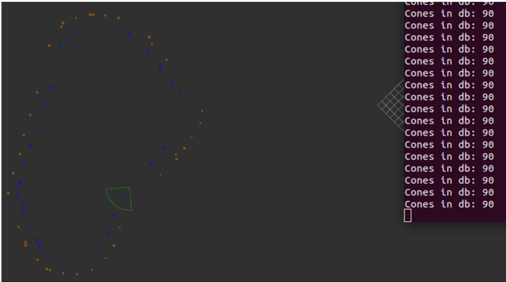
Figure 60: small-track simulation, with car speed of 2.5m/s and the update frequency of 30Hz
