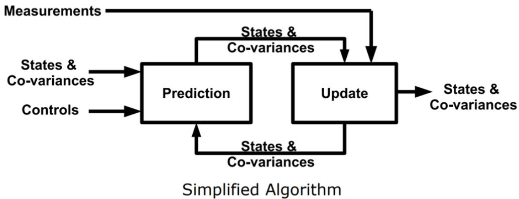
Figure 16: The Extended Kalman Filter simplified algorithm scheme [27]
