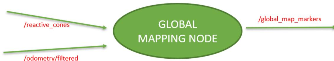
Figure 32: The global mapping node scheme
