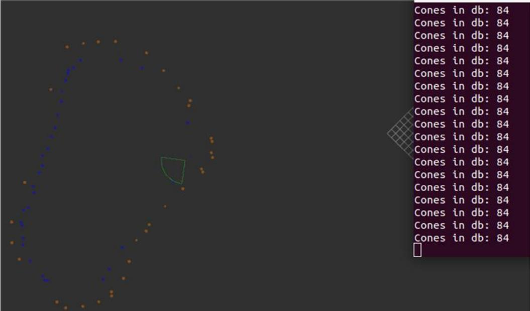
Figure 62: small-track simulation, with car speed of 7m/s and the update frequency of 10Hz
