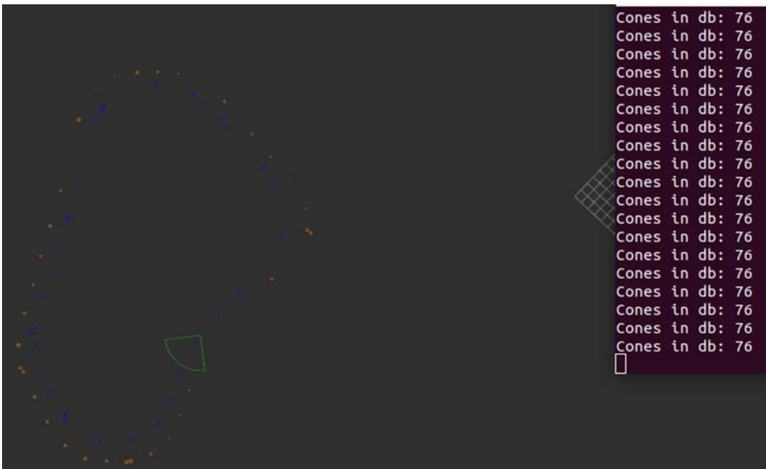
Figure 55: small-track simulation, with car speed of 1.5m/s and the update frequency of 20Hz
