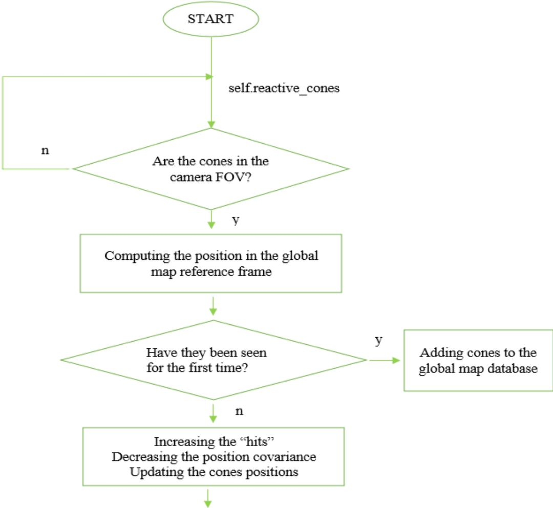
Figure 33: the global mapping algorithm flowchart (part\_1)
