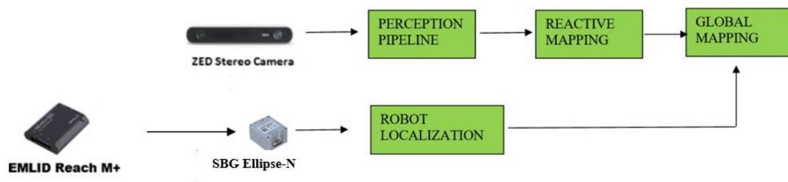
Figure 14: Overall scheme of the PoliTo SC19 electric car SLAM process
