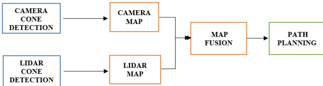
Figure 70: Camera and LIDAR map fusion
