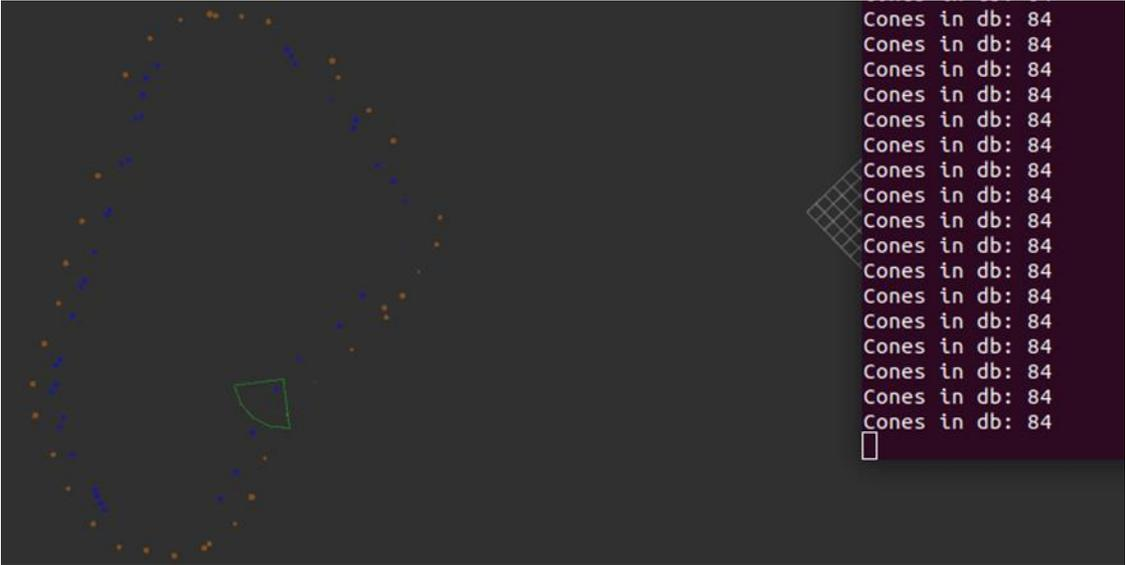
Figure 59: small-track simulation, with car speed of 2.5m/s and the update frequency of 20Hz
