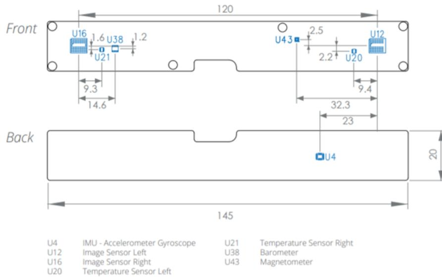
Figure 10: sensors placement on the ZED 2 stereo camera [37]
