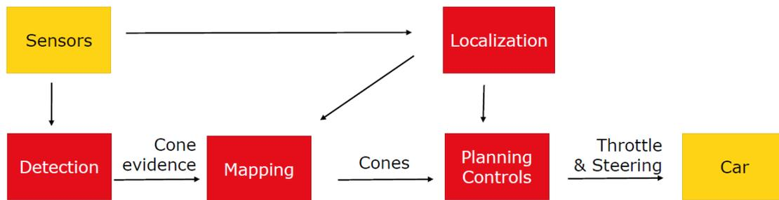
Figure 37: The EUFS simulator architecture [27]
