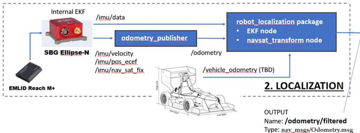
Figure 17: Localization software architecture
