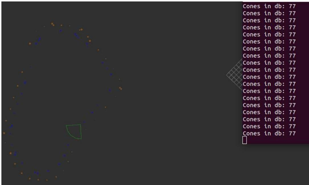
Figure 53: small-track simulation, with car speed of 1.5m/s and the update frequency of 5Hz
