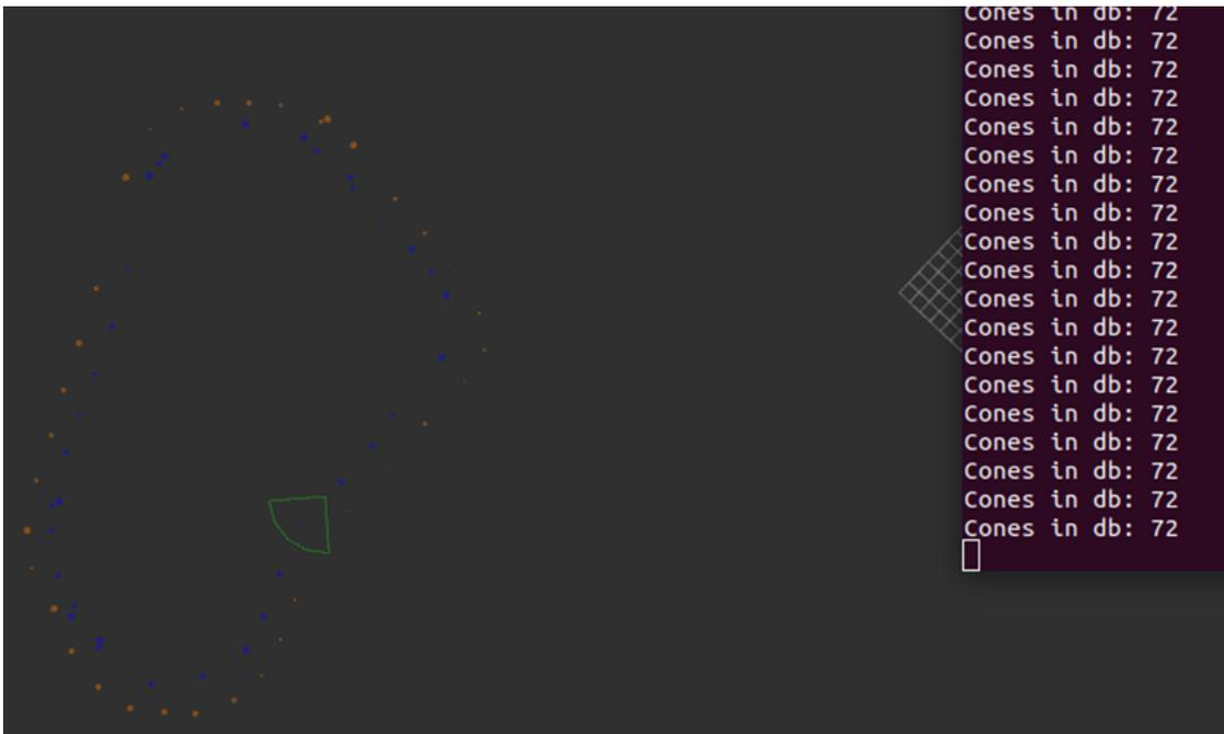
Figure 54: small-track simulation, with car speed of 1.5m/s and the update frequency of 10Hz
