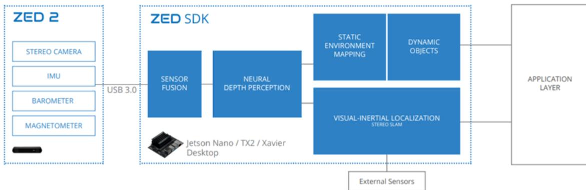
Figure 11: Functional SDK Diagram [37]
