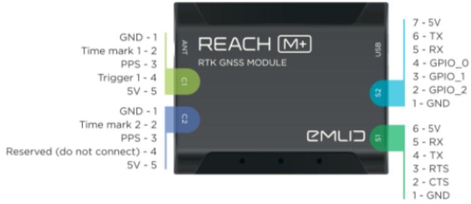
Figure 13: connectors pinout scheme [26]
