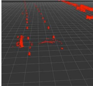
*Figure 6: example of pointcloud obtained by a 40-layer single LIDAR [27]*
