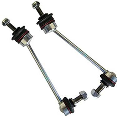
Figure 2.19: Anti Roll Drop Link
